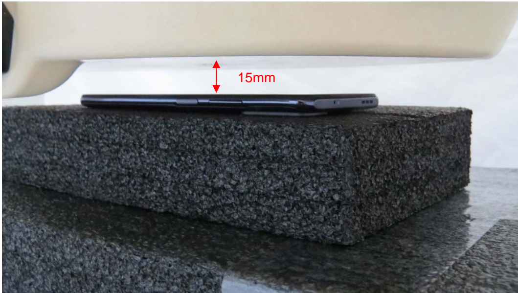
Picture 7: Front Side, the distance from handset to the bottom of the Phantom is 15mm
