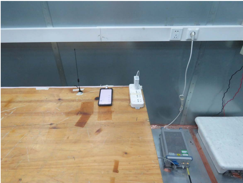
Picture 2 Conducted Emission Test Setup
