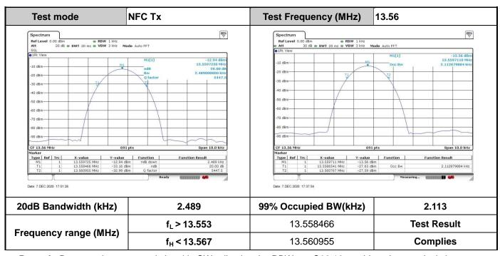
**Remark:** Because the measured signal is CW adjusting the RBW per C63.10 would not be practical since measured bandwidth will always follow the RBW and the result will be approximately twice the RBW.
