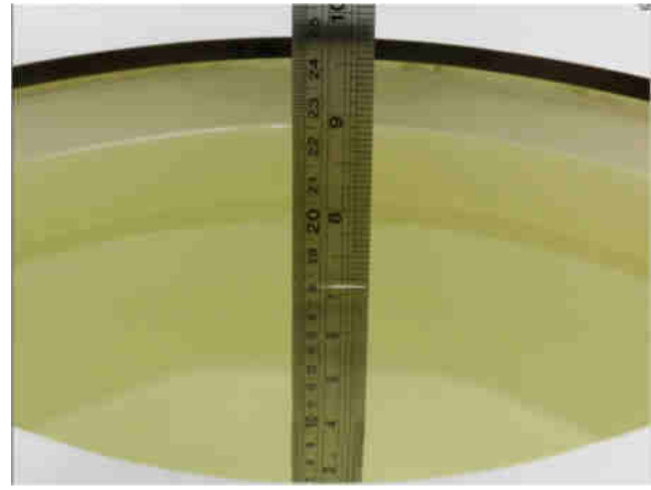
Fig 11.2 Photo of Liquid Height for Body SAR
