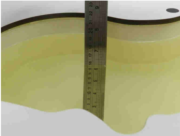
Fig 11.1 Photo of Liquid Height for Head SAR
