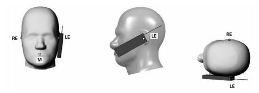
Fig 9.2.3 cheek or touch position. The reference points for the right ear (RE), left ear (LE), and mouth (M), which establish the Reference Plane for handset positioning, are indicated.
