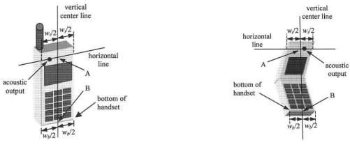
Fig 9.2.1 Handset vertical and horizontal reference lines—"fixed case
