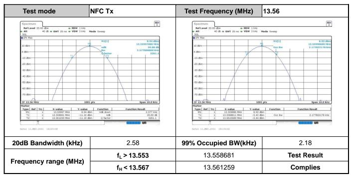
**Remark:** Because the measured signal is CW adjusting the RBW per C63.10 would not be practical since measured bandwidth will always follow the RBW and the result will be approximately twice the RBW.
