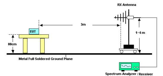
For radiated test from 1GHz to 18GHz
