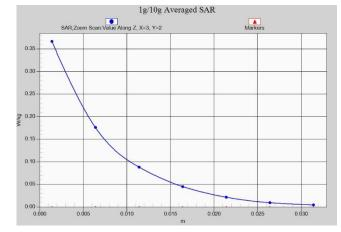
Fig. 1-45 Z-Scan at power reference point (LTE Band38)
