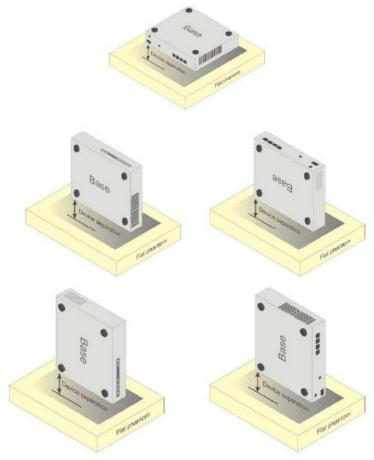
Picture D.5 Test positions for desktop devices
