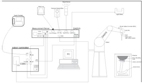
Picture C.1SAR Lab Test Measurement Set-up
