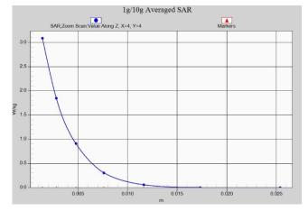
Fig. 1-48 Z-Scan at power reference point (5 GHz)
