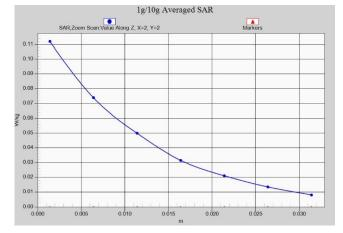
Fig. 1-21 Z-Scan at power reference point (PCS1900)
