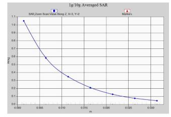
Fig. 1-36 Z-Scan at power reference point (LTE Band4)
