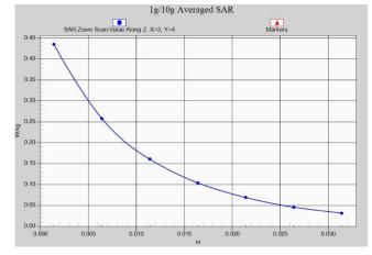
Fig. 1-39 Z-Scan at power reference point (LTE Band5)
