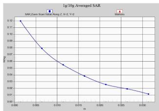
Fig. 1-35 Z-Scan at power reference point (LTE Band4)
