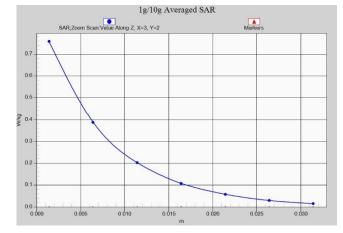
Fig. 1-42 Z-Scan at power reference point (LTE Band 7)
