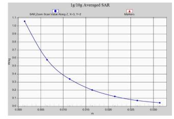
Fig. 1-33 Z-Scan at power reference point (LTE Band2)
