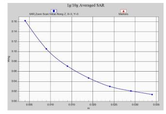
Fig. 1-27 Z-Scan at power reference point (WCDMA1700)
