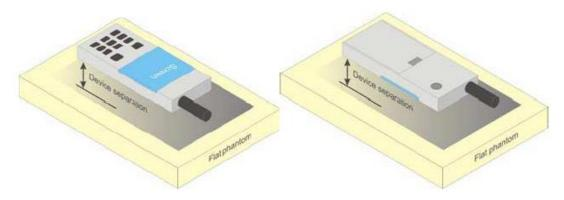
Picture D.4Test positions for body-worn devices
