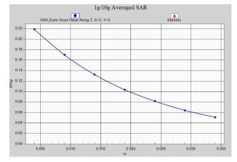
Fig. 1-30 Z-Scan at power reference point (WCDMA850)
