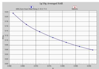
Fig. 1-38 Z-Scan at power reference point (LTE Band5)
