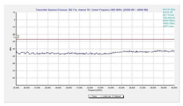
Fig. 82 Conducted Spurious Emission (802.11a, Ch161, 25 GHz-40 GHz)
