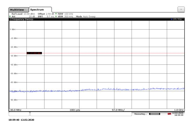
Fig. 65 Conducted Spurious Emission (802.11ax-HE40-RU242-right, Ch151, 30 MHz-1 GHz)
