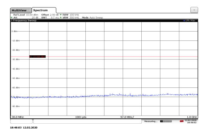
Fig. 133 Conducted Spurious Emission (802.11ax-HE40-RU242-right, Ch151, 30 MHz-1 GHz)
