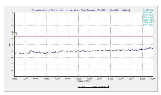
Fig. 73 Conducted Spurious Emission (802.11a, Ch149, 12 GHz-25 GHz)
