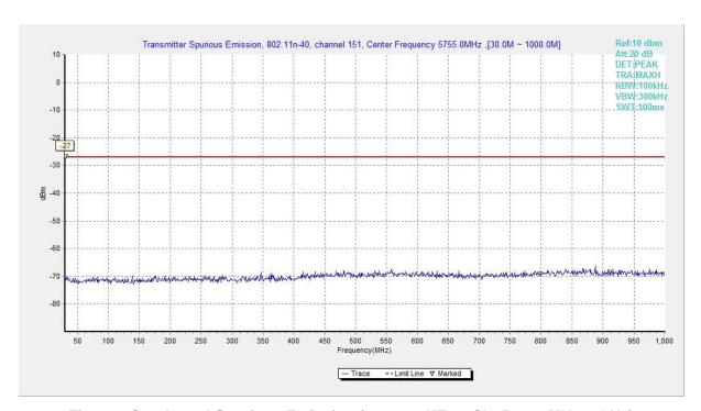
Fig. 107 Conducted Spurious Emission (802.11n-HT40, Ch151, 30 MHz-1 GHz)
