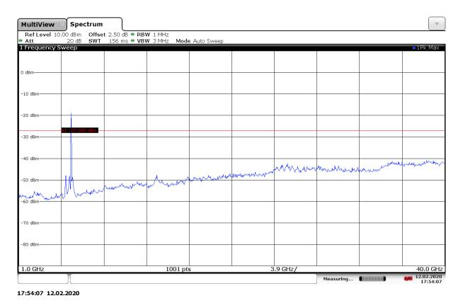
Fig. 130 Conducted Spurious Emission (802.11ax-HE20-RU106-right, Ch157, 1 GHz-40 GHz)
