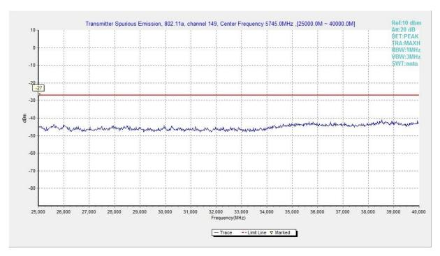
Fig. 74 Conducted Spurious Emission (802.11a, Ch149, 25 GHz-40 GHz)
