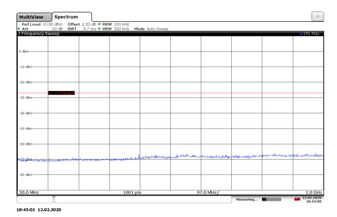
Fig. 135 Conducted Spurious Emission (802.11ax-HE40-RU242-right, Ch159, 30 MHz-1 GHz)
