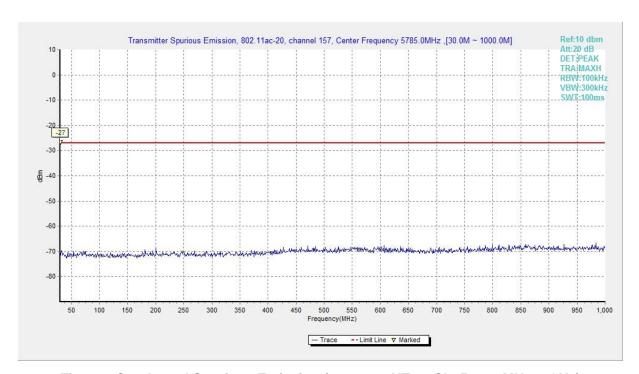
Fig. 99 Conducted Spurious Emission (802.11ac-HT20, Ch157, 30 MHz-1 GHz)
