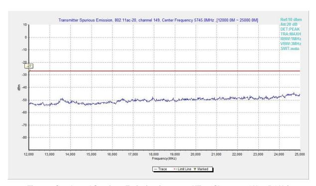
Fig. 97 Conducted Spurious Emission (802.11ac-HT20, Ch149, 12 GHz-25 GHz)
