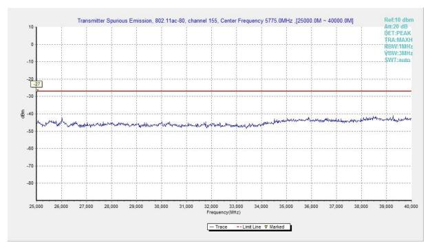
Fig. 126 Conducted Spurious Emission (802.11ac-HT80, Ch155, 25 GHz-40 GHz)
