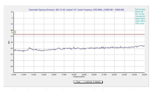
Fig. 89 Conducted Spurious Emission (802.11n-HT20, Ch157, 12 GHz-25 GHz)
