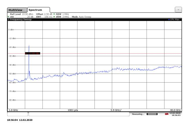
Fig. 66 Conducted Spurious Emission (802.11ax-HE40-RU242-right, Ch151, 1 GHz-40 GHz)
