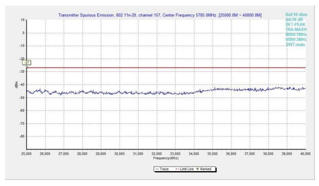
Fig. 90 Conducted Spurious Emission (802.11n-HT20, Ch157, 25 GHz-40 GHz)
