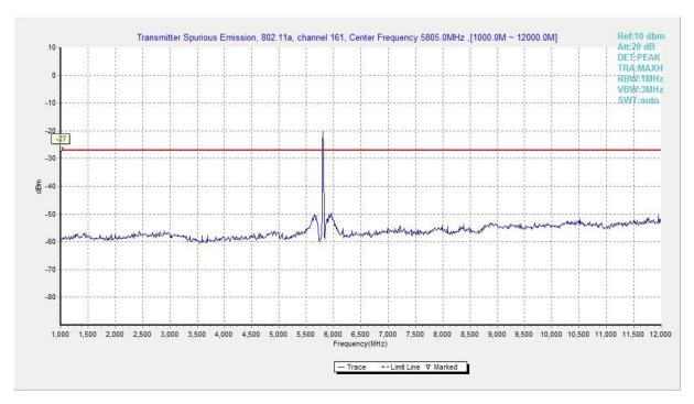
Fig. 80 Conducted Spurious Emission (802.11a, Ch161, 1 GHz -12 GHz)
