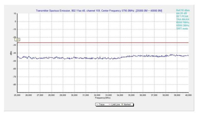
Fig. 122 Conducted Spurious Emission (802.11ac-HT40, Ch159, 25 GHz-40 GHz)
