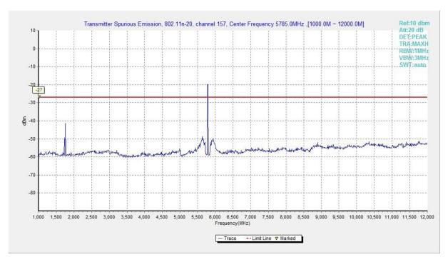
Fig. 88 Conducted Spurious Emission (802.11n-HT20, Ch157, 1 GHz -12 GHz)
