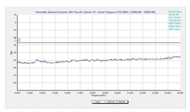
Fig. 117 Conducted Spurious Emission (802.11ac-HT40, Ch151, 12 GHz-25 GHz)
