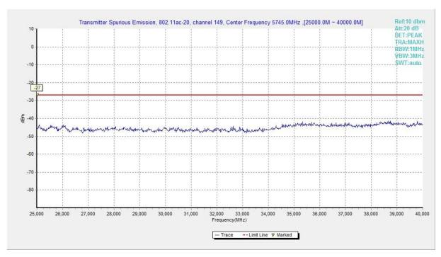
Fig. 98 Conducted Spurious Emission (802.11ac-HT20, Ch149, 25 GHz-40 GHz)
