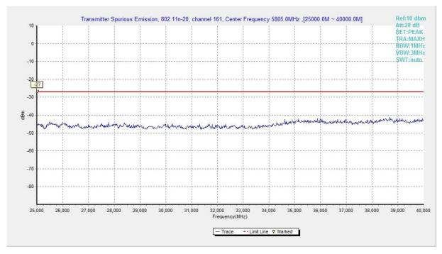
Fig. 94 Conducted Spurious Emission (802.11n-HT20, Ch161, 25 GHz-40 GHz)
