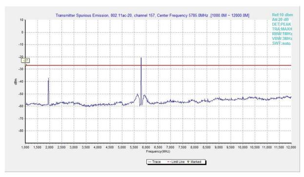
Fig. 100 Conducted Spurious Emission (802.11ac-HT20, Ch157, 1 GHz -12 GHz)
