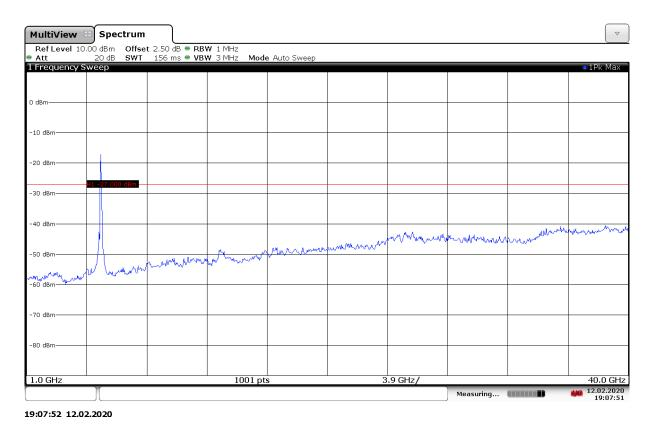
Fig. 68 Conducted Spurious Emission (802.11ax-HE40-RU242-right, Ch159, 1 GHz-40 GHz)
