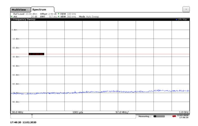
Fig. 131 Conducted Spurious Emission (802.11ax-HE20-RU106-right, Ch161, 30 MHz-1 GHz)
