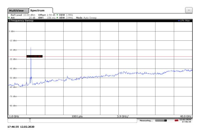
Fig. 132 Conducted Spurious Emission (802.11ax-HE20-RU106-right, Ch161, 1 GHz-40 GHz)
