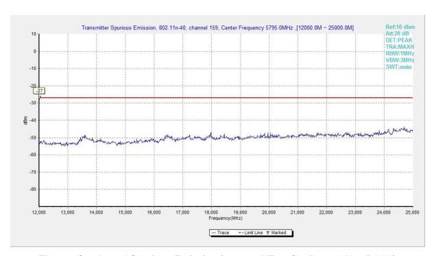
Fig. 113 Conducted Spurious Emission (802.11n-HT40, Ch159, 12 GHz-25 GHz)
