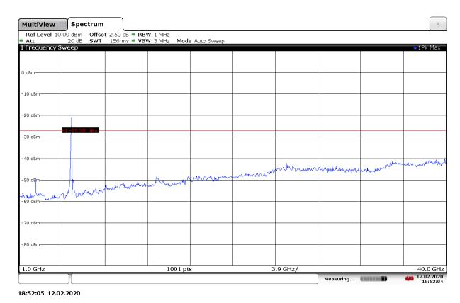
Fig. 134 Conducted Spurious Emission (802.11ax-HE40-RU242-right, Ch151, 1 GHz-40 GHz)
