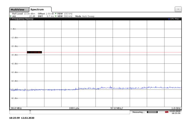
Fig. 69 Conducted Spurious Emission (802.11ax-HE80-RU484-right, Ch155, 30 MHz-1 GHz)
