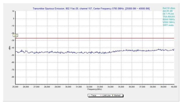
Fig. 102 Conducted Spurious Emission (802.11ac-HT20, Ch157, 25 GHz-40 GHz)
