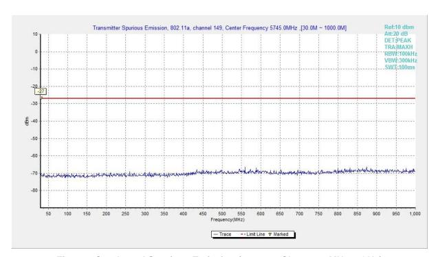
Fig. 71 Conducted Spurious Emission (802.11a, Ch149, 30 MHz-1 GHz)
