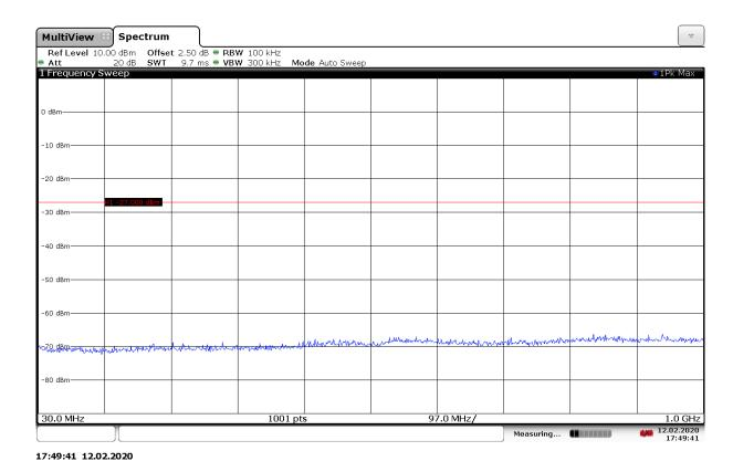
Fig. 129 Conducted Spurious Emission (802.11ax-HE20-RU106-right, Ch157, 30 MHz-1 GHz)
