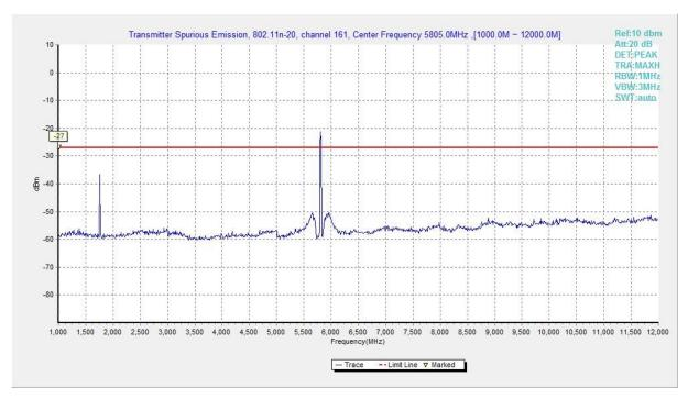
Fig. 92 Conducted Spurious Emission (802.11n-HT20, Ch161, 1 GHz -12 GHz)
