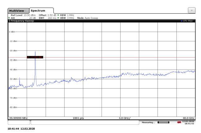
Fig. 136 Conducted Spurious Emission (802.11ax-HE40-RU242-right, Ch159, 1 GHz-40 GHz)
