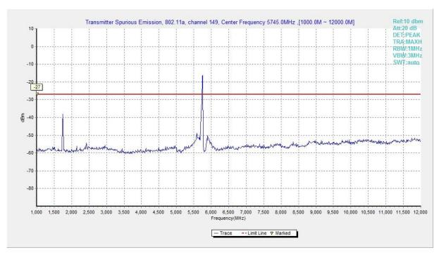
Fig. 72 Conducted Spurious Emission (802.11a, Ch149, 1 GHz -12 GHz)
