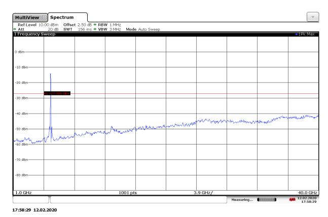
Fig. 128 Conducted Spurious Emission (802.11ax-HE20-RU106-right, Ch149, 1 GHz-40 GHz)
