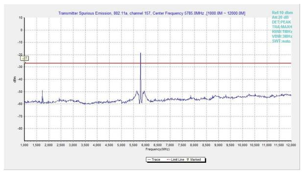
Fig. 76 Conducted Spurious Emission (802.11a, Ch157, 1 GHz -12 GHz)
