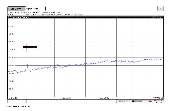
Fig. 138 Conducted Spurious Emission (802.11ax-HE80-RU484-right, Ch155, 1 GHz-40 GHz)
