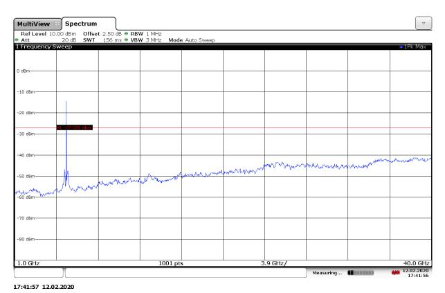
Fig. 64 Conducted Spurious Emission (802.11ax-HE20-RU106-right, Ch161, 1 GHz-40 GHz)
