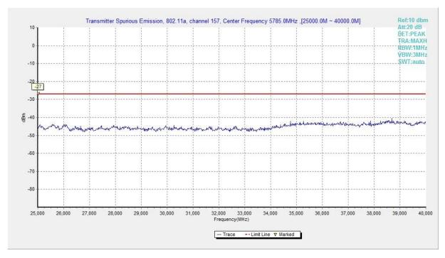
Fig. 78 Conducted Spurious Emission (802.11a, Ch157, 25 GHz-40 GHz)
