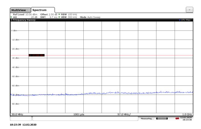
Fig. 137 Conducted Spurious Emission (802.11ax-HE80-RU484-right, Ch155, 30 MHz-1 GHz)
