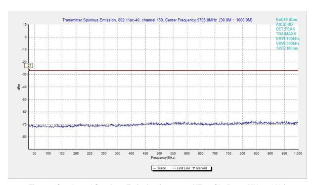
Fig. 119 Conducted Spurious Emission (802.11ac-HT40, Ch159, 30 MHz-1 GHz)
