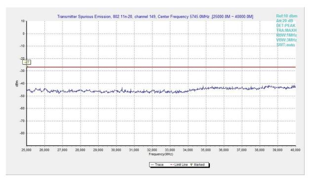
Fig. 86 Conducted Spurious Emission (802.11n-HT20, Ch149, 25 GHz-40 GHz)
