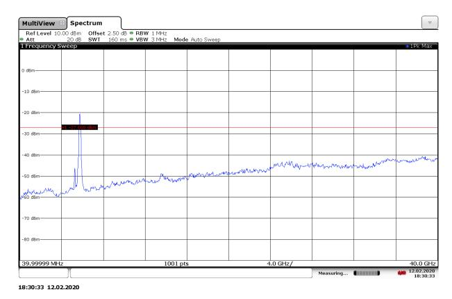
Fig. 70 Conducted Spurious Emission (802.11ax-HE80-RU484-right, Ch155, 1 GHz-40 GHz)
