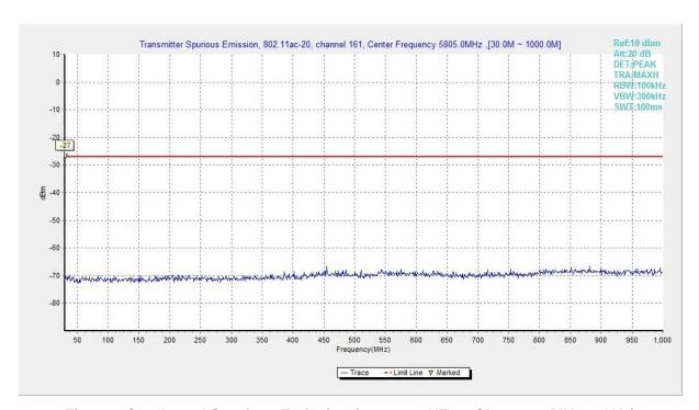
Fig. 103 Conducted Spurious Emission (802.11ac-HT20, Ch161, 30 MHz-1 GHz)
