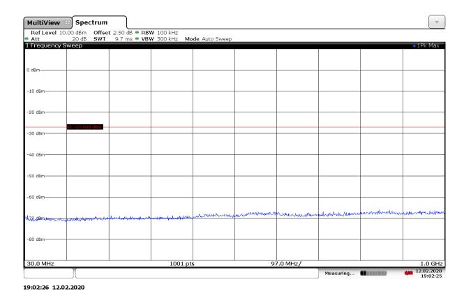
Fig. 67 Conducted Spurious Emission (802.11ax-HE40-RU242-right, Ch159, 30 MHz-1 GHz)
