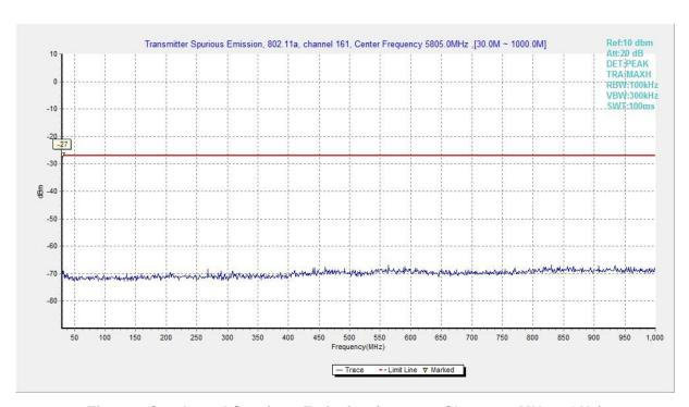
Fig. 79 Conducted Spurious Emission (802.11a, Ch161, 30 MHz-1 GHz)
