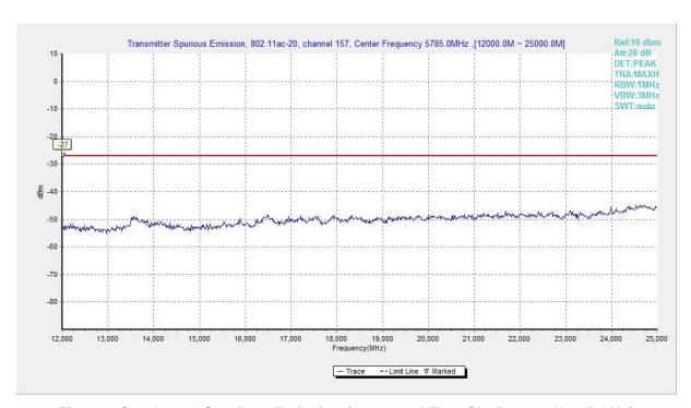
Fig. 101 Conducted Spurious Emission (802.11ac-HT20, Ch157, 12 GHz-25 GHz)
