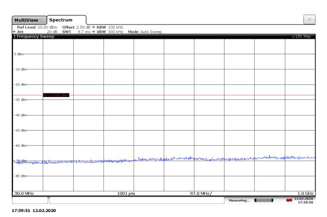
Fig. 127 Conducted Spurious Emission (802.11ax-HE20-RU106-right, Ch149, 30 MHz-1 GHz)
