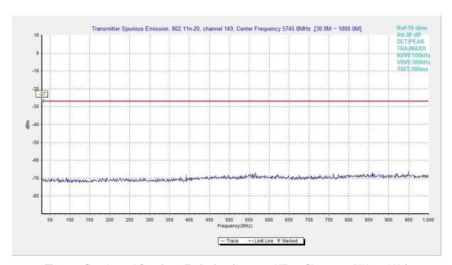
Fig. 83 Conducted Spurious Emission (802.11n-HT20, Ch149, 30 MHz-1 GHz)
