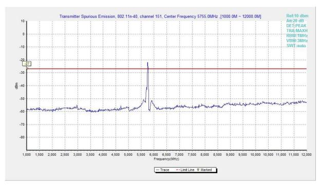
Fig. 108 Conducted Spurious Emission (802.11n-HT40, Ch151, 1 GHz -12 GHz)
