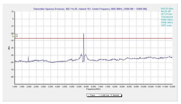
Fig. 24 Conducted Spurious Emission (802.11n-HT20, Ch161, 1 GHz -12 GHz)
