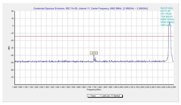
Fig.A.6.1.169 Transmitter Spurious Emission - Conducted (802.11n-HT20, Ch11, 1 GHz-2.5 GHz)
