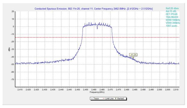
Fig.A.6.1.167 Transmitter Spurious Emission - Conducted (802.11n-HT20, Ch11, Center Frequency)
