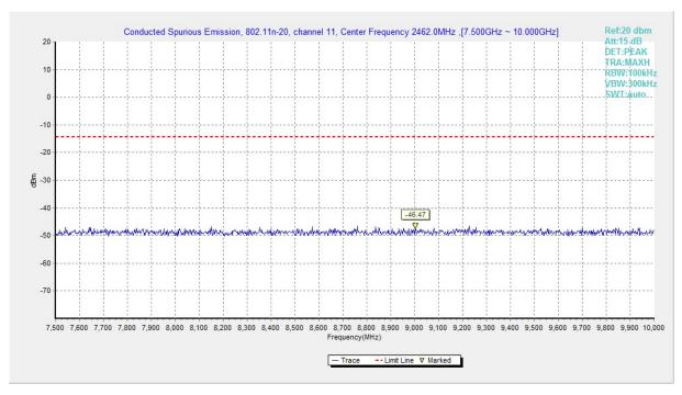
Fig.A.6.1.171 Transmitter Spurious Emission - Conducted (802.11n-HT20, Ch11, 7.5 GHz-10 GHz)
