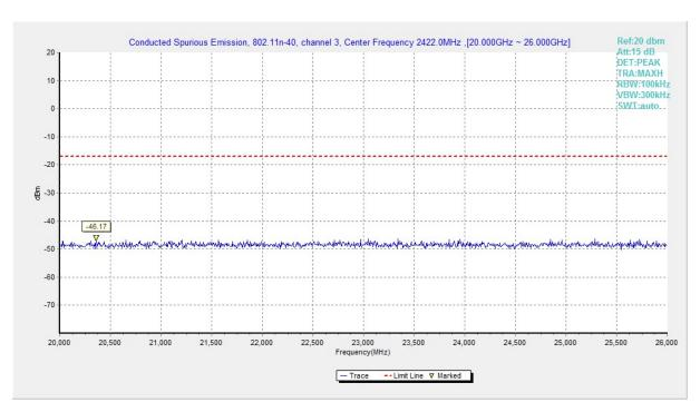
Fig.A.6.1.182 Transmitter Spurious Emission - Conducted (802.11n-HT40, Ch3, 20 GHz-26 GHz)
