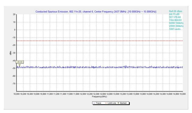
Fig.A.6.1.164 Transmitter Spurious Emission - Conducted (802.11n-HT20, Ch6, 10 GHz-15 GHz)
