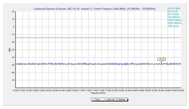
Fig.A.6.1.173 Transmitter Spurious Emission - Conducted (802.11n-HT20, Ch11, 15 GHz-20 GHz)
