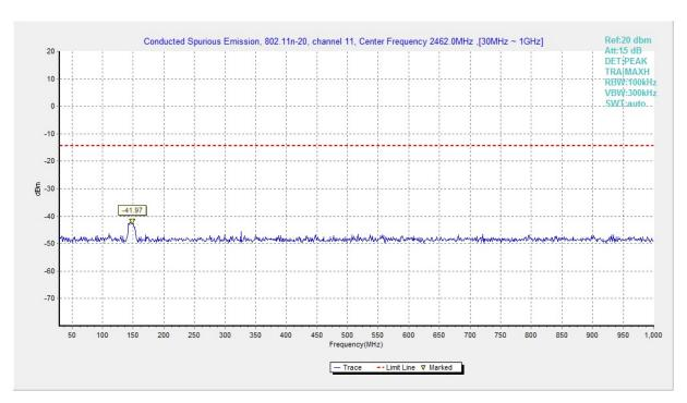
Fig.A.6.1.168 Transmitter Spurious Emission - Conducted (802.11n-HT20, Ch11, 30 MHz-1 GHz)
