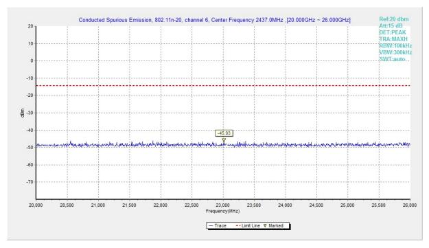
Fig.A.6.1.166 Transmitter Spurious Emission - Conducted (802.11n-HT20, Ch6, 20 GHz-26 GHz)
