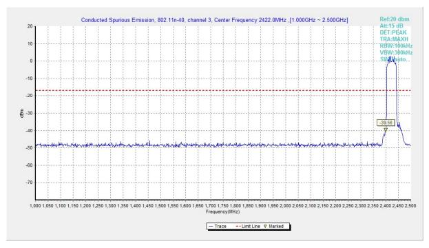
Fig.A.6.1.177 Transmitter Spurious Emission - Conducted (802.11n-HT40, Ch3, 1 GHz-2.5 GHz)
