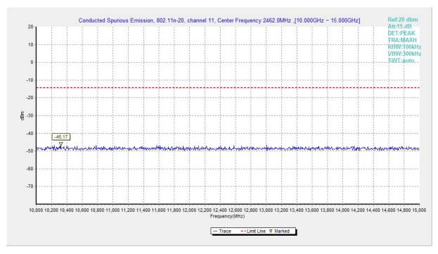
Fig.A.6.1.172 Transmitter Spurious Emission - Conducted (802.11n-HT20, Ch11, 10 GHz-15 GHz)
