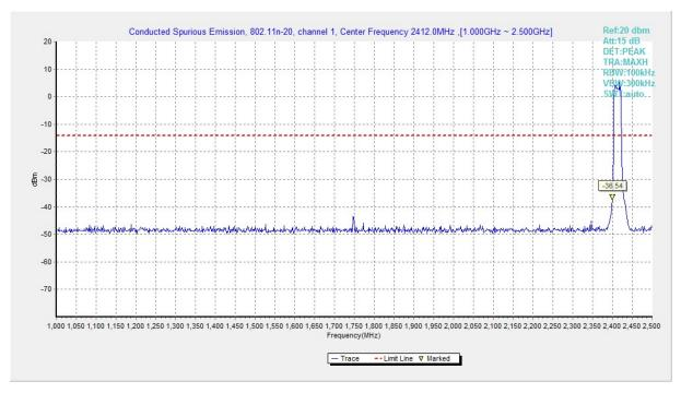
Fig.A.6.1.153 Transmitter Spurious Emission - Conducted (802.11n-HT20, Ch1, 1 GHz-2.5 GHz)
