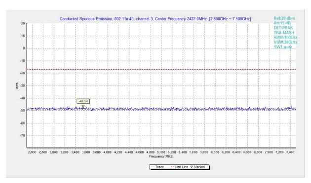
Fig.A.6.1.178 Transmitter Spurious Emission - Conducted (802.11n-HT40, Ch3, 2.5 GHz-7.5 GHz)
