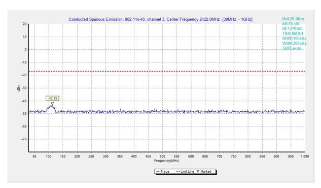
Fig.A.6.1.176 Transmitter Spurious Emission - Conducted (802.11n-HT40, Ch3, 30 MHz-1 GHz)
