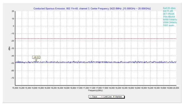
Fig.A.6.1.181 Transmitter Spurious Emission - Conducted (802.11n-HT40, Ch3, 15 GHz-20 GHz)
