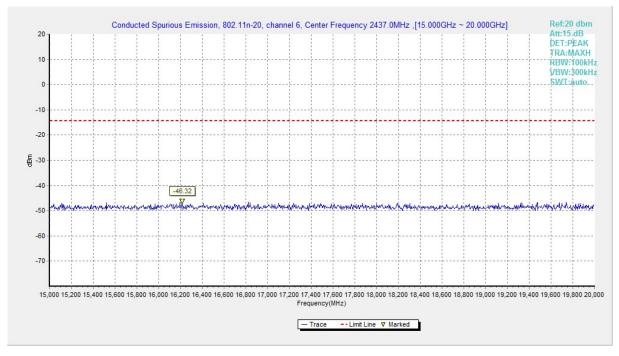
Fig.A.6.1.165 Transmitter Spurious Emission - Conducted (802.11n-HT20, Ch6, 15 GHz-20 GHz)
