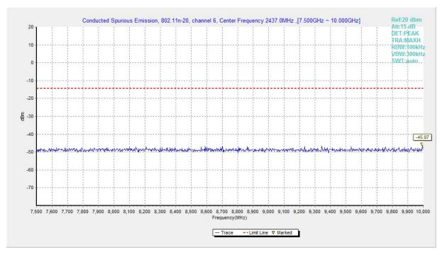
Fig.A.6.1.163 Transmitter Spurious Emission - Conducted (802.11n-HT20, Ch6, 7.5 GHz-10 GHz)
