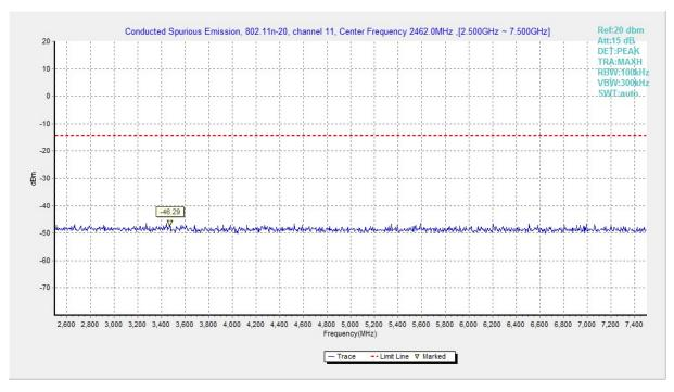
Fig.A.6.1.170 Transmitter Spurious Emission - Conducted (802.11n-HT20, Ch11, 2.5 GHz-7.5 GHz)
