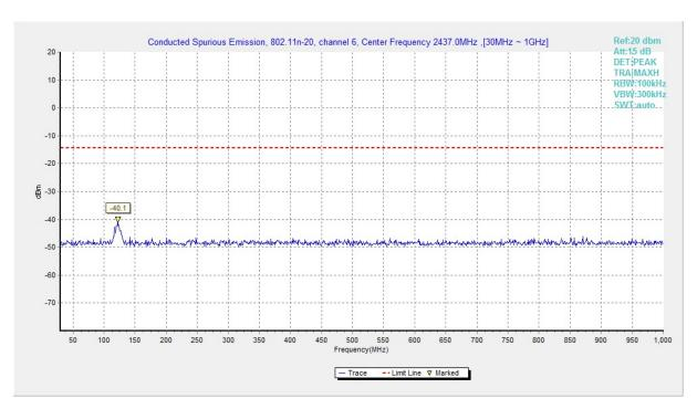
Fig.A.6.1.160 Transmitter Spurious Emission - Conducted (802.11n-HT20, Ch6, 30 MHz-1 GHz)
