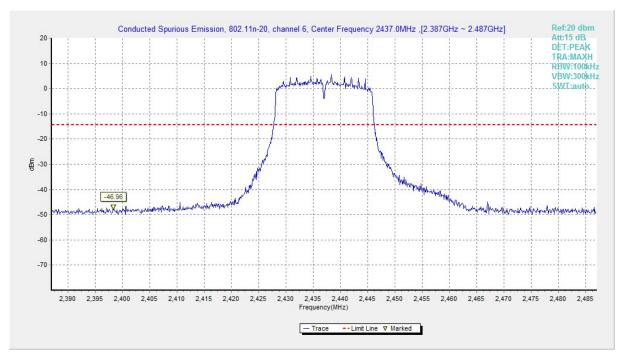
Fig.A.6.1.159 Transmitter Spurious Emission - Conducted (802.11n-HT20, Ch6, Center Frequency)
