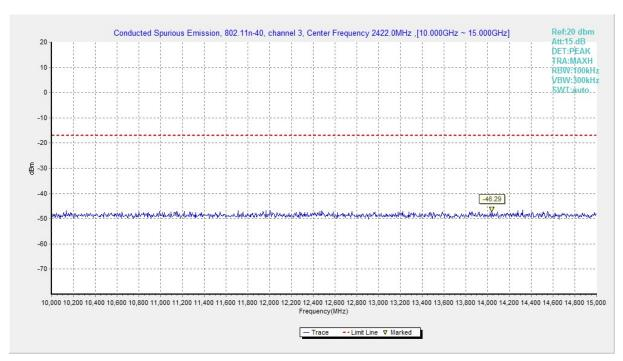
Fig.A.6.1.180 Transmitter Spurious Emission - Conducted (802.11n-HT40, Ch3, 10 GHz-15 GHz)
