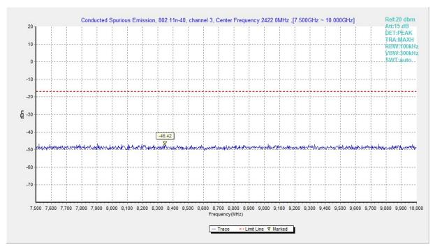
Fig.A.6.1.179 Transmitter Spurious Emission - Conducted (802.11n-HT40, Ch3, 7.5 GHz-10 GHz)
