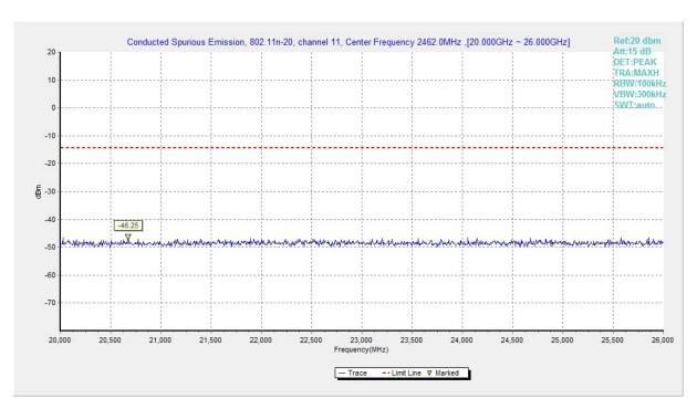
Fig.A.6.1.174 Transmitter Spurious Emission - Conducted (802.11n-HT20, Ch11, 20 GHz-26 GHz)
