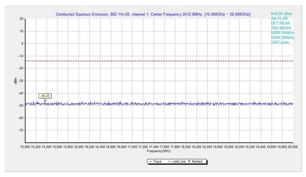
Fig.A.6.1.157 Transmitter Spurious Emission - Conducted (802.11n-HT20, Ch1, 15 GHz-20 GHz)
