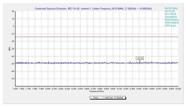
Fig.A.6.1.155 Transmitter Spurious Emission - Conducted (802.11n-HT20, Ch1, 7.5 GHz-10 GHz)
