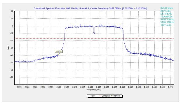
Fig.A.6.1.175 Transmitter Spurious Emission - Conducted (802.11n-HT40, Ch3, Center Frequency)
