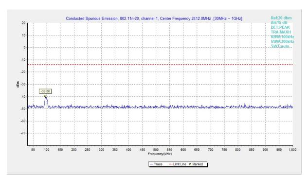
Fig.A.6.1.152 Transmitter Spurious Emission - Conducted (802.11n-HT20, Ch1, 30 MHz-1 GHz)
