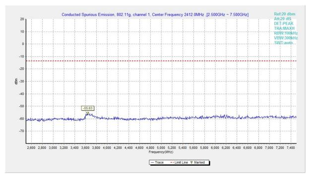
Fig.A.6.1.130 Transmitter Spurious Emission - Conducted (802.11g, Ch1, 2.5 GHz-7.5 GHz)
