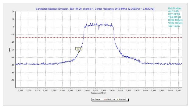
Fig.A.6.1.151 Transmitter Spurious Emission - Conducted (802.11n-HT20, Ch1, Center Frequency)
