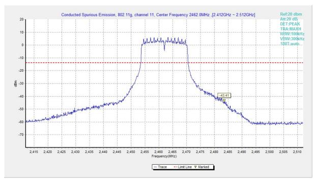
Fig.A.6.1.143 Transmitter Spurious Emission - Conducted (802.11g, Ch11, Center Frequency)
