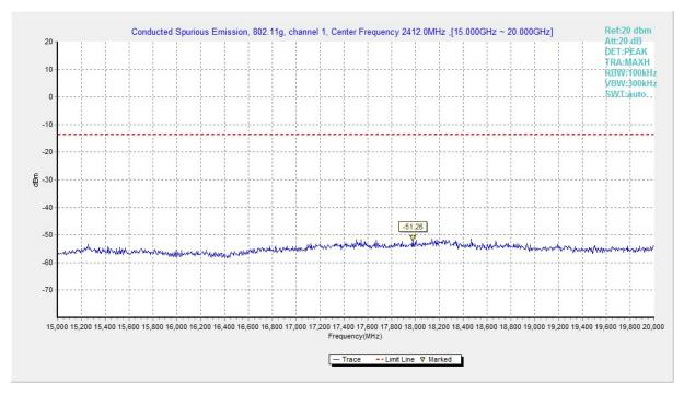
Fig.A.6.1.133 Transmitter Spurious Emission - Conducted (802.11g, Ch1, 15 GHz-20 GHz)
