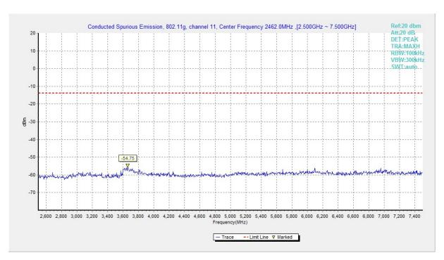
Fig.A.6.1.146 Transmitter Spurious Emission - Conducted (802.11g, Ch11, 2.5 GHz-7.5 GHz)
