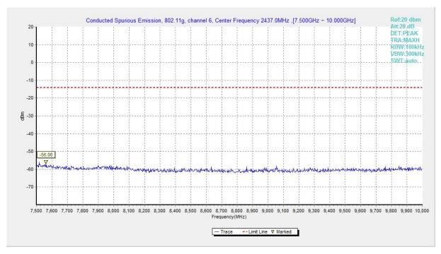
Fig.A.6.1.139 Transmitter Spurious Emission - Conducted (802.11g, Ch6, 7.5 GHz-10 GHz)
