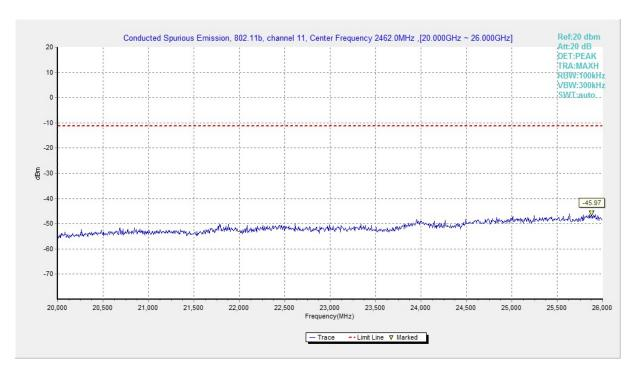
Fig.A.6.1.126 Transmitter Spurious Emission - Conducted (802.11b, Ch11, 20 GHz-26 GHz)
