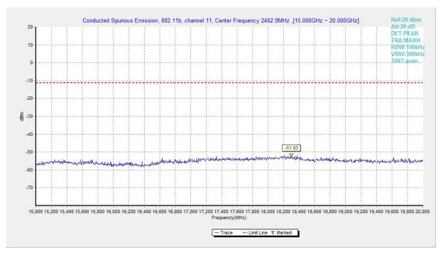
Fig.A.6.1.125 Transmitter Spurious Emission - Conducted (802.11b, Ch11, 15 GHz-20 GHz)
