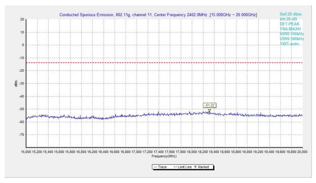
Fig.A.6.1.149 Transmitter Spurious Emission - Conducted (802.11g, Ch11, 15 GHz-20 GHz)
