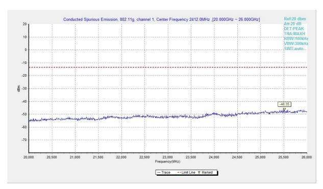
Fig.A.6.1.134 Transmitter Spurious Emission - Conducted (802.11g, Ch1, 20 GHz-26 GHz)
