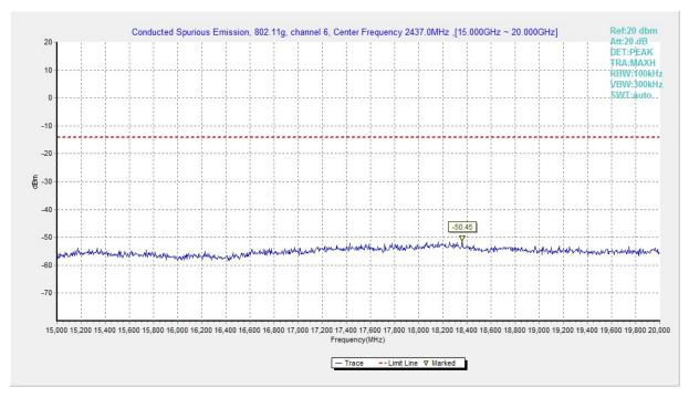
Fig.A.6.1.141 Transmitter Spurious Emission - Conducted (802.11g, Ch6, 15 GHz-20 GHz)
