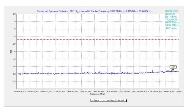
Fig.A.6.1.140 Transmitter Spurious Emission - Conducted (802.11g, Ch6, 10 GHz-15 GHz)
