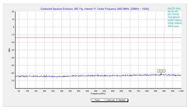
Fig.A.6.1.144 Transmitter Spurious Emission - Conducted (802.11g, Ch11, 30 MHz-1 GHz)
