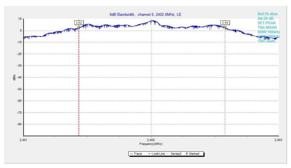
Fig.26. 6dB Bandwidth: GFSK, 2402 MHz
