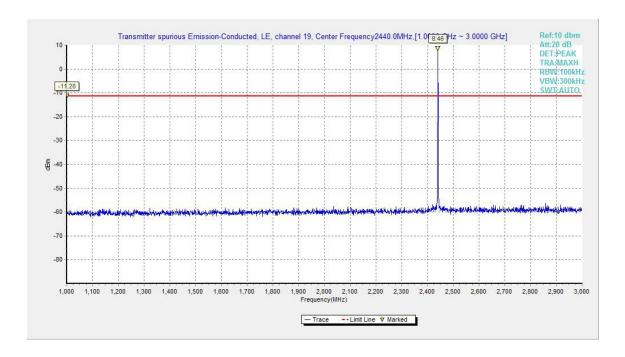
Fig.18. Transmitter Spurious Emission - Conducted: GFSK, 2440 MHz, 1GHz - 3GHz
