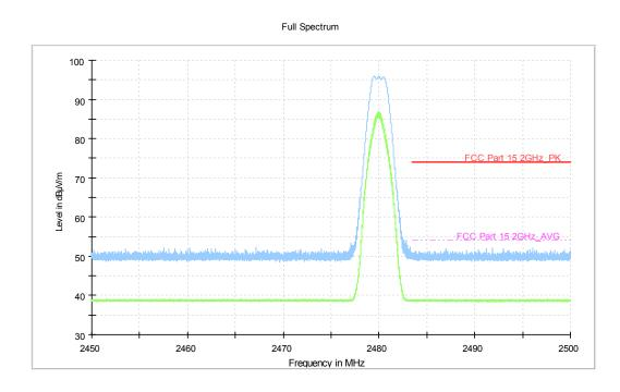
Fig.10. Frequency Band Edges: EUT4 ANT4 BLE 5.0 GFSK, 2480 MHz, Hopping Off , 2.45 GHz - 2.50GHz
