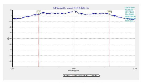
Fig.27. 6dB Bandwidth: GFSK, 2440 MHz
