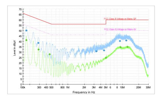
Fig.A.9.2 AC Powerline Conducted Emission-Idle EUT3(M2001J2G)+AE1+AE3+AE6 Note: The graphic result above is the maximum of the measurements for both phase line and neutral line.
