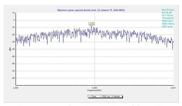
Fig.30. Maximum Power Spectral Density Level Function: GFSK, 2440 MHz
