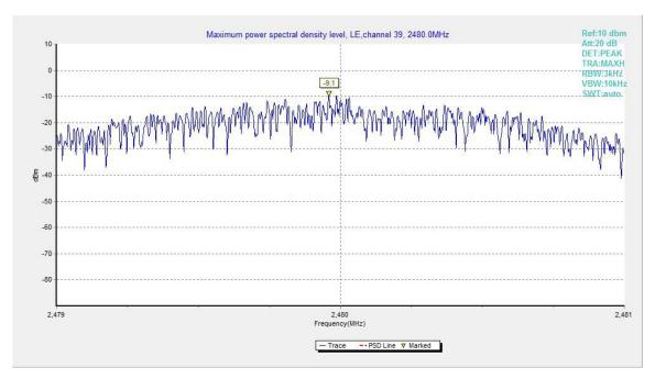
Fig.31. Maximum Power Spectral Density Level Function: GFSK, 2480 MHz
