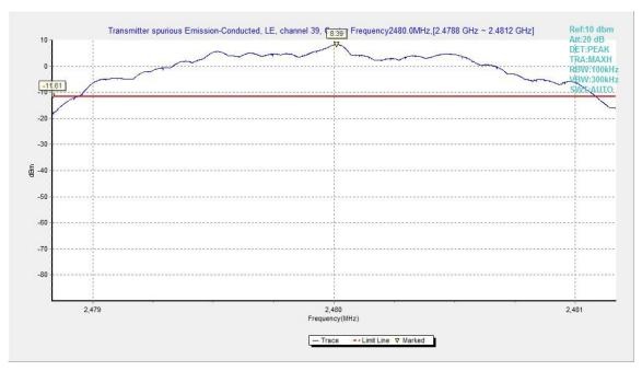
Fig.21. Transmitter Spurious Emission - Conducted: GFSK, 2480 MHz
