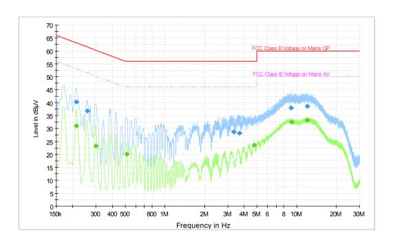
Fig.A.9.1 AC Powerline Conducted Emission- Bluetooth EUT3(M2001J2G)+AE1+AE3+AE6
