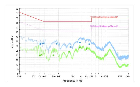
Fig.A.9.1 AC Powerline Conducted Emission- Bluetooth EUT5(M2001J2G)+AE11+AE13+AE16
