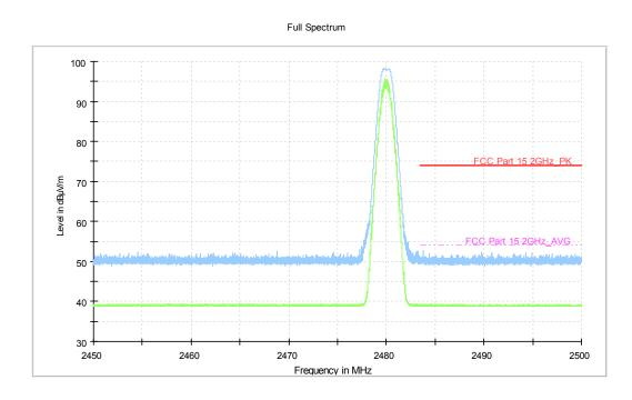
Fig.4. Frequency Band Edges: EUT3 ANT3 BLE 4.0GFSK, 2480 MHz, Hopping Off , 2.45
