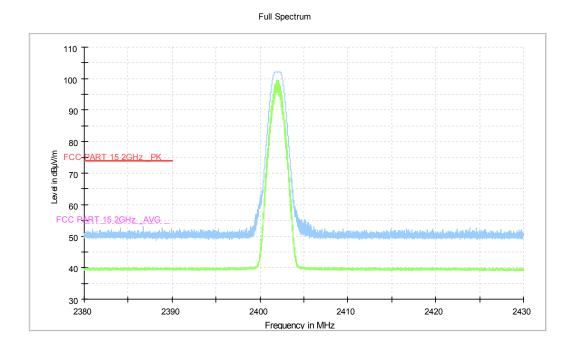
Fig.3. Frequency Band Edges: EUT3 ANT3 BLE 4.0 GFSK, 2402 MHz, Hopping Off, 2.38 GHz – 2.45GHz
