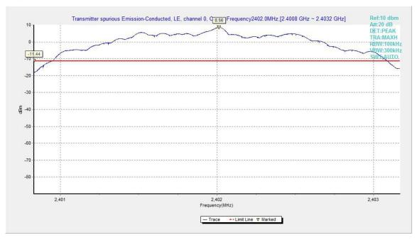
Fig.11. Transmitter Spurious Emission - Conducted: GFSK,2402MHz
