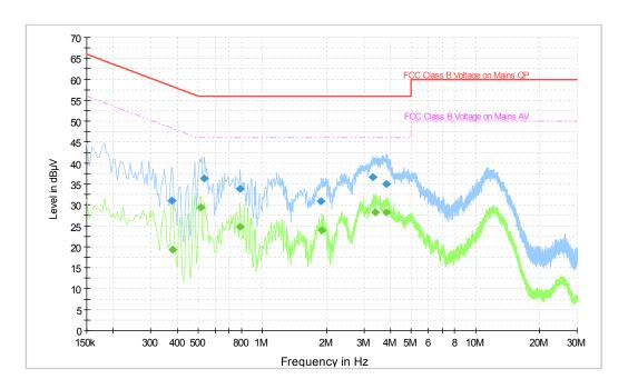
Fig.A.9.2 AC Powerline Conducted Emission-Idle EUT5(M2001J2G)+AE11+AE13+AE16
