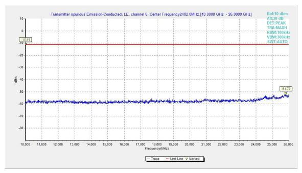
Fig.15. Transmitter Spurious Emission - Conducted: GFSK, 2402 MHz,10GHz - 26GHz
