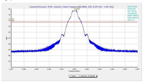
Fig.34. Conducted spurious emission: GFSK, Channel 0,2402MHz
