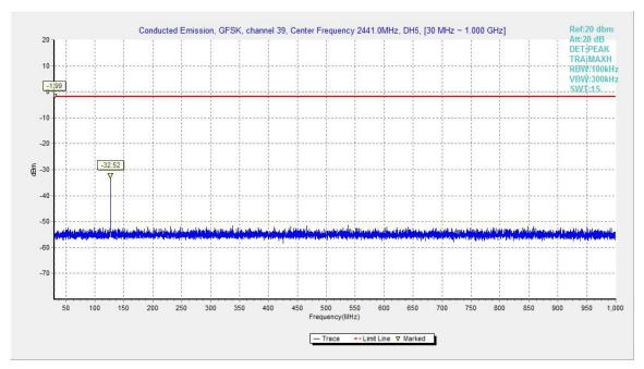
Fig.40. Conducted spurious emission: GFSK, Channel 39, 30MHz - 1GHz
