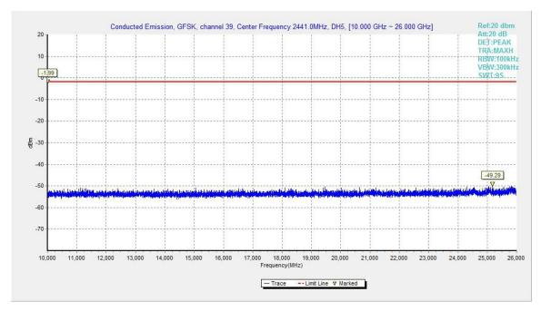
Fig.43. Conducted spurious emission: GFSK, Channel 39, 10GHz – 26GHz
