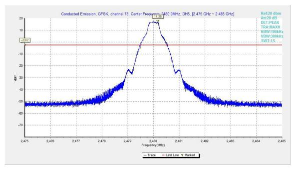
Fig.44. Conducted spurious emission: GFSK, Channel 78, 2480MHz
