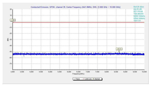
Fig.42. Conducted spurious emission: GFSK, Channel 39, 3GHz – 10GHz
