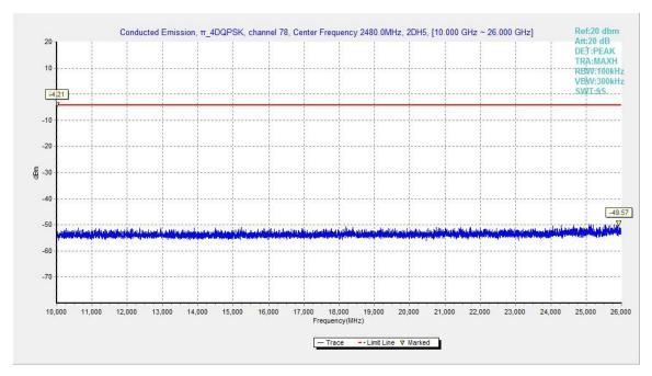
Fig.63. Conducted spurious emission: π/4 DQPSK, Channel 78, 10GHz - 26GHz
