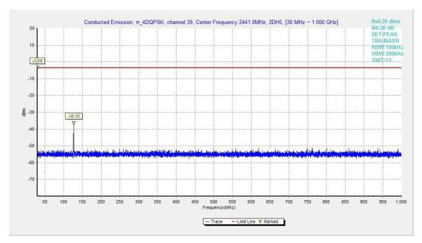
Fig.55. Conducted spurious emission:  $\pi/4$  DQPSK, Channel 39, 30MHz - 1GHz
