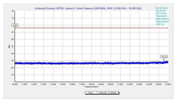
Fig.68. Conducted spurious emission: 8DPSK, Channel 0,10GHz - 26GHz
