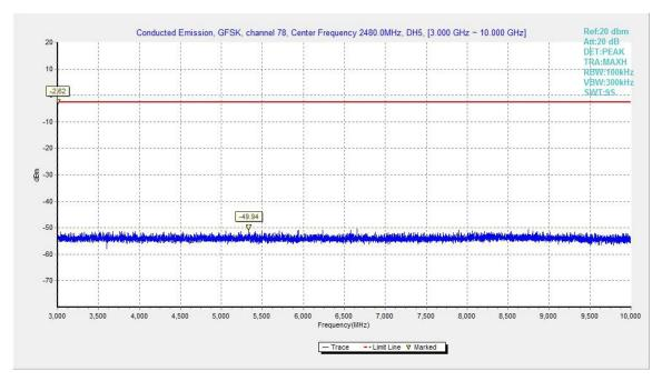
Fig.47. Conducted spurious emission: GFSK, Channel 78, 3GHz - 10GHz
