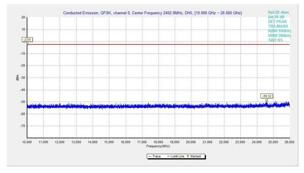
Fig.38. Conducted spurious emission: GFSK, Channel 0,10GHz - 26GHz
