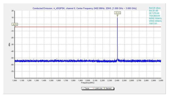
Fig.51. Conducted spurious emission:  $\pi/4$  DQPSK, Channel 0, 1GHz - 3GHz
