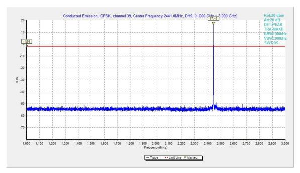
Fig.41. Conducted spurious emission: GFSK, Channel 39, 1GHz – 3GHz
