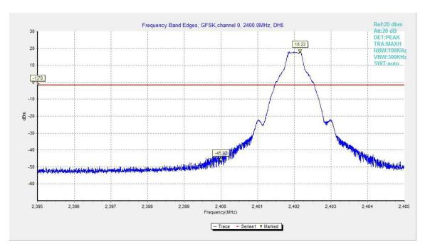
Fig.10. Frequency Band Edges: GFSK, Channel 0, Hopping Off
