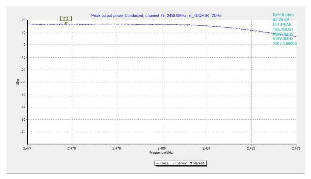
Fig.6. Peak Output Power -Conducted: Antenna 3, π/4 DQPSK, Channel 78,
