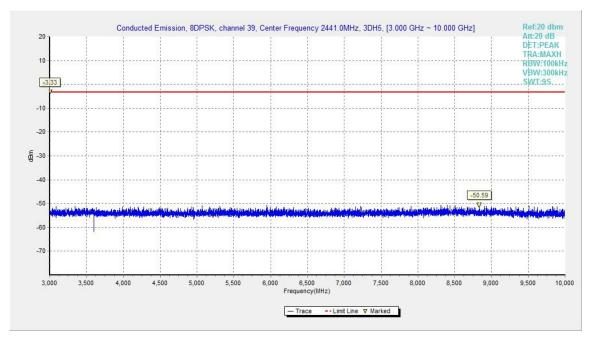
Fig.72. Conducted spurious emission: 8DPSK, Channel 39, 3GHz - 10GHz
