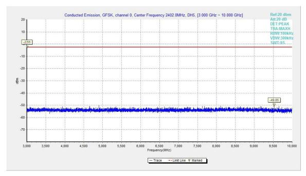
Fig.37. Conducted spurious emission: GFSK, Channel 0, 3GHz - 10GHz
