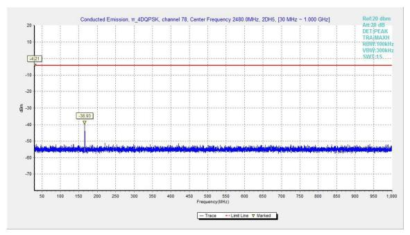
Fig.60. Conducted spurious emission: π/4 DQPSK, Channel 78, 30MHz - 1GHz
