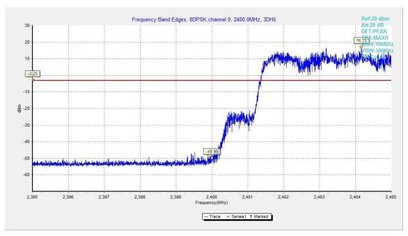
Fig.19. Frequency Band Edges: 8DPSK, Channel 0, Hopping On
