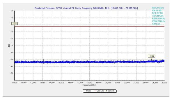
Fig.48. Conducted spurious emission: GFSK, Channel 78, 10GHz - 26GHz
