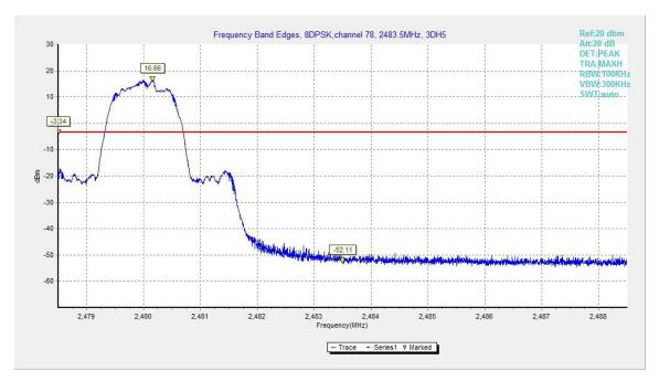
Fig.20. Frequency Band Edges: 8DPSK, Channel 78, Hopping Off
