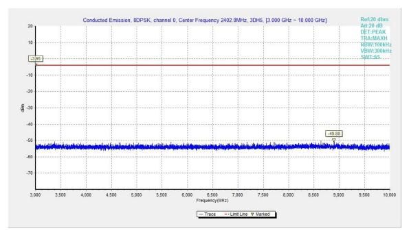
Fig.67. Conducted spurious emission: 8DPSK, Channel 0, 3GHz - 10GHz
