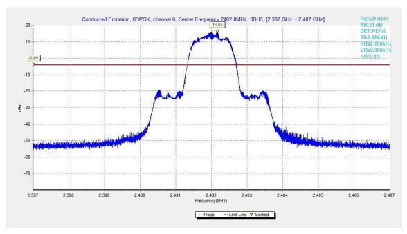
Fig.64. Conducted spurious emission: 8DPSK, Channel 0,2402MHz
