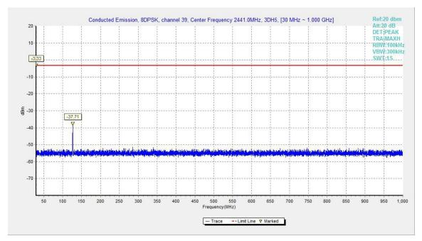
Fig.70. Conducted spurious emission: 8DPSK, Channel 39, 30MHz - 1GHz
