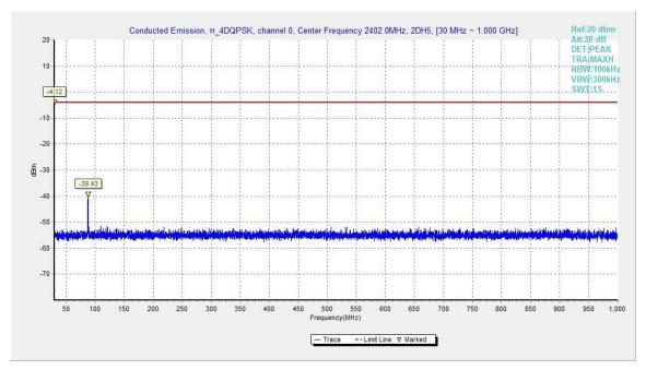
Fig.50. Conducted spurious emission:  $\pi/4$  DQPSK, Channel 0, 30MHz - 1GHz
