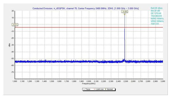
Fig.61. Conducted spurious emission:  $\pi/4$  DQPSK, Channel 78, 1GHz - 3GHz
