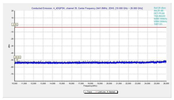
Fig.58. Conducted spurious emission:  $\pi/4$  DQPSK, Channel 39, 10GHz - 26GHz
