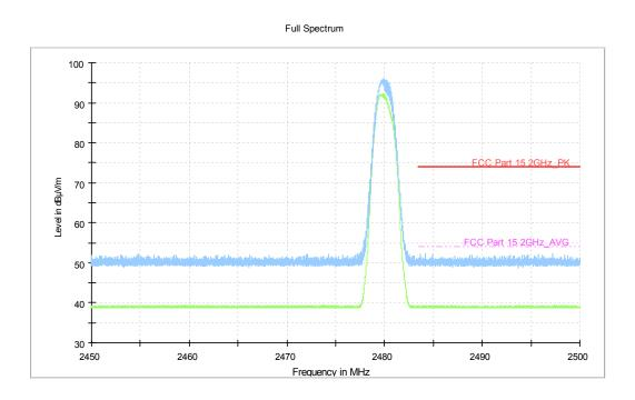
Fig.27. Frequency Band Edges: EUT3 ANT3 8DPSK, Channel 78, 2.38 GHz - 2.45GHz
