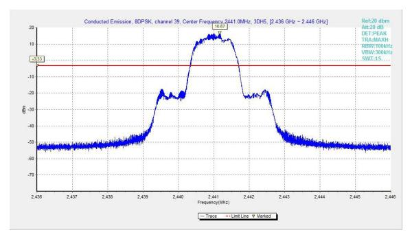
Fig.69. Conducted spurious emission: 8DPSK, Channel 39, 2441MHz
