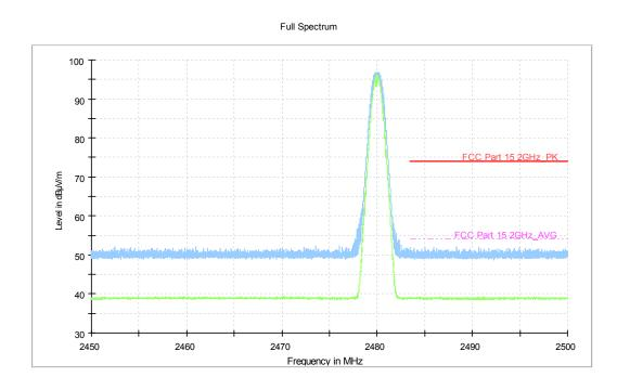
Fig.23. Frequency Band Edges: EUT3 ANT3 GFSK, Channel 78, Hopping Off, ch11, 2.45 GHz - 2.50GHz
