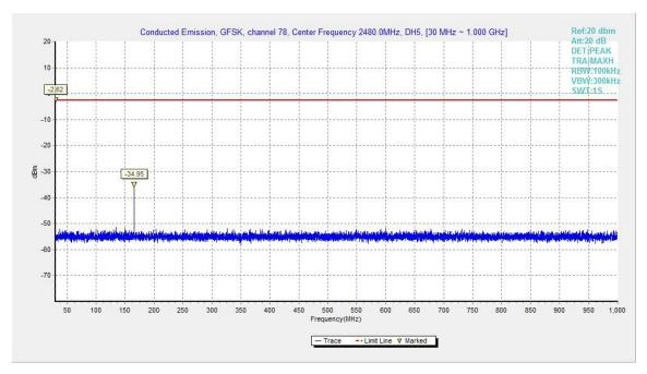
Fig.45. Conducted spurious emission: GFSK, Channel 78, 30MHz - 1GHz
