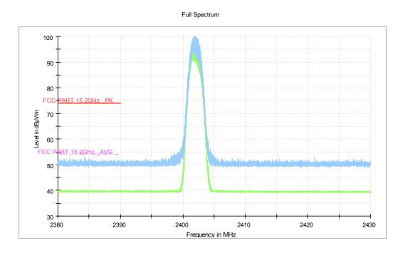
Fig.26. Frequency Band Edges: EUT3 ANT3 DPSK, Channel 0, 2.38 GHz - 2.45GHz
