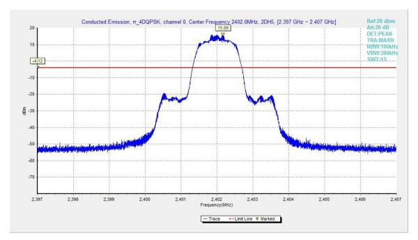
Fig.49. Conducted spurious emission:  $\pi/4$  DQPSK, Channel 0,2402MHz
