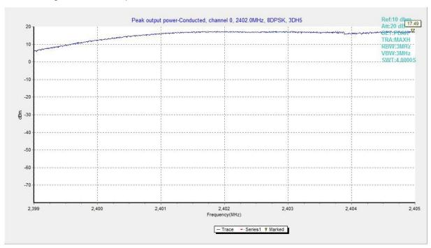
Fig.7. Peak Output Power -Conducted: Antenna 3, 8DPSK, Channel 0,
