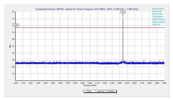
Fig.71. Conducted spurious emission: 8DPSK, Channel 39, 1GHz - 3GHz
