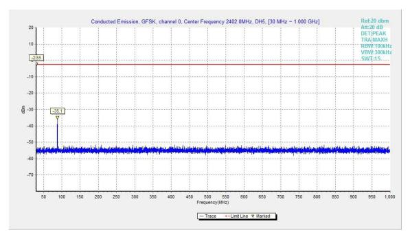
Fig.35. Conducted spurious emission: GFSK, Channel 0, 30MHz - 1GHz
