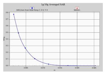
Fig. 1-49 Z-Scan at power reference point (5 GHz)
