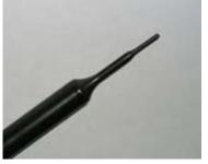
Picture C.2Near-field Probe
