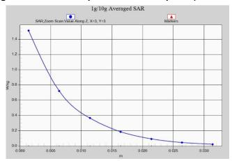
Fig. 1-47 Z-Scan at power reference point (2450 MHz)
