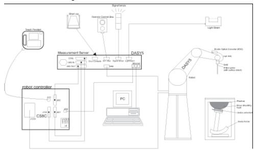
**Picture C.1SAR Lab Test Measurement Set-up**
