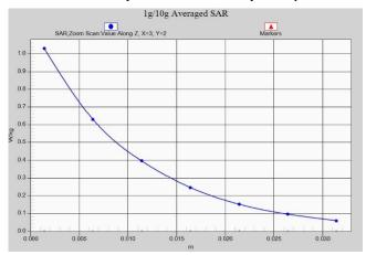
Fig. 1-26 Z-Scan at power reference point (WCDMA1900)
