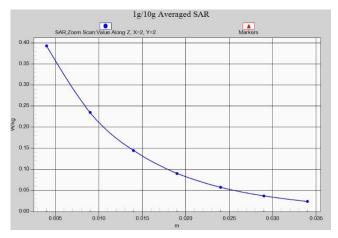
Fig. 1-31 Z-Scan at power reference point (WCDMA850)
