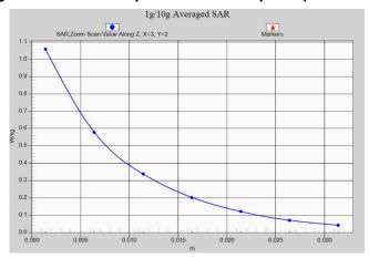
Fig. 1-33 Z-Scan at power reference point (LTE Band2)
