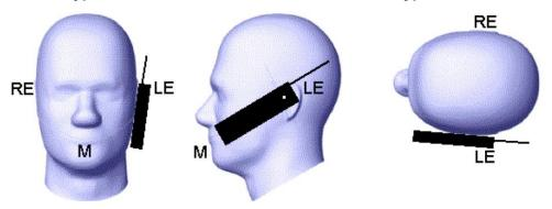
Picture D.2 Cheek position of the wireless device on the left side of SAM
