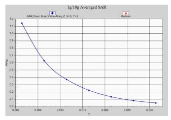
Fig. 1-28 Z-Scan at power reference point (WCDMA1700)
