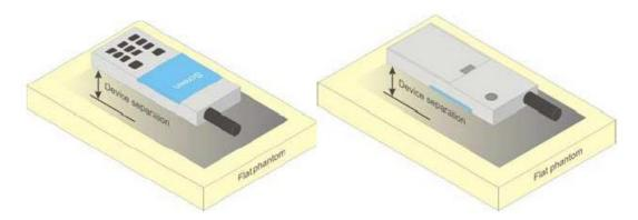
Picture D.4Test positions for body-worn devices
