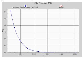
Fig. 1-48 Z-Scan at power reference point (5 GHz)
