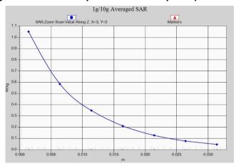
Fig. 1-36 Z-Scan at power reference point (LTE Band4)
