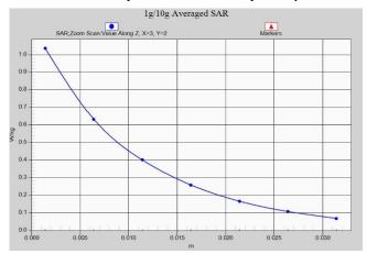
Fig. 1-29 Z-Scan at power reference point (WCDMA1700)
