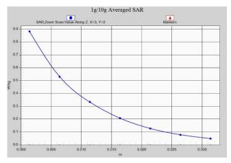
Fig. 1-34 Z-Scan at power reference point (LTE Band2)
