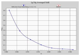
Fig. 1-44 Z-Scan at power reference point (LTE Band38)
