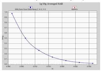
Fig. 1-41 Z-Scan at power reference point (LTE Band 7)
