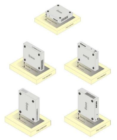
Picture D.5 Test positions for desktop devices
