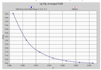
Fig. 1-20 Z-Scan at power reference point (LTE Band38)
