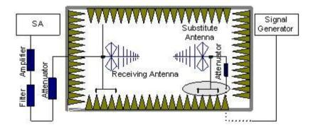
In the chamber, a substitution antenna for the frequency band of interest is placed at the reference point of the chamber. An RF Signal source for the frequency band of interest is connected to the substitution antenna with a cable that has been constructed to not interfere with the radiation pattern of the antenna. A power  $(P_{\text{Mea}})$  is applied to the input of the
