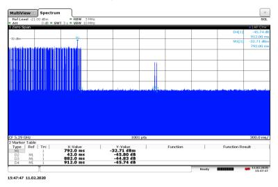
Fig.A.3 channel closing transmission time
