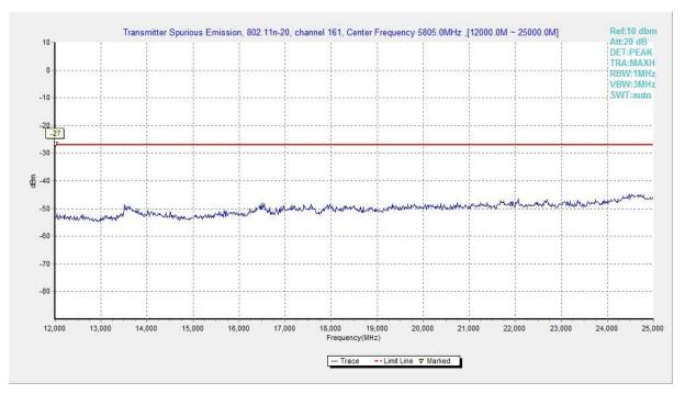
Fig. 93 Conducted Spurious Emission (802.11n-HT20, Ch161, 12 GHz-25 GHz)
