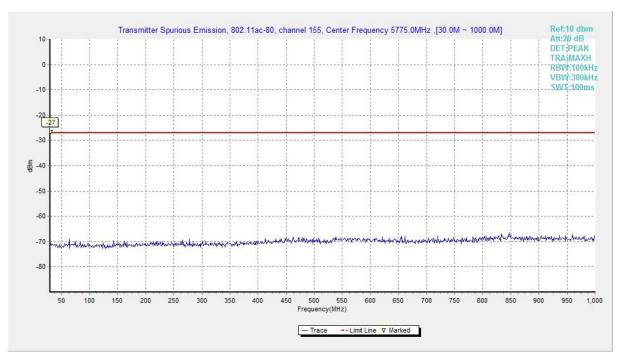
Fig. 123 Conducted Spurious Emission (802.11ac-HT80, Ch155, 30 MHz-1 GHz)
