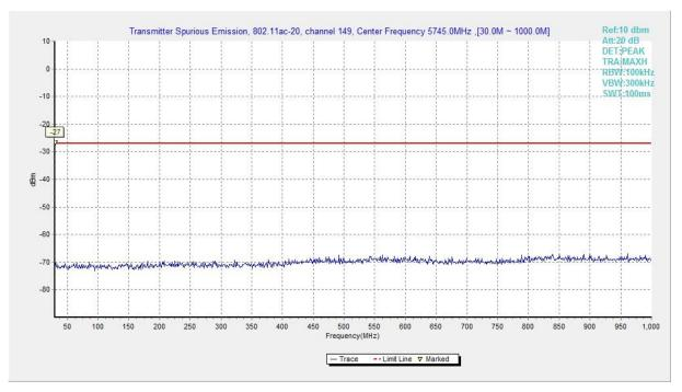
Fig. 95 Conducted Spurious Emission (802.11ac-HT20, Ch149, 30 MHz-1 GHz)
