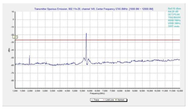
Fig. 84 Conducted Spurious Emission (802.11n-HT20, Ch149, 1 GHz -12 GHz)
