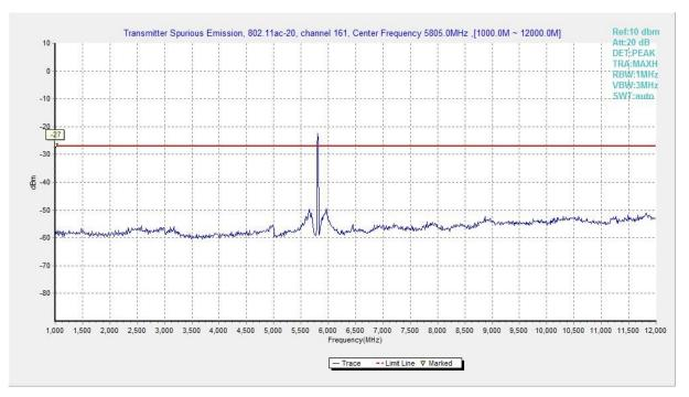
Fig. 104 Conducted Spurious Emission (802.11ac-HT20, Ch161, 1 GHz -12 GHz)
