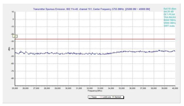
Fig. 110 Conducted Spurious Emission (802.11n-HT40, Ch151, 25 GHz-40 GHz)
