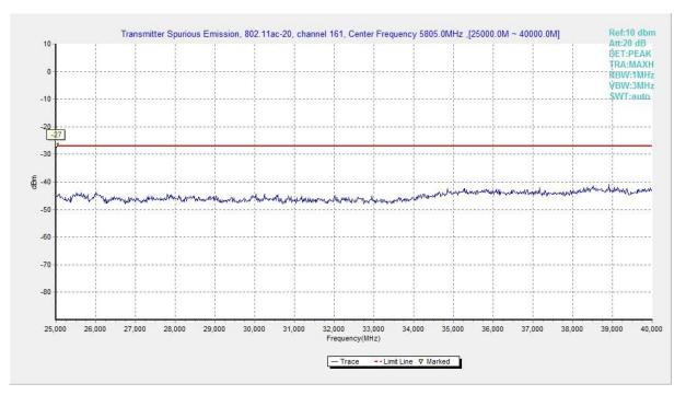
Fig. 106 Conducted Spurious Emission (802.11ac-HT20, Ch161, 25 GHz-40 GHz)
