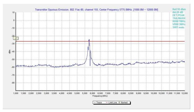
Fig. 56 Conducted Spurious Emission (802.11ac-HT80, Ch155, 1 GHz -12 GHz)
