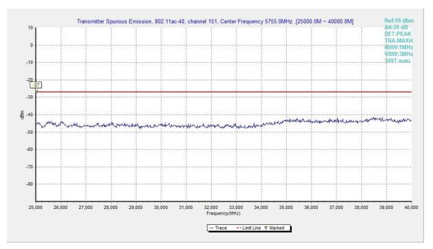
Fig. 118 Conducted Spurious Emission (802.11ac-HT40, Ch151, 25 GHz-40 GHz)
