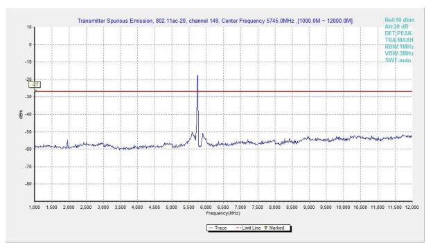
Fig. 96 Conducted Spurious Emission (802.11ac-HT20, Ch149, 1 GHz -12 GHz)
