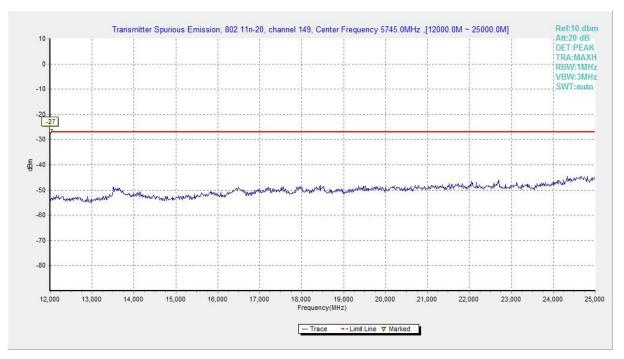
Fig. 85 Conducted Spurious Emission (802.11n-HT20, Ch149, 12 GHz-25 GHz)
