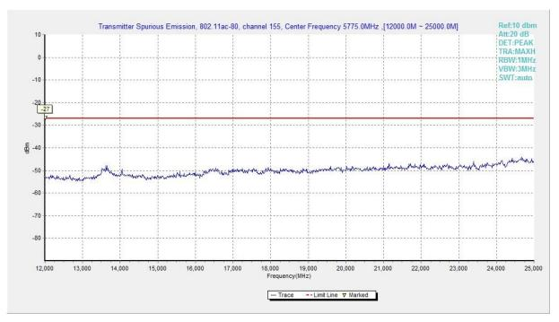
Fig. 125 Conducted Spurious Emission (802.11ac-HT80, Ch155, 12 GHz-25 GHz)
