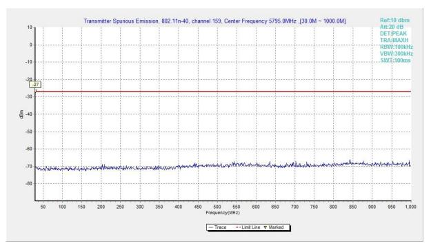
Fig. 111 Conducted Spurious Emission (802.11n-HT40, Ch159, 30 MHz-1 GHz)
