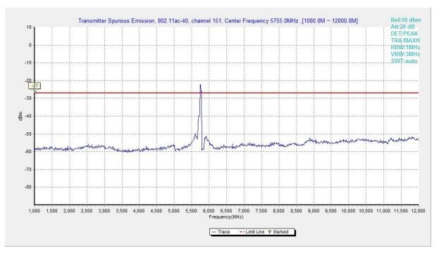
Fig. 116 Conducted Spurious Emission (802.11ac-HT40, Ch151, 1 GHz -12 GHz)
