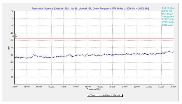
Fig. 57 Conducted Spurious Emission (802.11ac-HT80, Ch155, 12 GHz-25 GHz)
