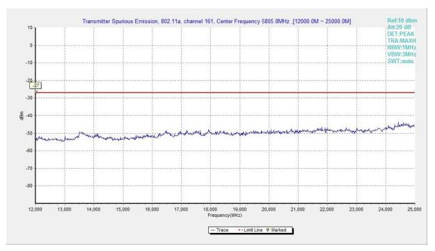
Fig. 81 Conducted Spurious Emission (802.11a, Ch161, 12 GHz-25 GHz)
