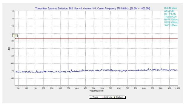
Fig. 115 Conducted Spurious Emission (802.11ac-HT40, Ch151, 30 MHz-1 GHz)
