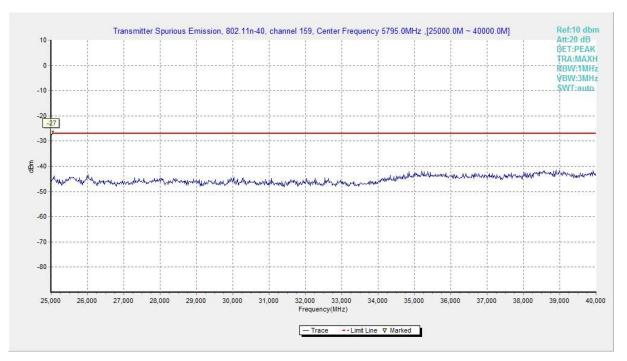
Fig. 114 Conducted Spurious Emission (802.11n-HT40, Ch159, 25 GHz-40 GHz)
