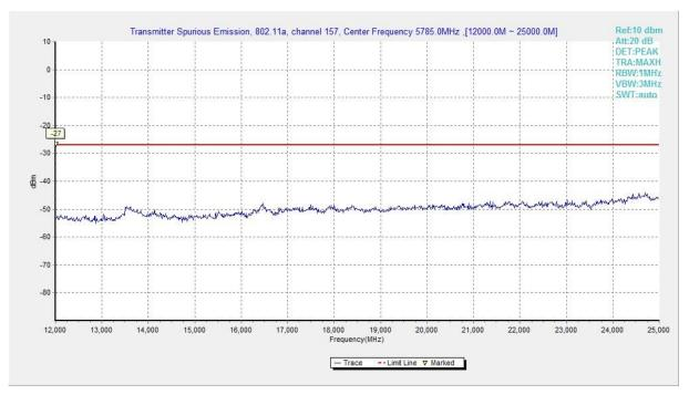
Fig. 77 Conducted Spurious Emission (802.11a, Ch157, 12 GHz-25 GHz)
