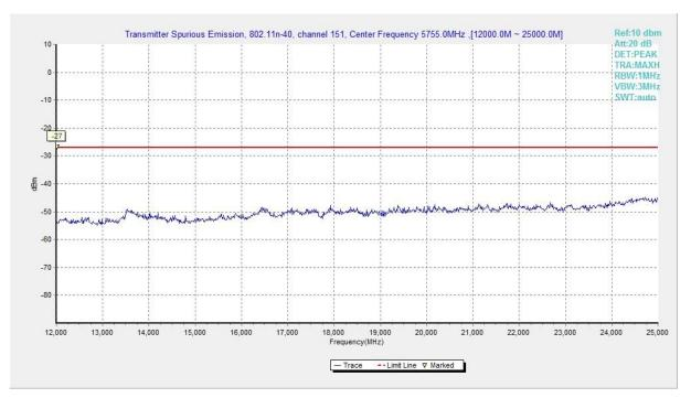
Fig. 109 Conducted Spurious Emission (802.11n-HT40, Ch151, 12 GHz-25 GHz)
