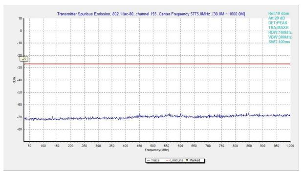
Fig. 55 Conducted Spurious Emission (802.11ac-HT80, Ch155, 30 MHz-1 GHz)
