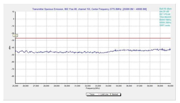
Fig. 58 Conducted Spurious Emission (802.11ac-HT80, Ch155, 25 GHz-40 GHz)
