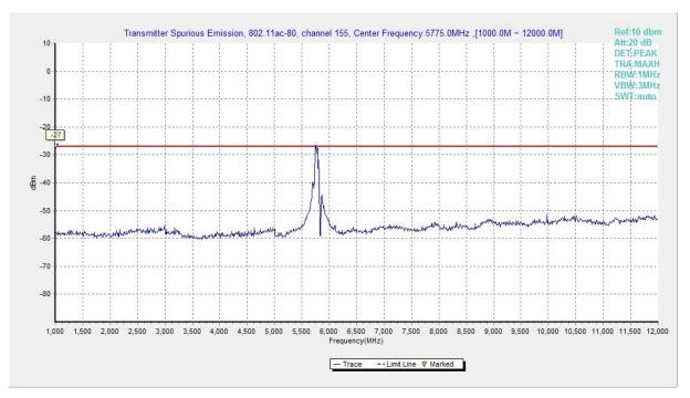
Fig. 124 Conducted Spurious Emission (802.11ac-HT80, Ch155, 1 GHz -12 GHz)
