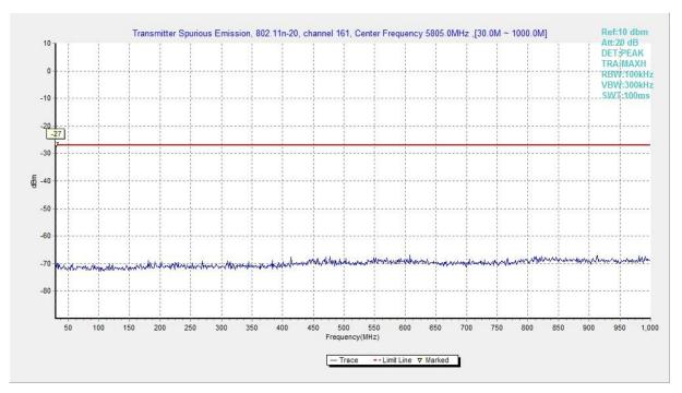
Fig. 91 Conducted Spurious Emission (802.11n-HT20, Ch161, 30 MHz-1 GHz)
