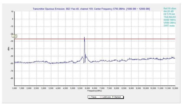
Fig. 120 Conducted Spurious Emission (802.11ac-HT40, Ch159, 1 GHz -12 GHz)
