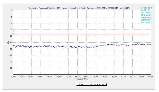
Fig. 54 Conducted Spurious Emission (802.11ac-HT40, Ch159, 25 GHz-40 GHz)
