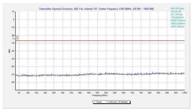
Fig. 75 Conducted Spurious Emission (802.11a, Ch157, 30 MHz-1 GHz)
