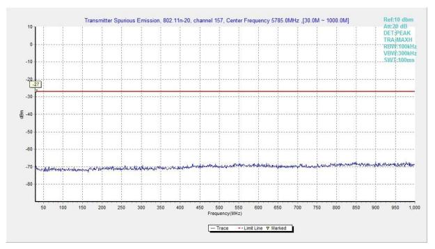
Fig. 87 Conducted Spurious Emission (802.11n-HT20, Ch157, 30 MHz-1 GHz)
