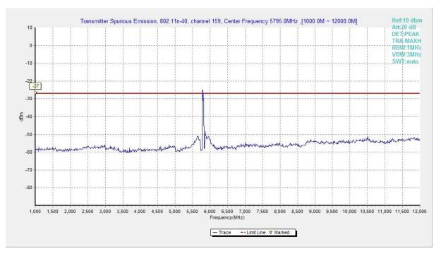
Fig. 112 Conducted Spurious Emission (802.11n-HT40, Ch159, 1 GHz -12 GHz)
