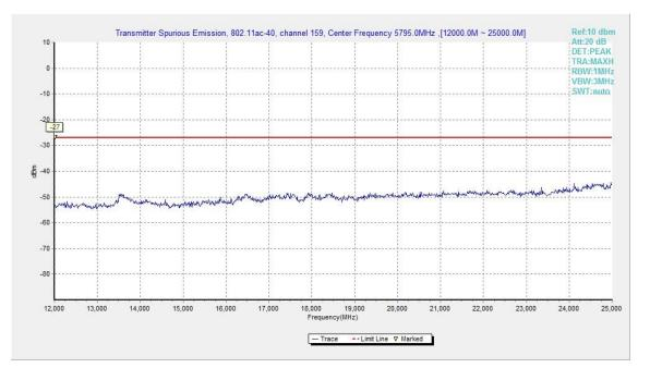
Fig. 121 Conducted Spurious Emission (802.11ac-HT40, Ch159, 12 GHz-25 GHz)
