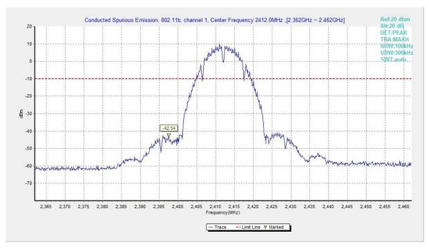
Fig.A.6.1.103 Transmitter Spurious Emission - Conducted (802.11b, Ch1, Center Frequency)
