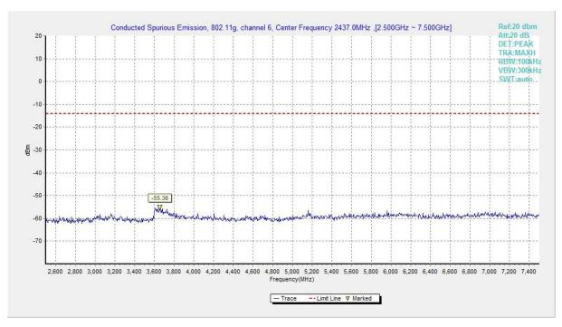
Fig.A.6.1.138 Transmitter Spurious Emission - Conducted (802.11g, Ch6, 2.5 GHz-7.5 GHz)
