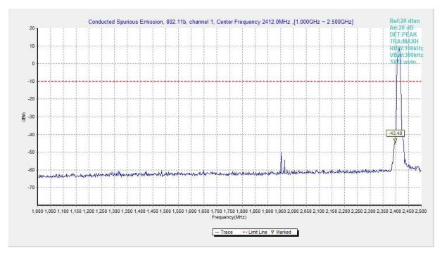
Fig.A.6.1.105 Transmitter Spurious Emission - Conducted (802.11b, Ch1, 1 GHz-2.5 GHz)
