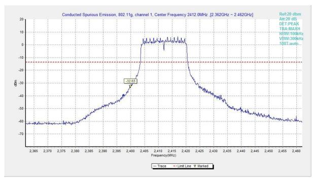
Fig.A.6.1.127 Transmitter Spurious Emission - Conducted (802.11g, Ch1, Center Frequency)
