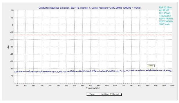
Fig.A.6.1.128 Transmitter Spurious Emission - Conducted (802.11g, Ch1, 30 MHz-1 GHz)
