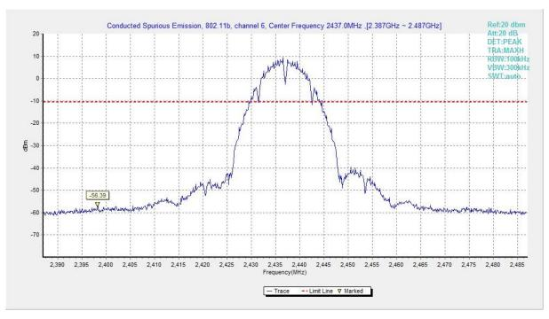
Fig.A.6.1.111 Transmitter Spurious Emission - Conducted (802.11b, Ch6, Center Frequency)
