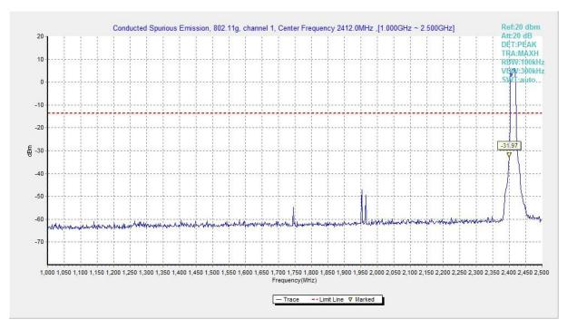
Fig.A.6.1.129 Transmitter Spurious Emission - Conducted (802.11g, Ch1, 1 GHz-2.5 GHz)
