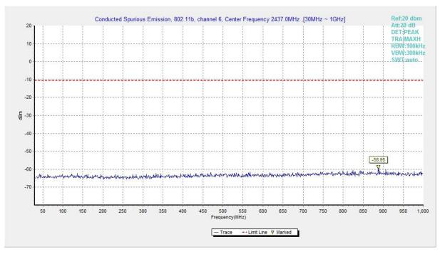
Fig.A.6.1.112 Transmitter Spurious Emission - Conducted (802.11b, Ch6, 30 MHz-1 GHz)
