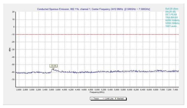
Fig.A.6.1.106 Transmitter Spurious Emission - Conducted (802.11b, Ch1, 2.5 GHz-7.5 GHz)
