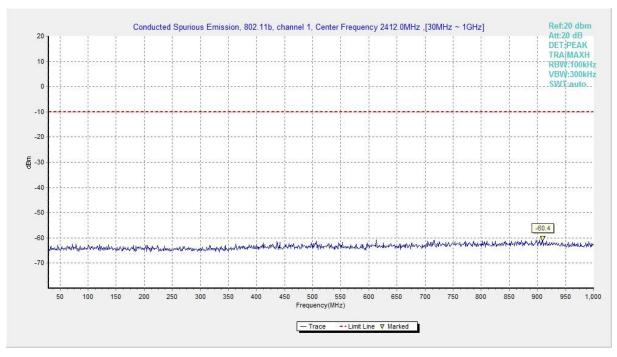
Fig.A.6.1.104 Transmitter Spurious Emission - Conducted (802.11b, Ch1, 30 MHz-1 GHz)
