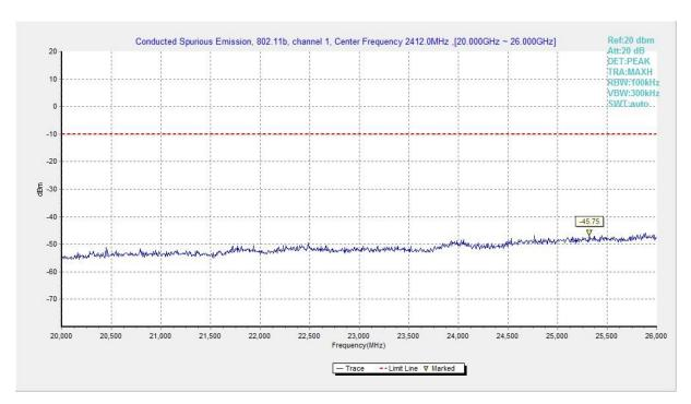
Fig.A.6.1.110 Transmitter Spurious Emission - Conducted (802.11b, Ch1, 20 GHz-26 GHz)
