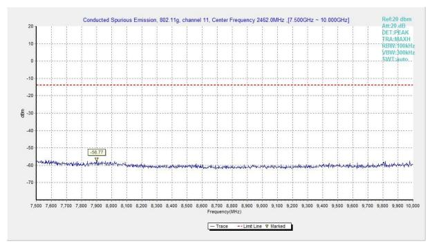
Fig.A.6.1.147 Transmitter Spurious Emission - Conducted (802.11g, Ch11, 7.5 GHz-10 GHz)
