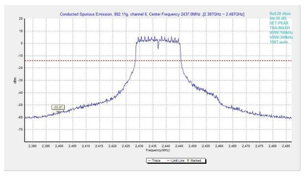
Fig.A.6.1.135 Transmitter Spurious Emission - Conducted (802.11g, Ch6, Center Frequency)
