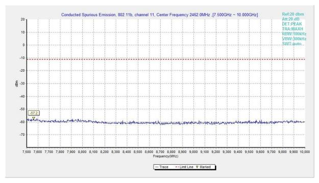
Fig.A.6.1.123 Transmitter Spurious Emission - Conducted (802.11b, Ch11, 7.5 GHz-10 GHz)
