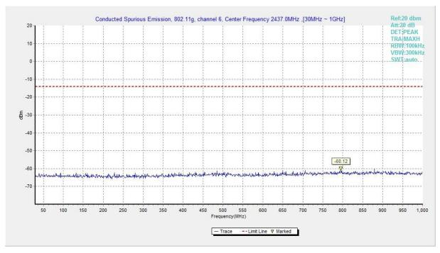
Fig.A.6.1.136 Transmitter Spurious Emission - Conducted (802.11g, Ch6, 30 MHz-1 GHz)
