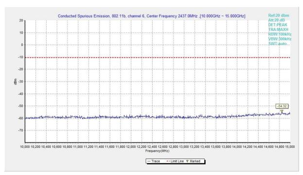
Fig.A.6.1.116 Transmitter Spurious Emission - Conducted (802.11b, Ch6, 10 GHz-15 GHz)
