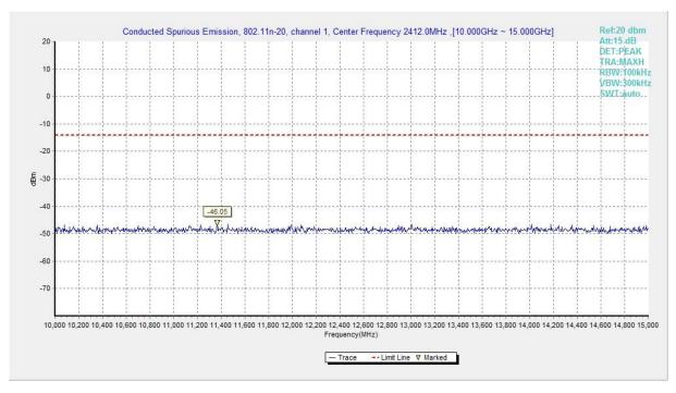
Fig.A.6.1.156 Transmitter Spurious Emission - Conducted (802.11n-HT20, Ch1, 10 GHz-15 GHz)
