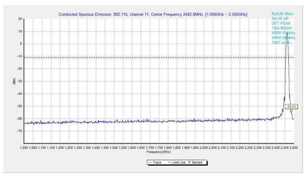
Fig.A.6.1.121 Transmitter Spurious Emission - Conducted (802.11b, Ch11, 1 GHz-2.5 GHz)
