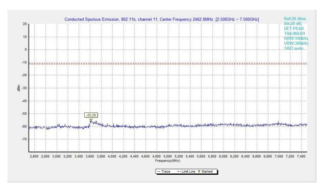
Fig.A.6.1.122 Transmitter Spurious Emission - Conducted (802.11b, Ch11, 2.5 GHz-7.5 GHz)
