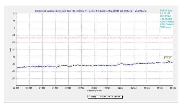
Fig.A.6.1.150 Transmitter Spurious Emission - Conducted (802.11g, Ch11, 20 GHz-26 GHz)
