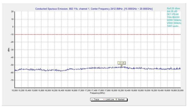
Fig.A.6.1.109 Transmitter Spurious Emission - Conducted (802.11b, Ch1, 15 GHz-20 GHz)
