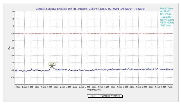
Fig.A.6.1.114 Transmitter Spurious Emission - Conducted (802.11b, Ch6, 2.5 GHz-7.5 GHz)
