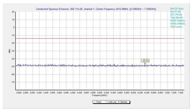
Fig.A.6.1.154 Transmitter Spurious Emission - Conducted (802.11n-HT20, Ch1, 2.5 GHz-7.5 GHz)
