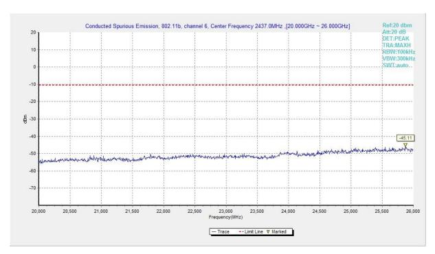
Fig.A.6.1.118 Transmitter Spurious Emission - Conducted (802.11b, Ch6, 20 GHz-26 GHz)
