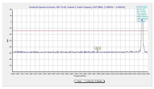
Fig.A.6.1.161 Transmitter Spurious Emission - Conducted (802.11n-HT20, Ch6, 1 GHz-2.5 GHz)
