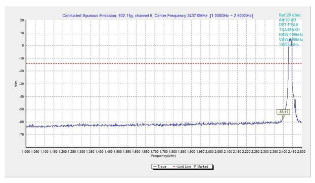
Fig.A.6.1.137 Transmitter Spurious Emission - Conducted (802.11g, Ch6, 1 GHz-2.5 GHz)
