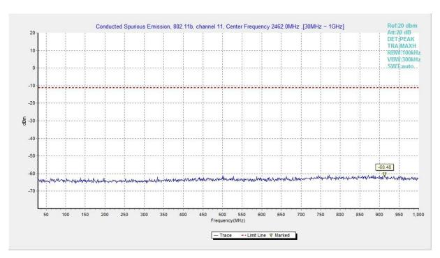
Fig.A.6.1.120 Transmitter Spurious Emission - Conducted (802.11b, Ch11, 30 MHz-1 GHz)
