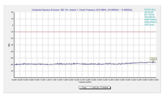
Fig.A.6.1.108 Transmitter Spurious Emission - Conducted (802.11b, Ch1, 10 GHz-15 GHz)
