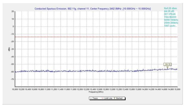
Fig.A.6.1.148 Transmitter Spurious Emission - Conducted (802.11g, Ch11, 10 GHz-15 GHz)
