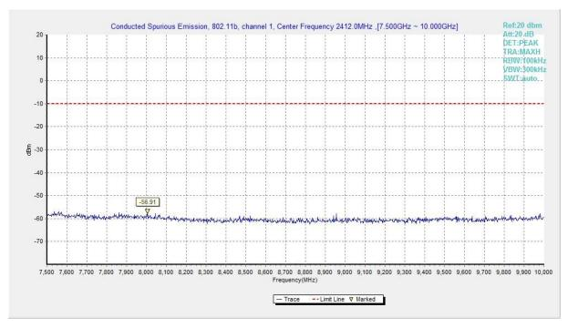
Fig.A.6.1.107 Transmitter Spurious Emission - Conducted (802.11b, Ch1, 7.5 GHz-10 GHz)
