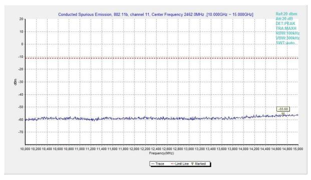
Fig.A.6.1.124 Transmitter Spurious Emission - Conducted (802.11b, Ch11, 10 GHz-15 GHz)
