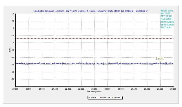
Fig.A.6.1.158 Transmitter Spurious Emission - Conducted (802.11n-HT20, Ch1, 20 GHz-26 GHz)
