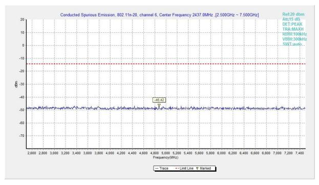
Fig.A.6.1.162 Transmitter Spurious Emission - Conducted (802.11n-HT20, Ch6, 2.5 GHz-7.5 GHz)
