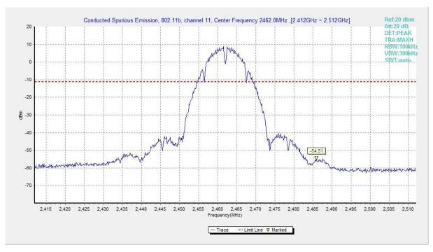
Fig.A.6.1.119 Transmitter Spurious Emission - Conducted (802.11b, Ch11, Center Frequency)
