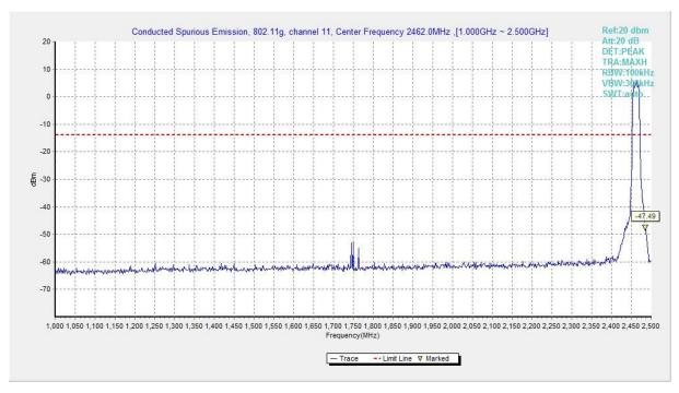
Fig.A.6.1.145 Transmitter Spurious Emission - Conducted (802.11g, Ch11, 1 GHz-2.5 GHz)
