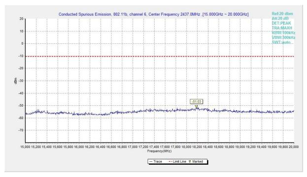
Fig.A.6.1.117 Transmitter Spurious Emission - Conducted (802.11b, Ch6, 15 GHz-20 GHz)
