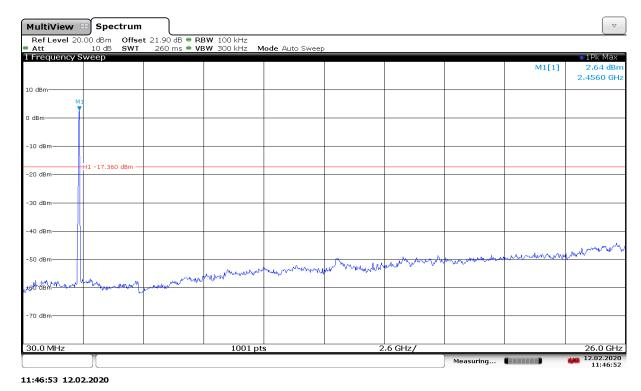
Fig.A.6.1.101 Transmitter Spurious Emission - Conducted (802.11ax-HE40-RU242-right, Ch6, 30 MHz-26 GHz)
