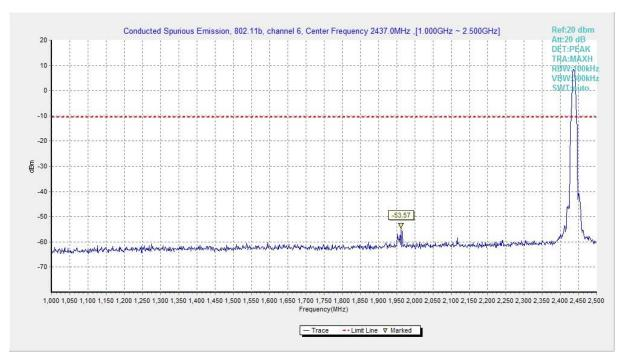
Fig.A.6.1.113 Transmitter Spurious Emission - Conducted (802.11b, Ch6, 1 GHz-2.5 GHz)
