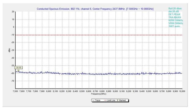
Fig.A.6.1.115 Transmitter Spurious Emission - Conducted (802.11b, Ch6, 7.5 GHz-10 GHz)
