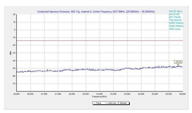
Fig.A.6.1.142 Transmitter Spurious Emission - Conducted (802.11g, Ch6, 20 GHz-26 GHz)
