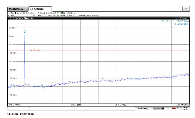
Fig.A.6.1.102 Transmitter Spurious Emission - Conducted (802.11ax-HE40-RU242-right, Ch9, 30 MHz-26 GHz)
