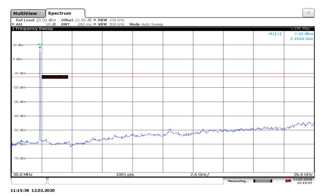
Fig.A.6.1.99 Transmitter Spurious Emission - Conducted (802.11ax-HE20-RU52-middle, Ch11, 30 MHz-26 GHz)
