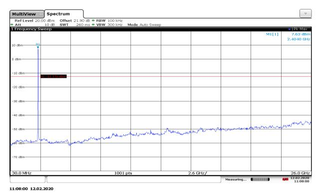
Fig.A.6.1.97 Transmitter Spurious Emission - Conducted (802.11ax-HE20-RU52-middle, Ch1, 30 MHz-26 GHz)
