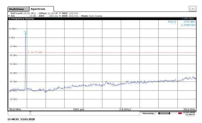
Fig.A.6.1.100 Transmitter Spurious Emission - Conducted (802.11ax-HE40-RU242-right, Ch3, 30 MHz-26 GHz)
