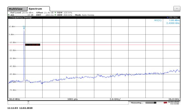
Fig.A.6.1.98 Transmitter Spurious Emission - Conducted (802.11ax-HE20-RU52-middle, Ch6, 30 MHz-26 GHz)
