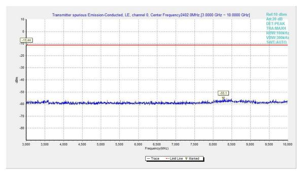
Fig.14. Transmitter Spurious Emission - Conducted: GFSK, 2402 MHz,3GHz - 10GHz
