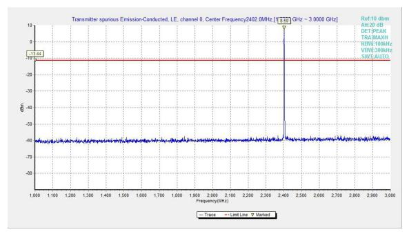
Fig.13. Transmitter Spurious Emission - Conducted: GFSK, 2402 MHz,1GHz - 3GHz
