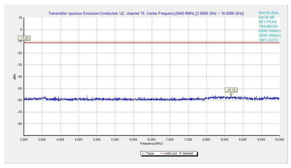
Fig.19. Transmitter Spurious Emission - Conducted: GFSK, 2440 MHz, 3GHz - 10GHz
