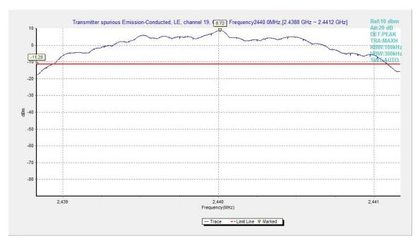
Fig.16. Transmitter Spurious Emission - Conducted: GFSK, 2440MHz
