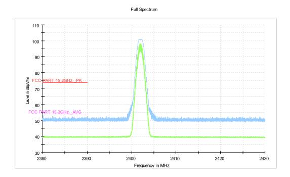
Fig.7. Frequency Band Edges: EUT4 ANT4 BLE 4.0 GFSK, 2402 MHz, Hopping Off, 2.38 GHz – 2.45GHz
