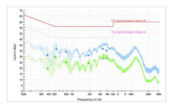
Fig.A.9.2 AC Powerline Conducted Emission-Idle EUT5(M2001J2G)+AE11+AE13+AE16
