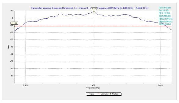
Fig.11. Transmitter Spurious Emission - Conducted: GFSK,2402MHz
