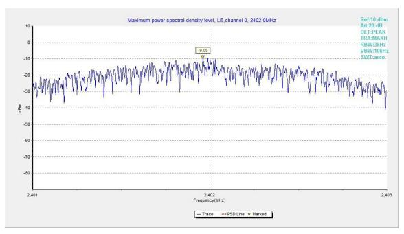
Fig.29. Maximum Power Spectral Density Level Function: GFSK, 2402 MHz
