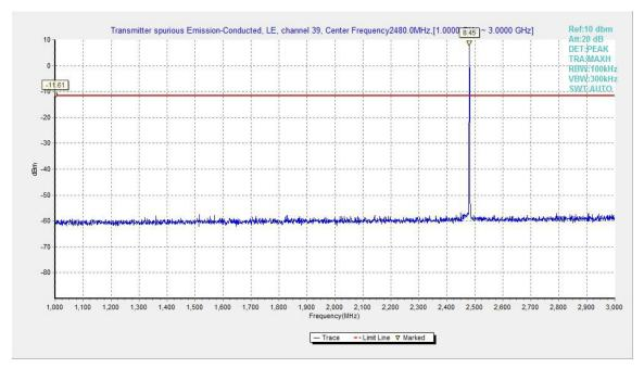
Fig.23. Transmitter Spurious Emission - Conducted: GFSK, 2480 MHz, 1GHz - 3GHz
