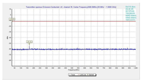
Fig.22. Transmitter Spurious Emission - Conducted: GFSK, 2480 MHz, 30MHz - 1GHz
