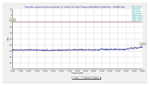
Fig.25. Transmitter Spurious Emission - Conducted: GFSK, 2480 MHz, 10GHz - 26GHz
