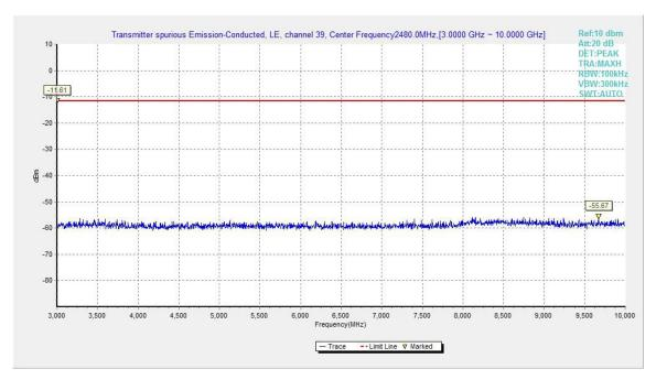
Fig.24. Transmitter Spurious Emission - Conducted: GFSK, 2480 MHz, 3GHz - 10GHz
