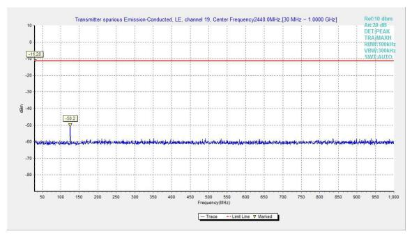
Fig.17. Transmitter Spurious Emission - Conducted: GFSK, 2440 MHz, 30MHz - 1GHz
