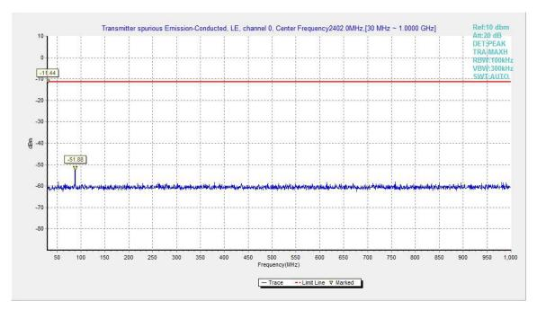
Fig.12. Transmitter Spurious Emission - Conducted: GFSK, 2402 MHz, 30MHz - 1GHz
