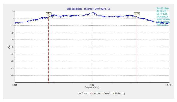
Fig.26. 6dB Bandwidth: GFSK, 2402 MHz
