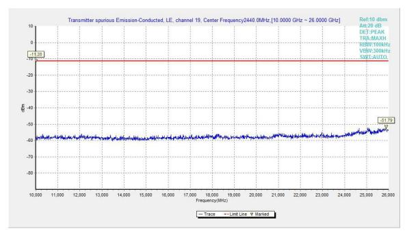
Fig.20. Transmitter Spurious Emission - Conducted: GFSK, 2440 MHz, 10GHz – 26GHz
