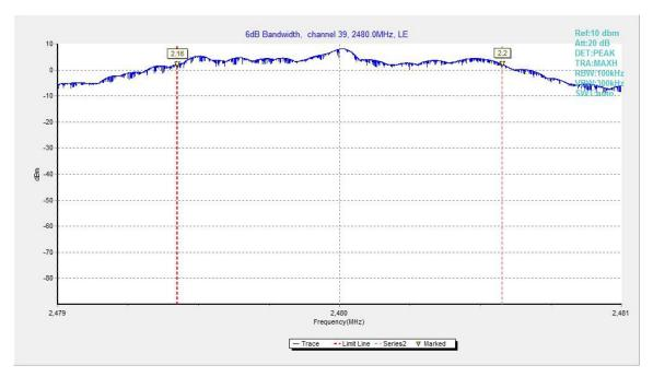
Fig.28. 6dB Bandwidth: GFSK, 2480 MHz
