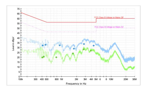
Fig.A.9.1 AC Powerline Conducted Emission- Bluetooth EUT5(M2001J2G)+AE11+AE13+AE16
