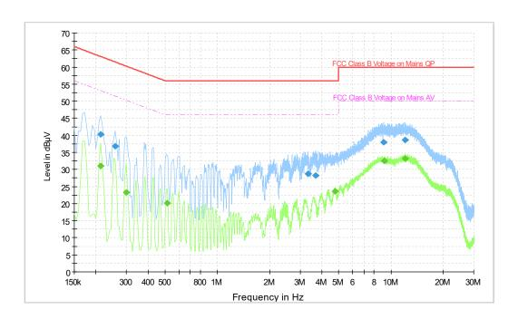
Fig.A.9.1 AC Powerline Conducted Emission- Bluetooth EUT3(M2001J2G)+AE1+AE3+AE6
