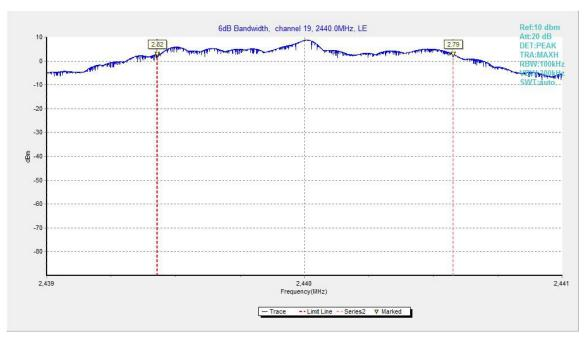
Fig.27. 6dB Bandwidth: GFSK, 2440 MHz
