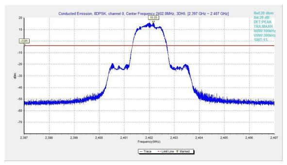
Fig.64. Conducted spurious emission: 8DPSK, Channel 0,2402MHz
