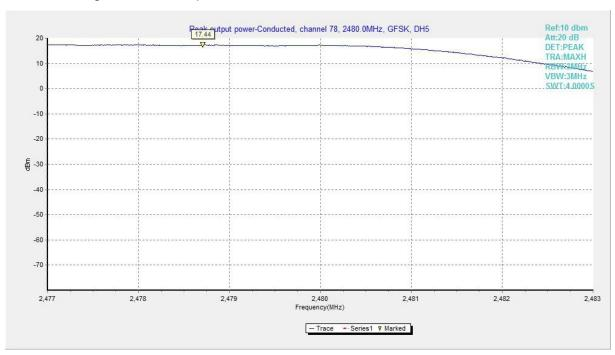
Fig.3. Peak Output Power -Conducted: Antenna 3, GFSK, Channel 78,
