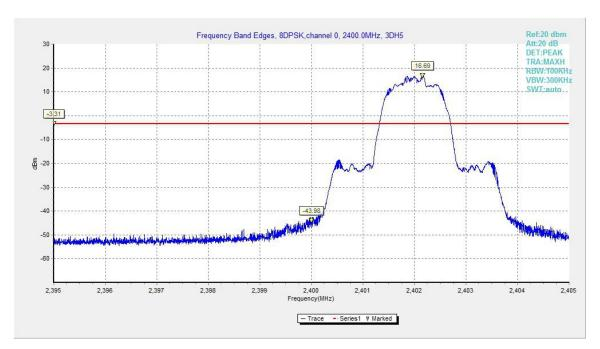
Fig.18. Frequency Band Edges: 8DPSK, Channel 0, Hopping Off
