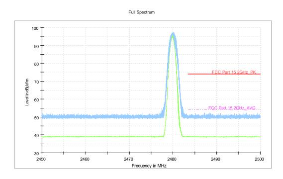
Fig.31. Frequency Band Edges: EUT4 ANT4  $\pi$ /4 DQPSK, Channel 78, Hopping Off, 2.38 GHz - 2.45GHz
