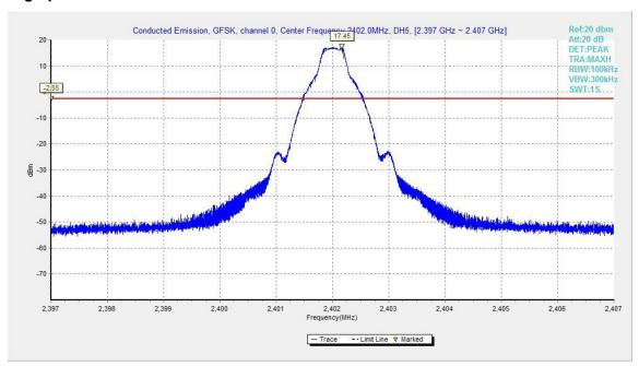
Fig.34. Conducted spurious emission: GFSK, Channel 0,2402MHz
