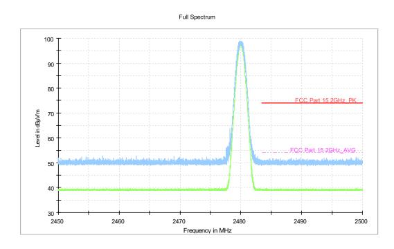
Fig.29. Frequency Band Edges: EUT4 ANT4 GFSK, Channel 78, Hopping Off, ch11, 2.45 GHz - 2.50GHz
