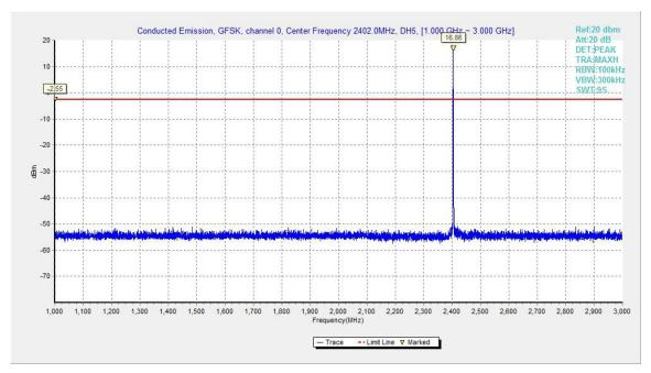
Fig.36. Conducted spurious emission: GFSK, Channel 0, 1GHz - 3GHz
