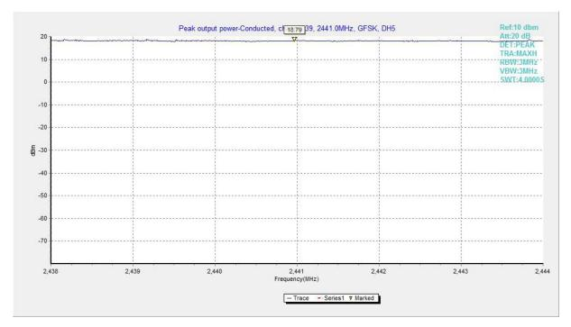
Fig.2. Peak Output Power -Conducted: Antenna 3, GFSK, Channel 39,
