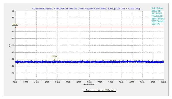
Fig.57. Conducted spurious emission:  $\pi/4$  DQPSK, Channel 39, 3GHz - 10GHz
