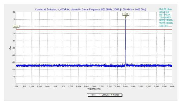
Fig.51. Conducted spurious emission: π/4 DQPSK, Channel 0, 1GHz - 3GHz
