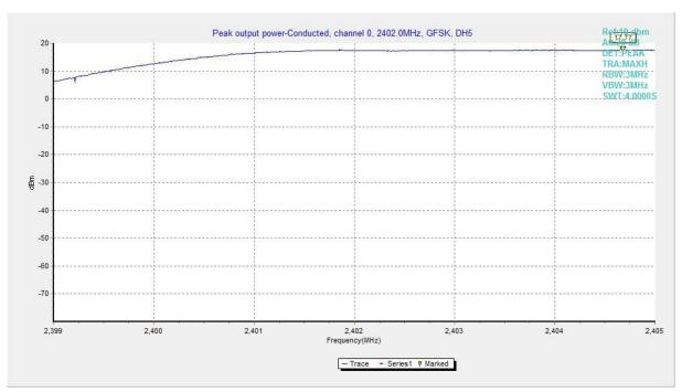
Fig.1. Peak Output Power -Conducted: Antenna 3, GFSK, Channel 0,
