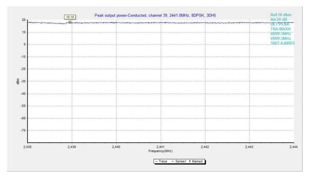
Fig.8. Peak Output Power -Conducted: Antenna 3, 8DPSK, Channel 39,
