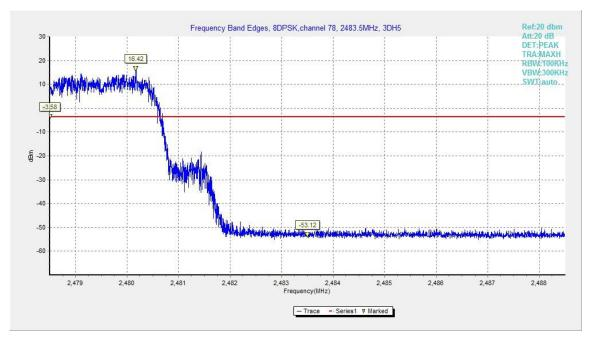
Fig.21. Frequency Band Edges: 8DPSK, Channel 78, Hopping On
