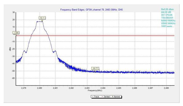
Fig.12. Frequency Band Edges: GFSK, Channel 78, Hopping Off
