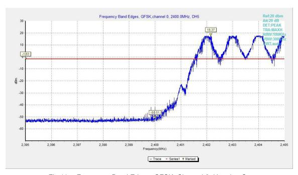
Fig.11. Frequency Band Edges: GFSK, Channel 0, Hopping On
