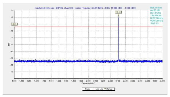
Fig.66. Conducted spurious emission: 8DPSK, Channel 0, 1GHz - 3GHz
