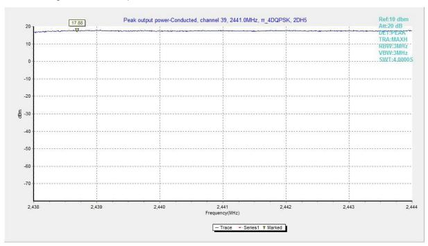
Fig.5. Peak Output Power -Conducted: Antenna 3, π/4 DQPSK, Channel 39,
