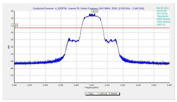
Fig.54. Conducted spurious emission:  $\pi/4$  DQPSK, Channel 39, 2441MHz
