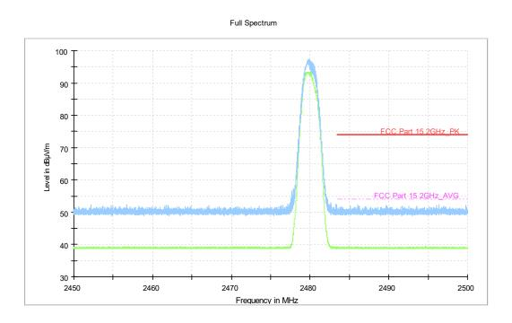
Fig.33. Frequency Band Edges: EUT4 ANT4 8DPSK, Channel 78, 2.38 GHz - 2.45GHz
