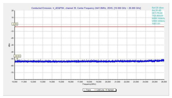
Fig.58. Conducted spurious emission: π/4 DQPSK, Channel 39, 10GHz – 26GHz
