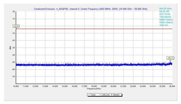
Fig.53. Conducted spurious emission: π/4 DQPSK, Channel 0,10GHz - 26GHz
