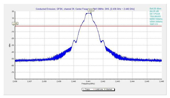
Fig.39. Conducted spurious emission: GFSK, Channel 39, 2441MHz
