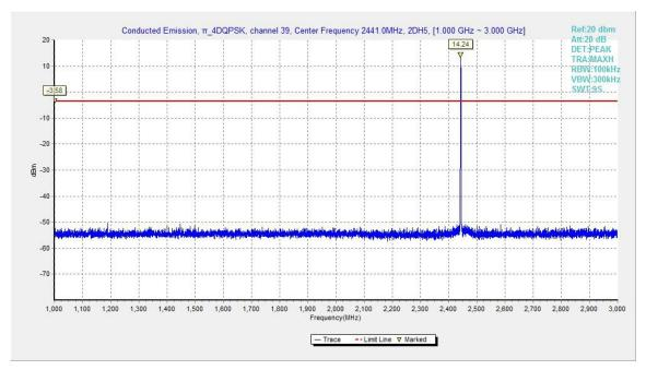
Fig.56. Conducted spurious emission:  $\pi/4$  DQPSK, Channel 39, 1GHz - 3GHz
