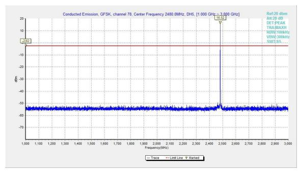
Fig.46. Conducted spurious emission: GFSK, Channel 78, 1GHz - 3GHz
