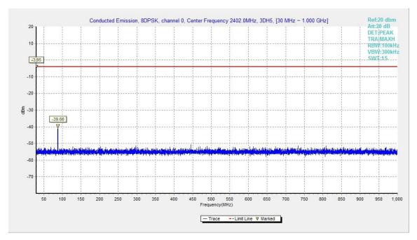
Fig.65. Conducted spurious emission: 8DPSK, Channel 0, 30MHz - 1GHz
