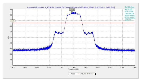
Fig.59. Conducted spurious emission:  $\pi/4$  DQPSK, Channel 78, 2480MHz
