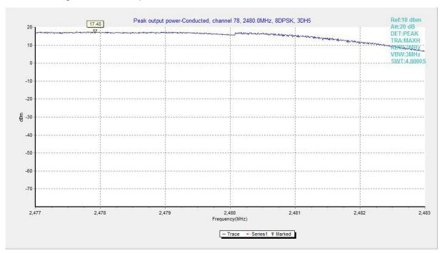
Fig.9. Peak Output Power -Conducted: Antenna 3, 8DPSK, Channel 78,
