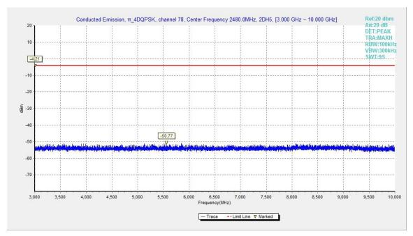
Fig.62. Conducted spurious emission: π/4 DQPSK, Channel 78, 3GHz - 10GHz
