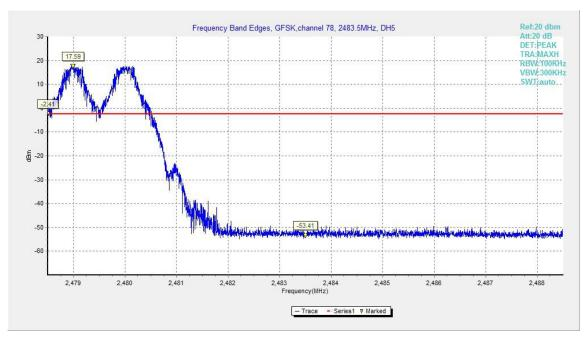
Fig.13. Frequency Band Edges: GFSK, Channel 78, Hopping On
