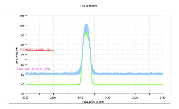
Fig.32. Frequency Band Edges: EUT4 ANT4 DPSK, Channel 0, 2.38 GHz - 2.45GHz
