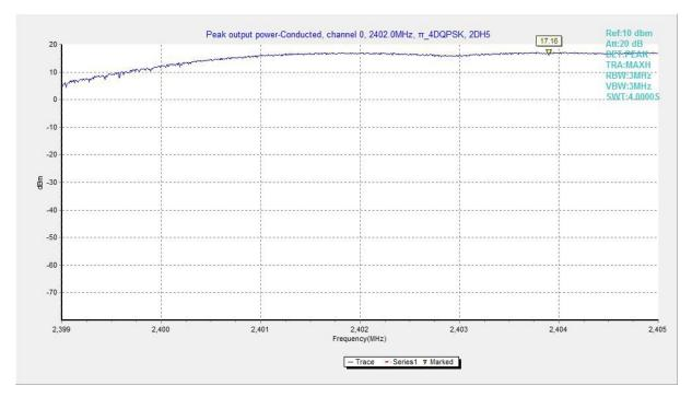
Fig.4. Peak Output Power -Conducted: Antenna 3, π/4 DQPSK, Channel 0,
