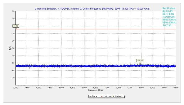
Fig.52. Conducted spurious emission:  $\pi/4$  DQPSK, Channel 0, 3GHz - 10GHz
