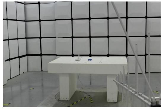
**1.3** Setup for Unwanted Emissions that fall Outside of the Restricted Bands(Radiated) and Unwanted Emissions in the Restricted Bands (Radiated) above 1GHz
