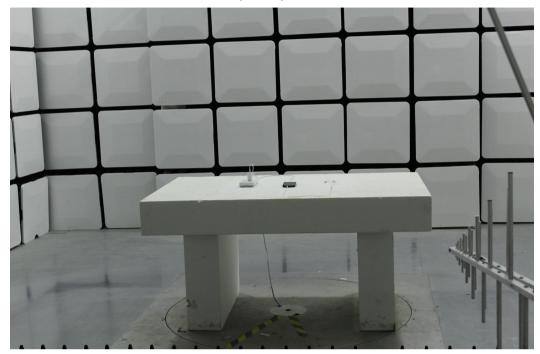
1.3 Setup for Unwanted Emissions that fall Outside of the Restricted Bands(Radiated) and Unwanted Emissions in the Restricted Bands (Radiated) above 1GHz (Test Location: SGS-CSTC STANDARDS TECHNICAL SERVICES (XI 'AN) CO., LTD.)
