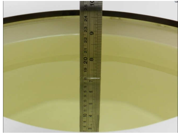
Fig 11.1.2 Photo of Liquid Height for Body SAR
