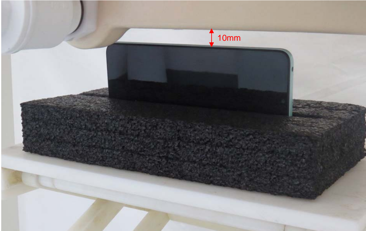
Picture 7: Left Edge, the distance from handset to the bottom of the Phantom is 10mm
