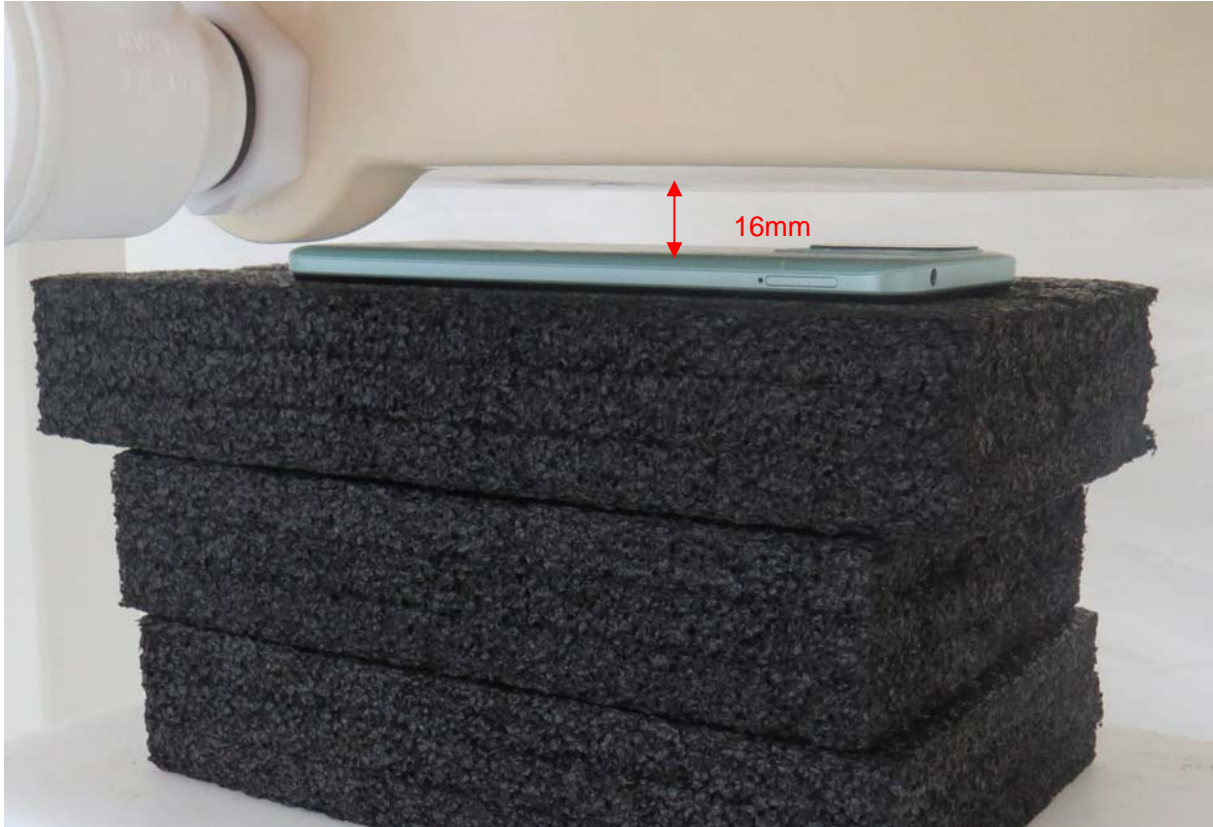
Picture 17: Back Side, the distance from handset to the bottom of the Phantom is 16mm
