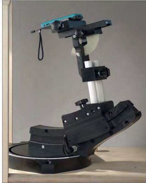
F-2. Device Holder for Transmitters
