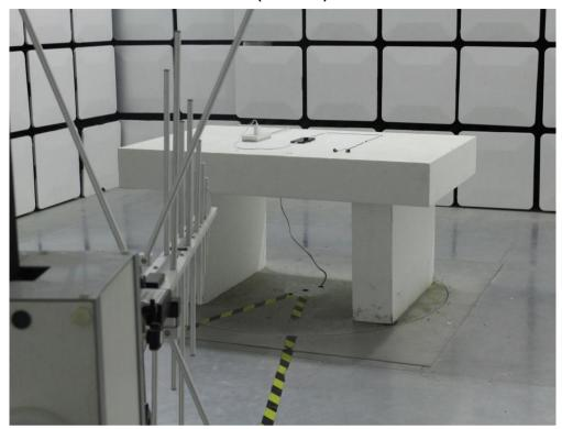
1.3 Setup for Unwanted Emissions that fall Outside of the Restricted Bands(Radiated) and Unwanted Emissions in the Restricted Bands (Radiated) above 1GHz
