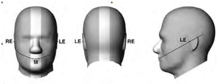
F-3. Front, back, and side views of SAM (model for the phantom shell). Full-head model is for illustration purposes only—procedures in this recommended practice are intended primarily for the phantom setup.
