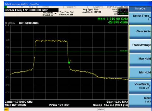
LTE Band 2 5MHz QPSK 1RB CH-High
