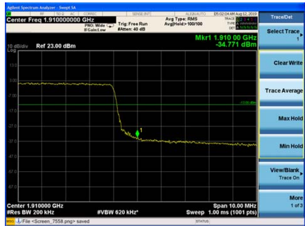
LTE Band 2 1.4MHz 64QAM 1RB CH-High
