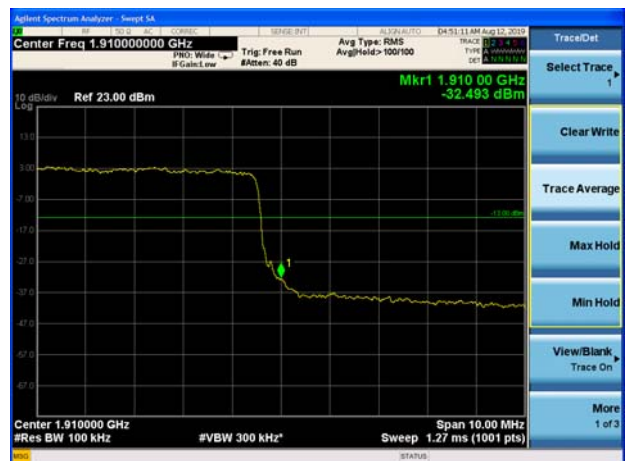
LTE Band 2 10MHz QPSK 100%RB CH-High
