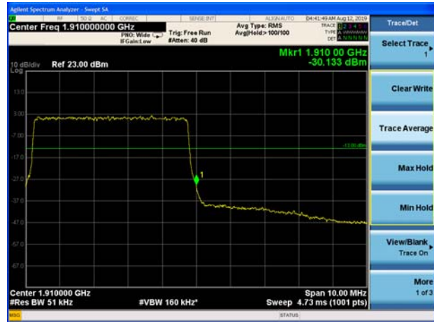
LTE Band 2 10MHz 16QAM 1RB CH-High
