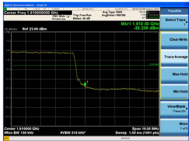
LTE Band 2 20MHz 16QAM 1RB CH-High
