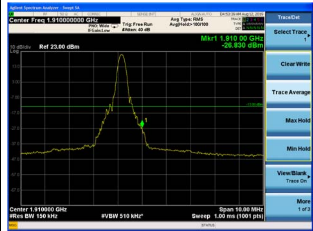
LTE Band 2 15MHz QPSK 100%RB CH-High
