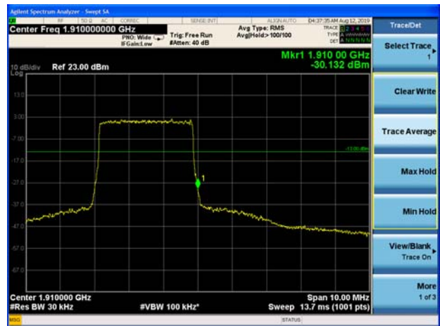
LTE Band 2 5MHz 16QAM 1RB CH-High
