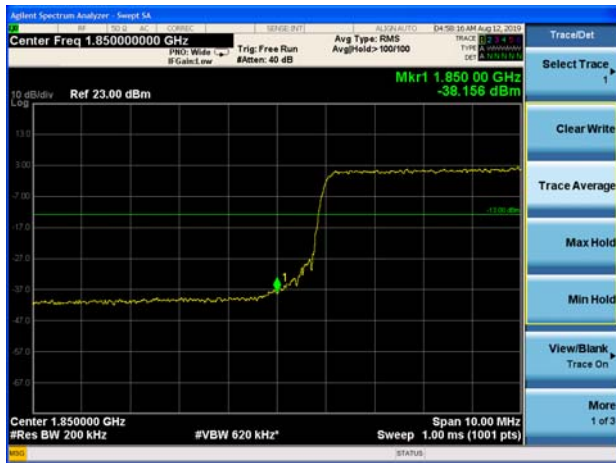
LTE Band 2 1.4MHz 64QAM 1RB CH-Low
