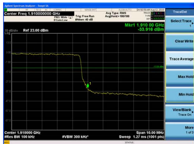
LTE Band 2 10MHz 16QAM 100%RB CH-High
