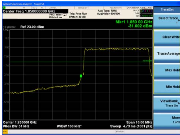
LTE Band 2 10MHz 64QAM 1RB CH-Low
