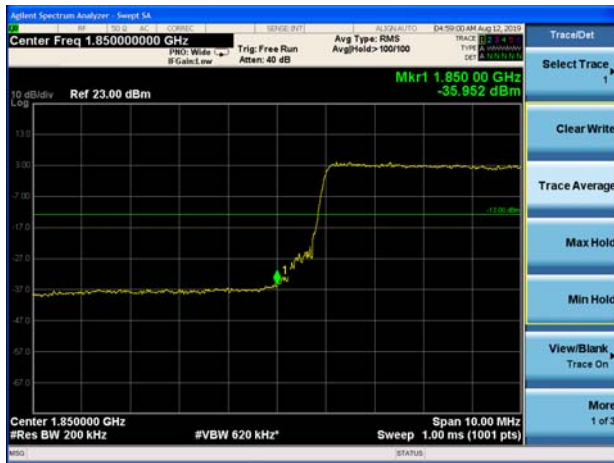
LTE Band 2 1.4MHz 16QAM 1RB CH-Low
