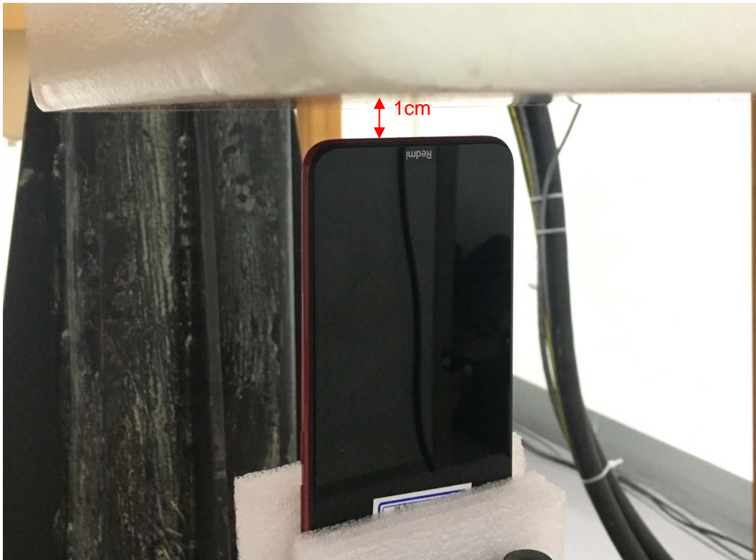
Picture 11: Bottom Side, the distance from handset to the bottom of the Phantom is 1.0cm
