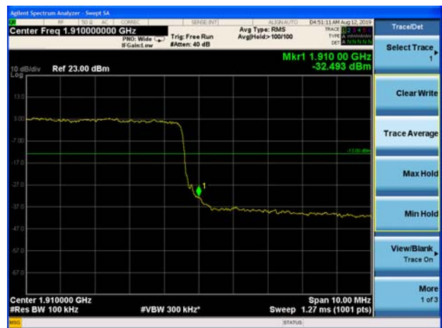
LTE Band 2 10MHz QPSK 100%RB CH-High
