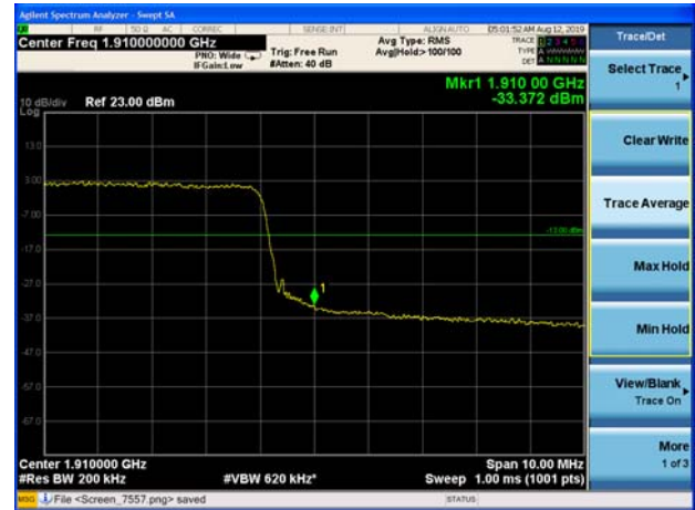
LTE Band 2 1.4MHz 16QAM 1RB CH-High
