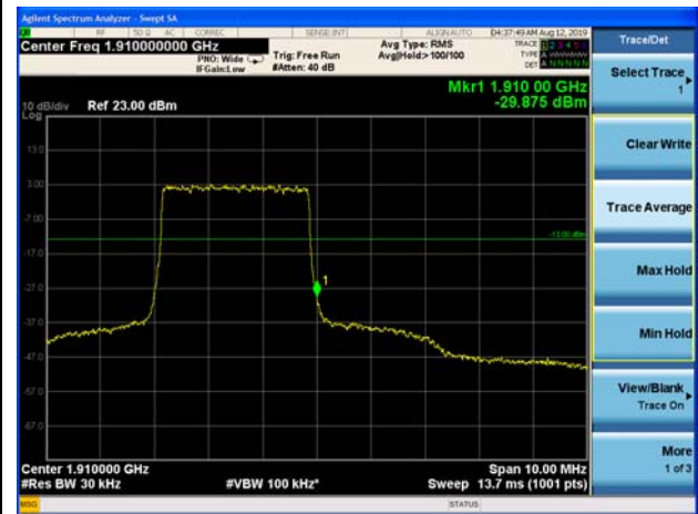
LTE Band 2 5MHz QPSK 1RB CH-High
