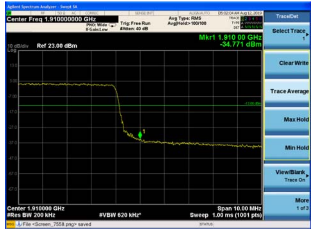
LTE Band 2 1.4MHz 64QAM 1RB CH-High
