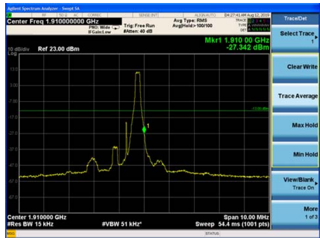
LTE Band 2 1.4MHz 64QAM 100%RB CH-High
