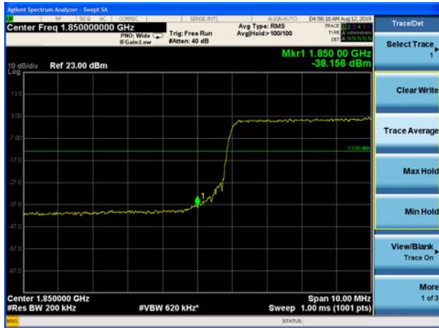
LTE Band 2 1.4MHz 64QAM 1RB CH-Low
