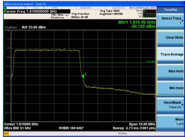
LTE Band 2 10MHz 16QAM 1RB CH-High
