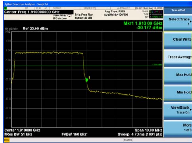
LTE Band 2 10MHz 64QAM 1RB CH-High
