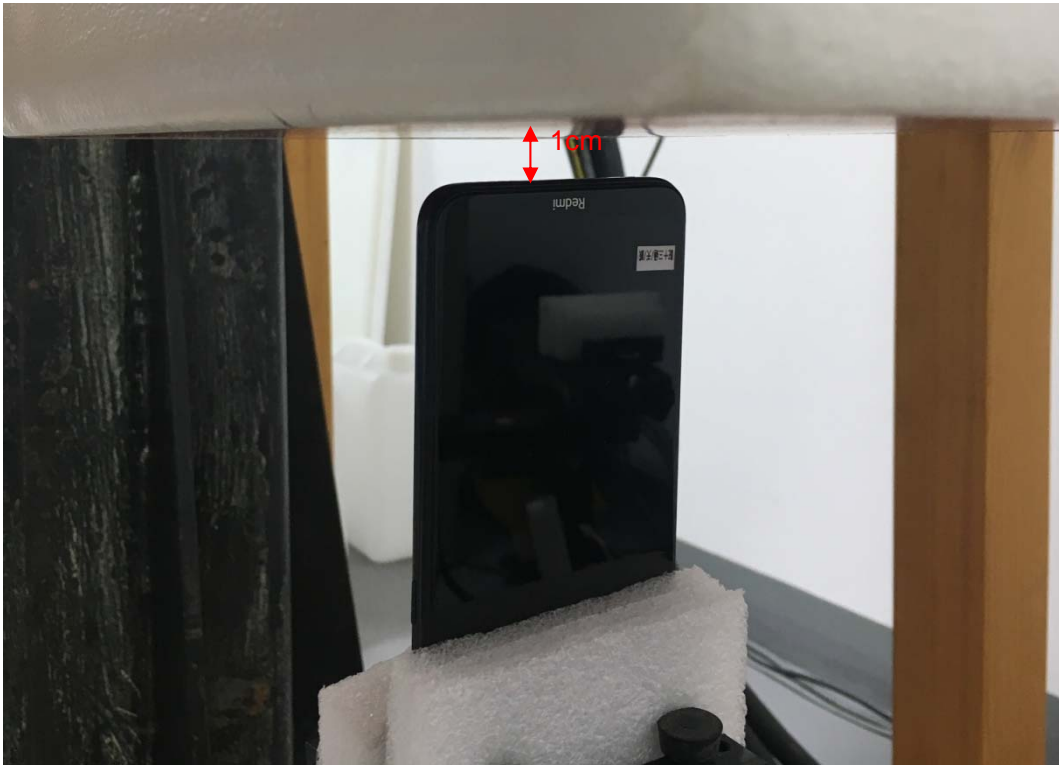
Picture 11: Bottom Side, the distance from handset to the bottom of the Phantom is 1.0cm
