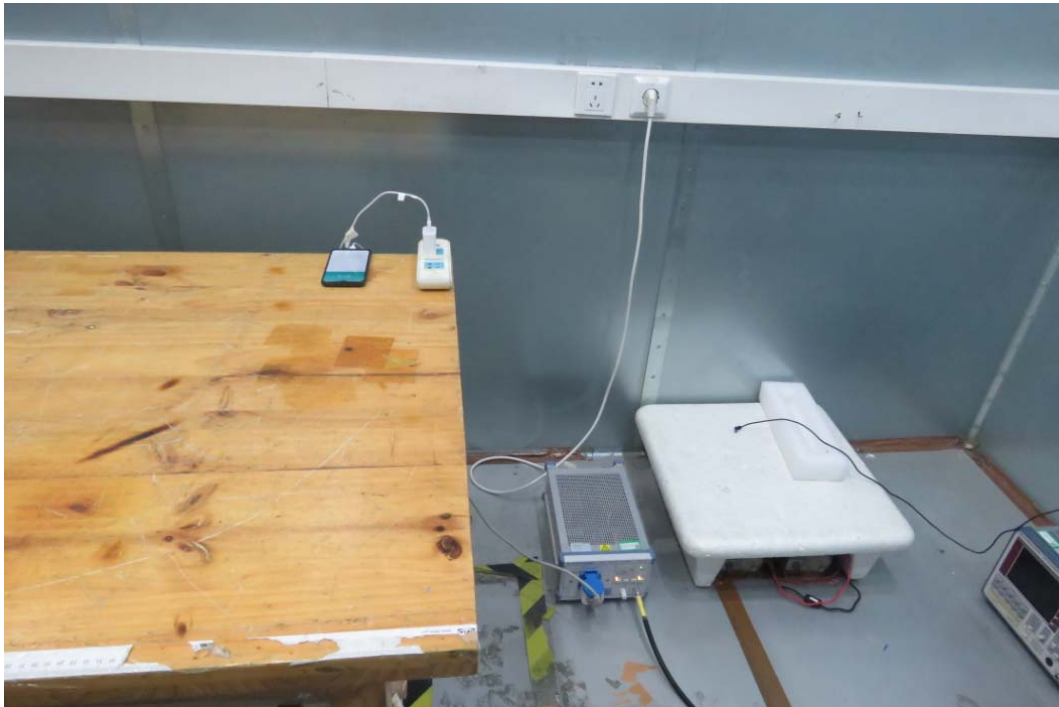
Picture 2 Conducted Emission Test Setup
