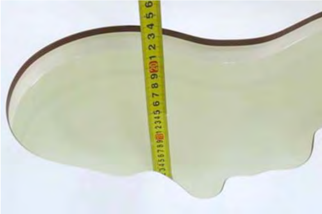
Picture 3: liquid depth in the head Phantom
