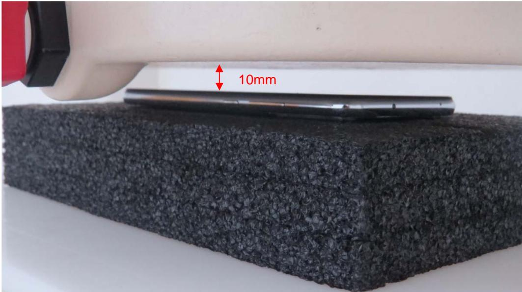
Picture 7: Front Side, the distance from handset to the bottom of the Phantom is 10mm
