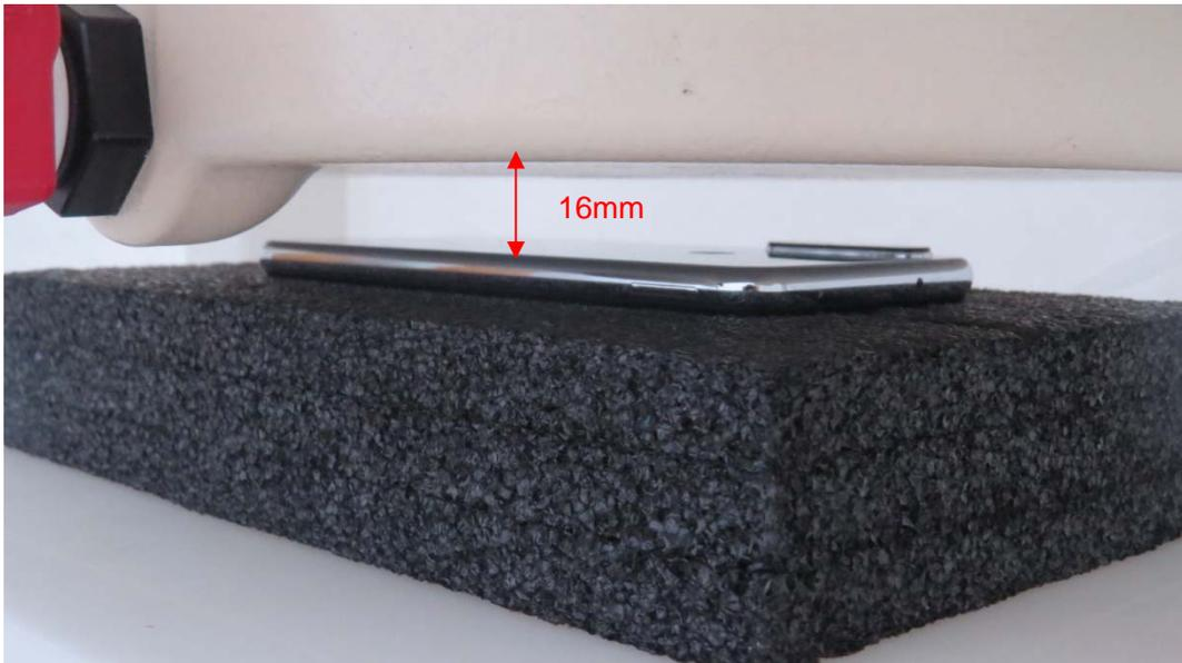
Picture 6: Back Side, the distance from handset to the bottom of the Phantom is 16mm
