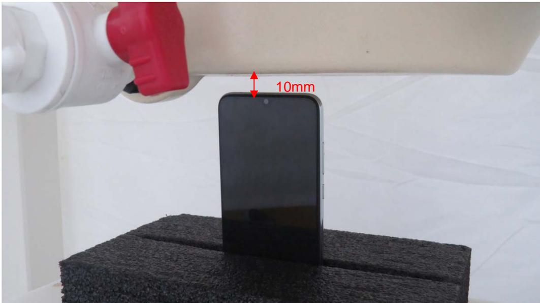
Picture 10: Top Side, the distance from handset to the bottom of the Phantom is 10mm
