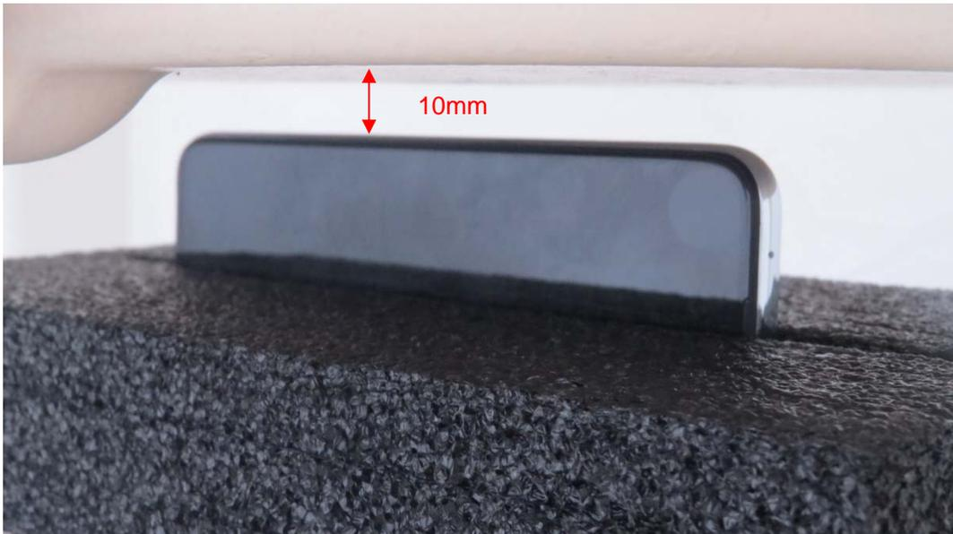
Picture 8: Left Side, the distance from handset to the bottom of the Phantom is 10mm
