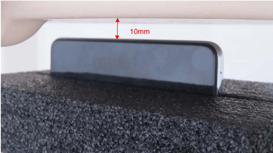
Picture 9: Right Side, the distance from handset to the bottom of the Phantom is 10mm
