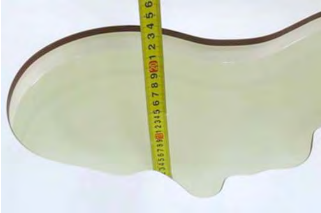
Picture 3: liquid depth in the head Phantom
