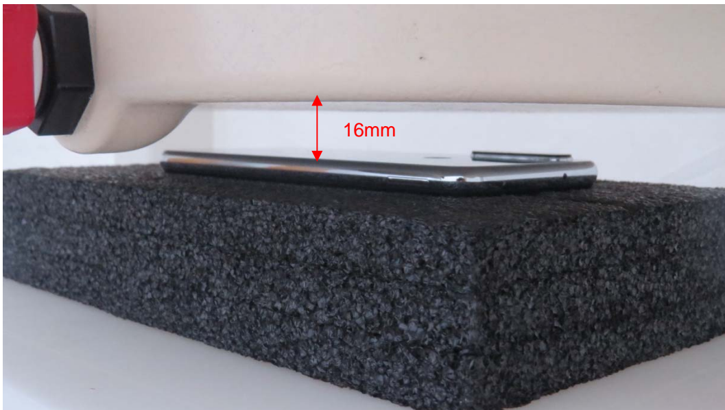
Picture 6: Back Side, the distance from handset to the bottom of the Phantom is 16mm
