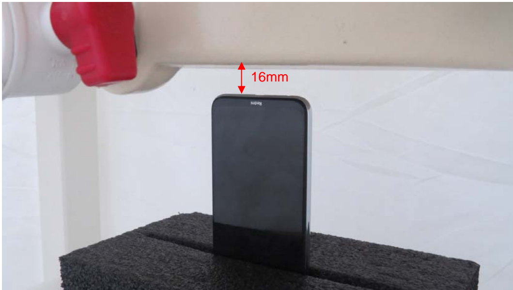
Picture 12: Bottom Side, the distance from handset to the bottom of the Phantom is 16mm
