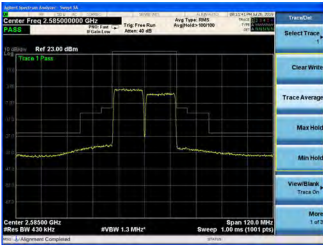
CA-38C 64QAM 15MHz+15MHz CH-Low, 1 RB
