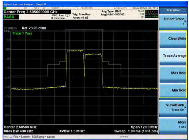
CA-38C 64QAM 15MHz+15MHz CH-High, 1 RB
