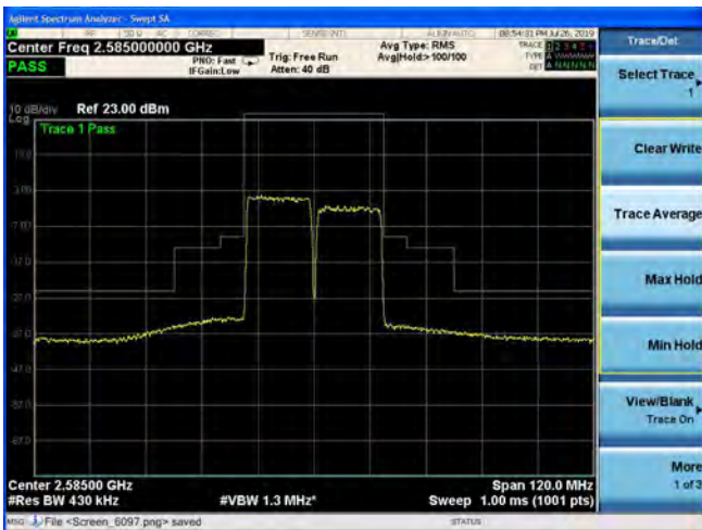
CA-38C 64QAM 15MHz+15MHz CH-Low, 100%RB
