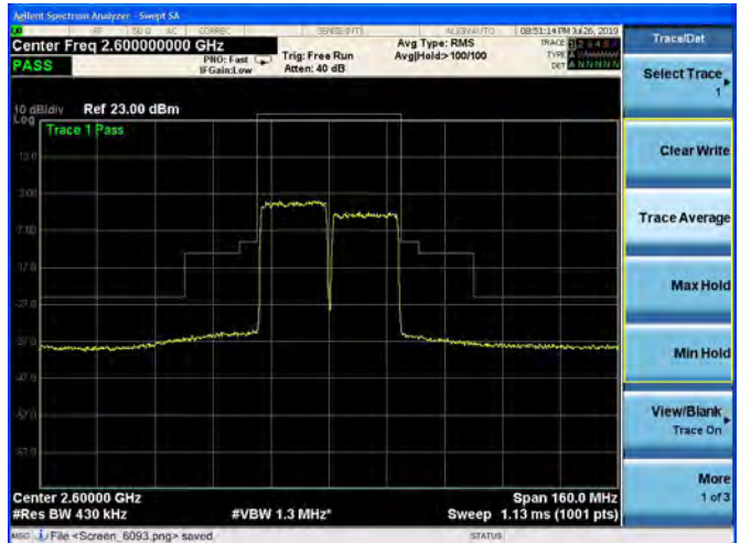
CA-38C 64QAM 20MHz+20MHz CH-High, 1 RB
