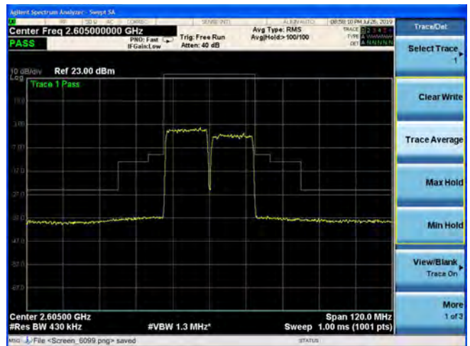
CA-38C 64QAM 15MHz+15MHz CH-High, 100%RB
