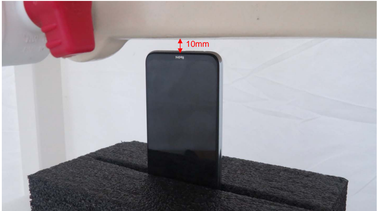
Picture 11: Bottom Side, the distance from handset to the bottom of the Phantom is 10mm
