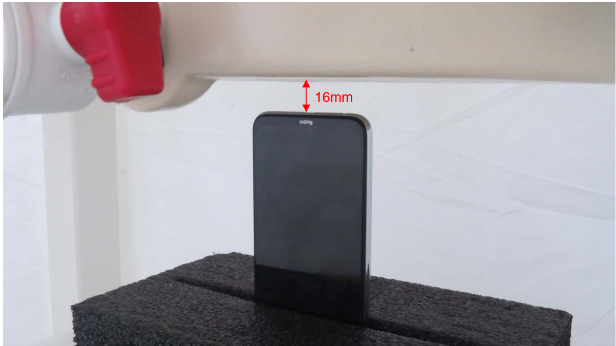
Picture 12: Bottom Side, the distance from handset to the bottom of the Phantom is 16mm
