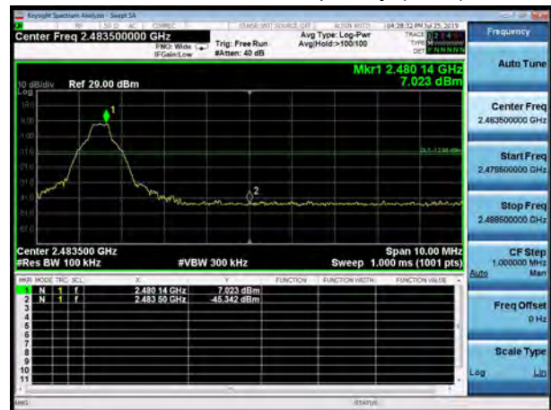
BT 2DH5 CH78, Carrier frequency (MHz): 2480
