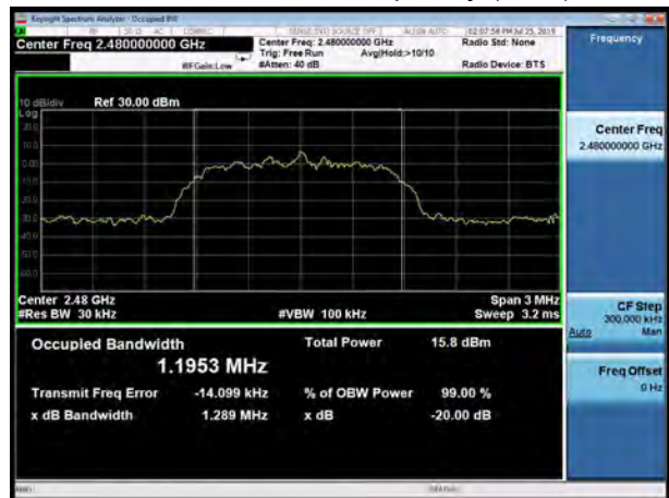
BT 2DH5 CH78, Carrier frequency (MHz): 2480
