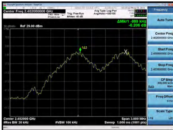
BT DH5 CH39, Carrier frequency (MHz): 2441
