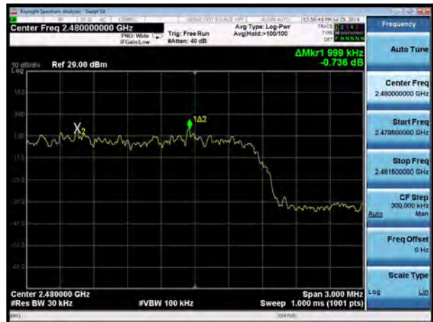
BT 2DH5 CH78, Carrier frequency (MHz): 2480
