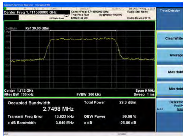
LTE Band 4 16QAM 3MHz CH-Middle
