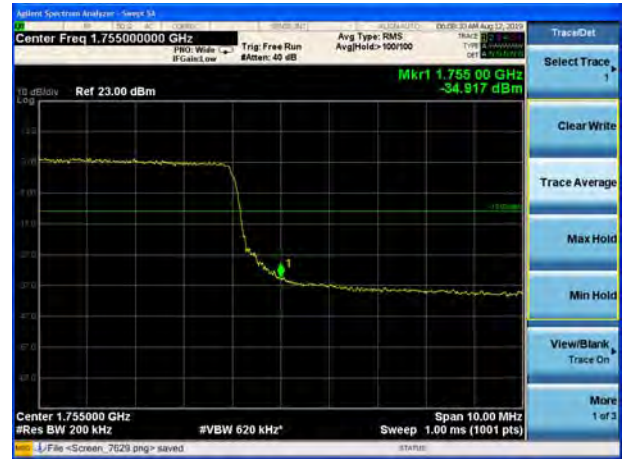
LTE Band 4 16QAM 1.4MHz CH-High, 1 RB
