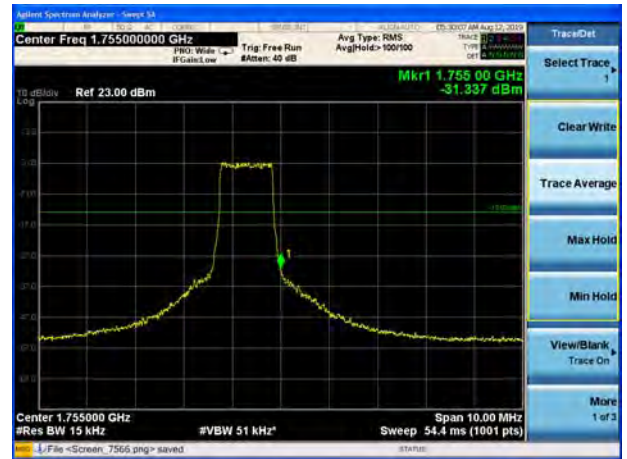
LTE Band 4 64QAM 1.4MHz CH-High, 100%RB
