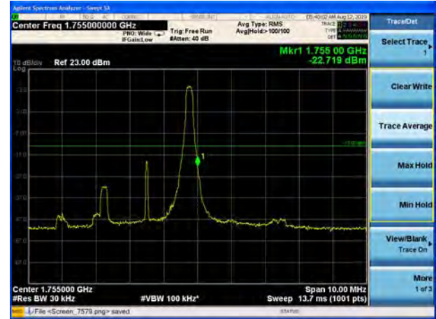
LTE Band 4 16QAM 3MHz CH-High, 100%RB
