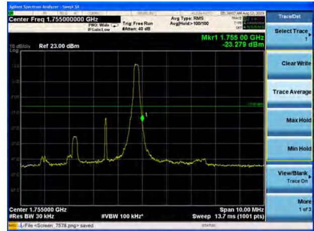
LTE Band 4 64QAM 3MHz CH-High, 100%RB
