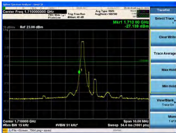
LTE Band 4 64QAM 1.4MHz CH-Low, 100%RB
