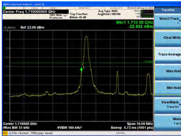
LTE Band 4 16QAM 5MHz CH-Low, 1 RB
