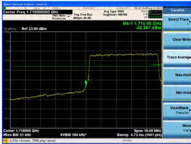
LTE Band 4 64QAM 10MHz CH-Low, 1 RB
