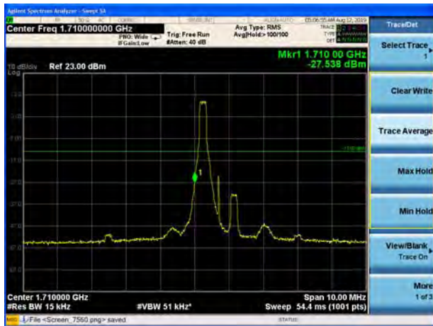
LTE Band 4 16QAM 1.4MHz CH-Low, 100%RB
