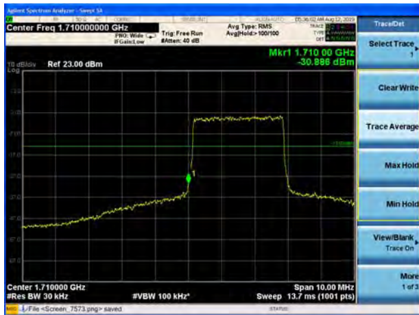
LTE Band 4 16QAM 5MHz CH-Low, 1 RB
