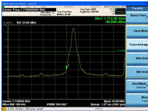
LTE Band 4 64QAM 10MHz CH-Low, 100%RB
