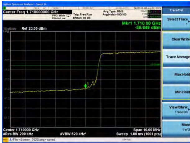
LTE Band 4 16QAM 1.4MHz CH-Low, 1 RB
