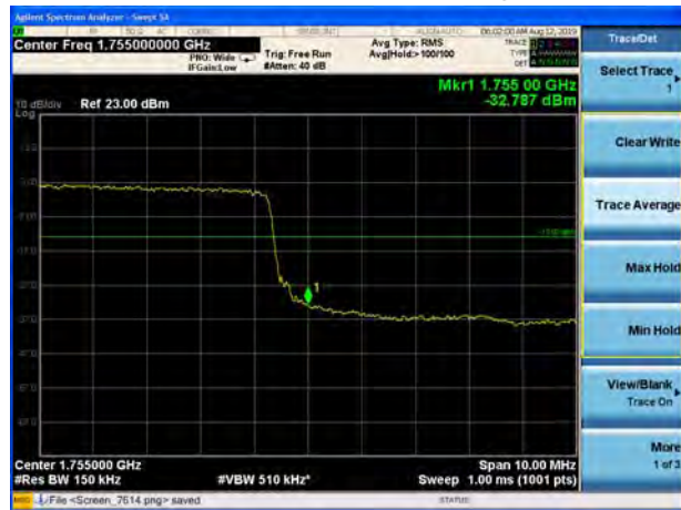
LTE Band 4 64QAM 20MHz CH-High, 1 RB
