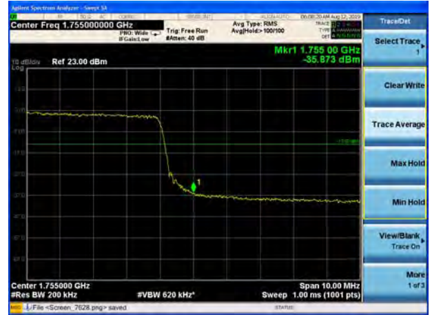
LTE Band 4 64QAM 1.4MHz CH-High, 1 RB
