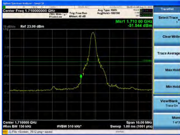
LTE Band 4 64QAM 15MHz CH-Low, 100%RB
