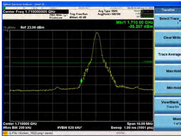
LTE Band 4 16QAM 20MHz CH-Low, 1 RB
