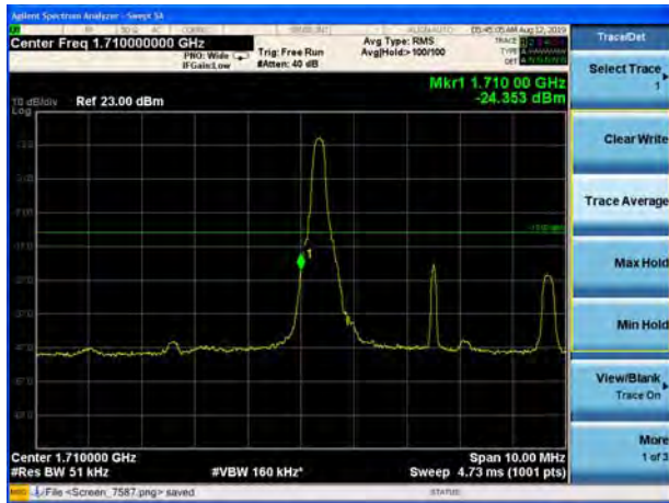
LTE Band 4 64QAM 5MHz CH-Low, 1 RB
