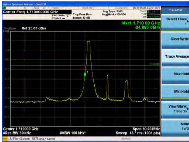
LTE Band 4 64QAM 3MHz CH-Low, 100%RB
