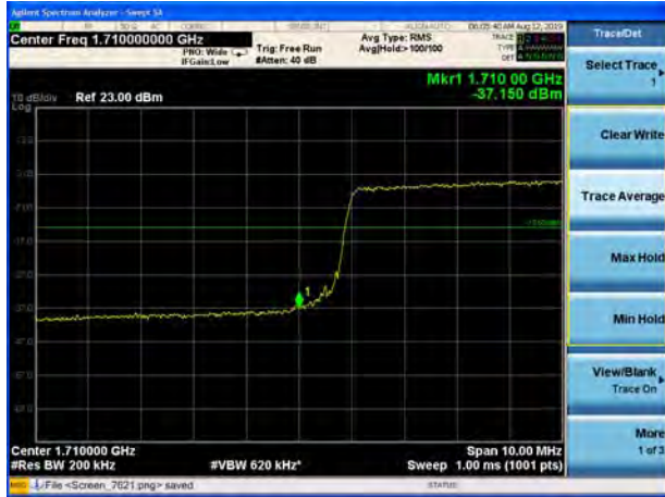
LTE Band 4 64QAM 1.4MHz CH-Low, 1 RB
