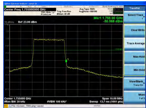
LTE Band 4 16QAM 5MHz CH-High, 1 RB
