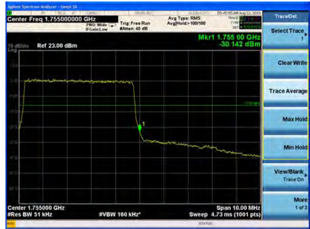
LTE Band 4 64QAM 10MHz CH-High, 1 RB
