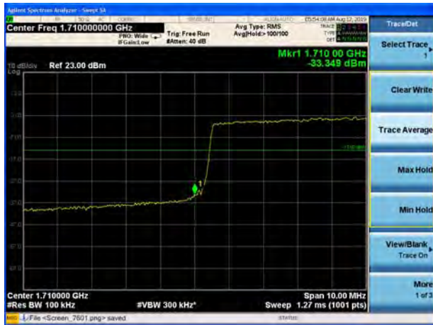
LTE Band 4 64QAM 10MHz CH-Low, 100%RB
