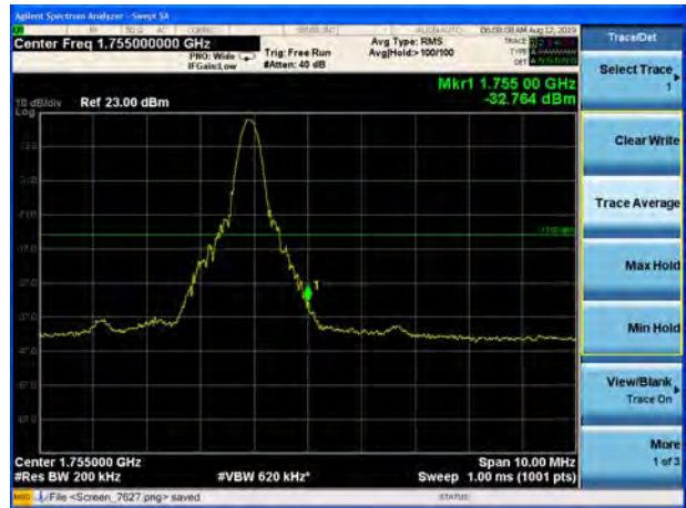
LTE Band 4 16QAM 20MHz CH-High, 1 RB
