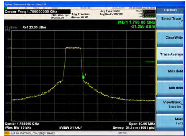
LTE Band 4 16QAM 1.4MHz CH-High, 100%RB
