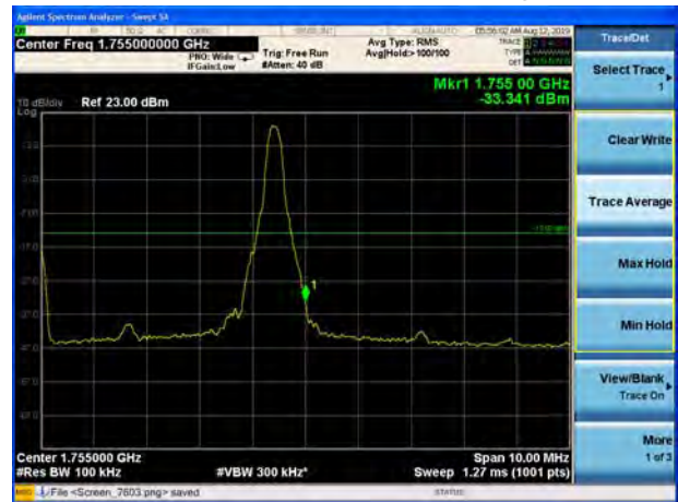
LTE Band 4 64QAM 10MHz CH-High, 100%RB
