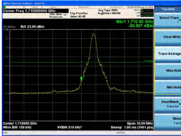
LTE Band 4 16QAM 15MHz CH-Low, 100%RB
