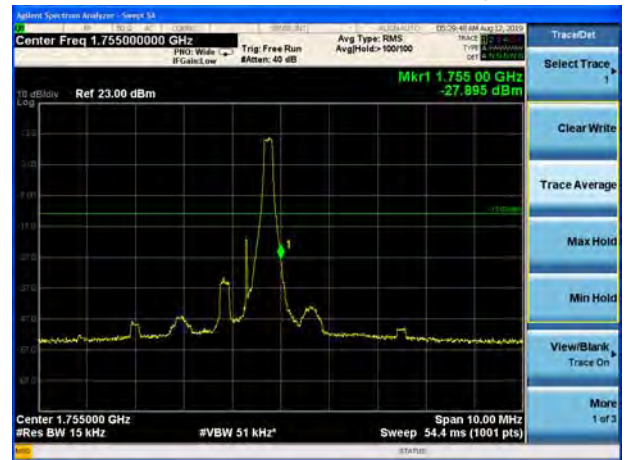
LTE Band 4 64QAM 1.4MHz CH-High, 100%RB
