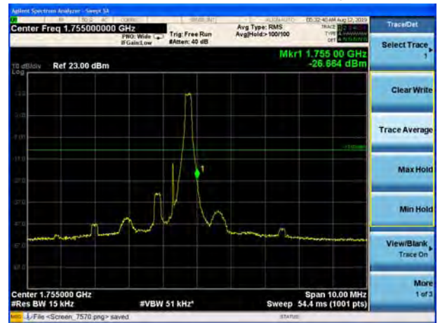
LTE Band 4 16QAM 1.4MHz CH-High, 100%RB
