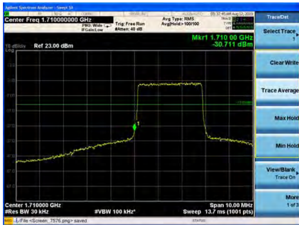
LTE Band 4 64QAM 5MHz CH-Low, 1 RB
