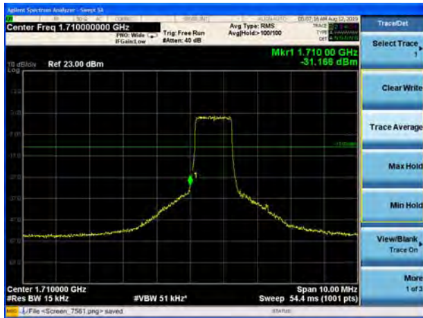
LTE Band 4 16QAM 1.4MHz CH-Low, 100%RB
