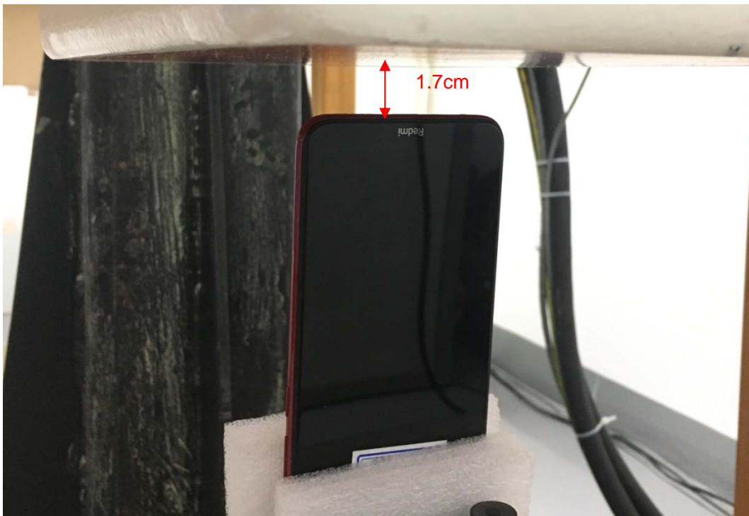
Picture 12: Bottom Side, the distance from handset to the bottom of the Phantom is 1.7cm
