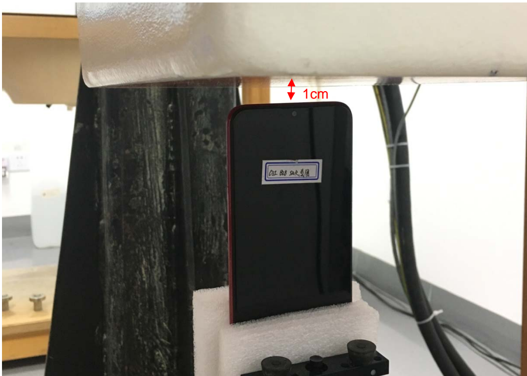
Picture 10: Top Side, the distance from handset to the bottom of the Phantom is 1.0cm
