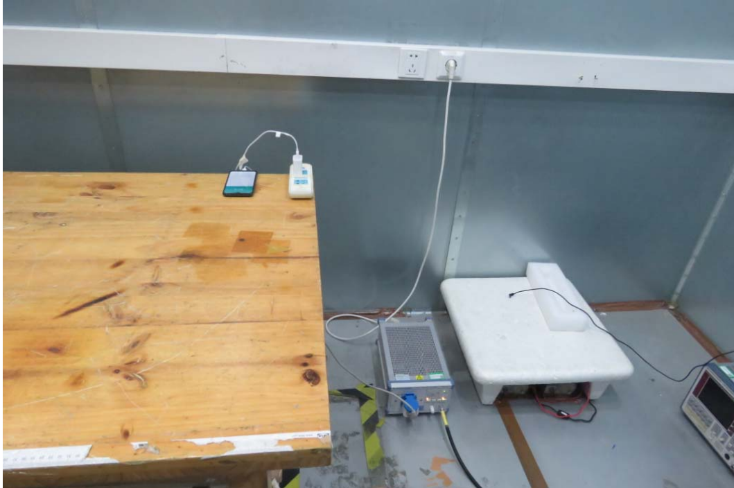
Picture 2 Conducted Emission Test Setup
