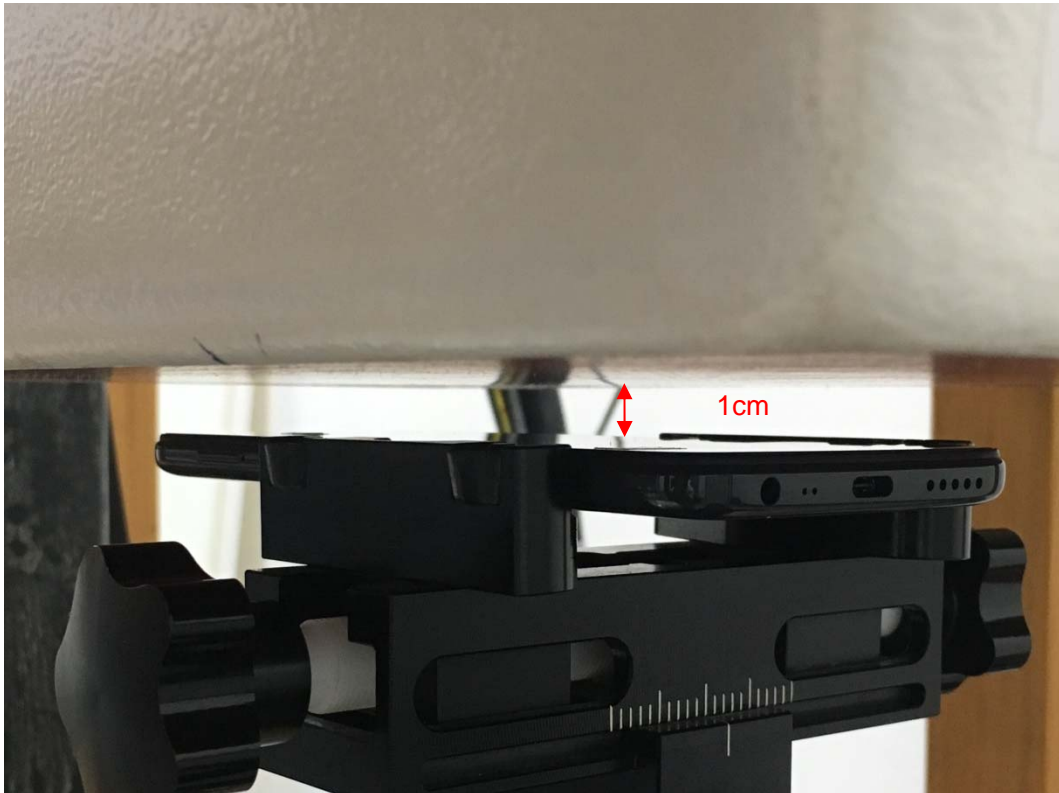
Picture 7: Front Side, the distance from handset to the bottom of the Phantom is 1.0cm
