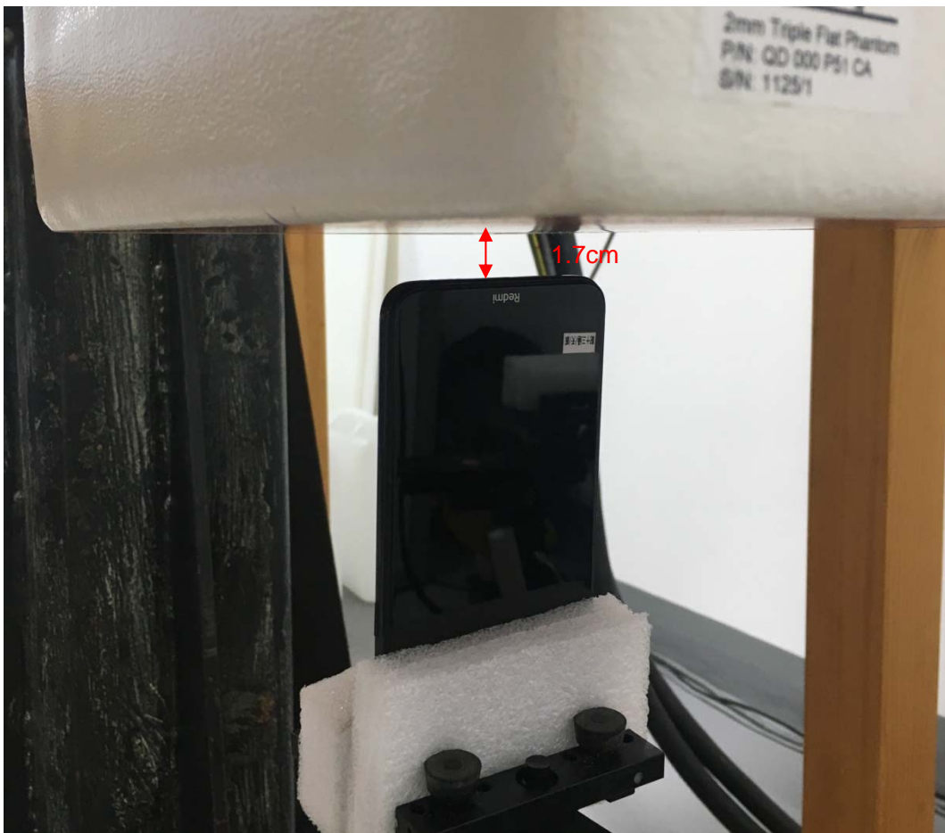
Picture 12: Bottom Side, the distance from handset to the bottom of the Phantom is 1.7cm
