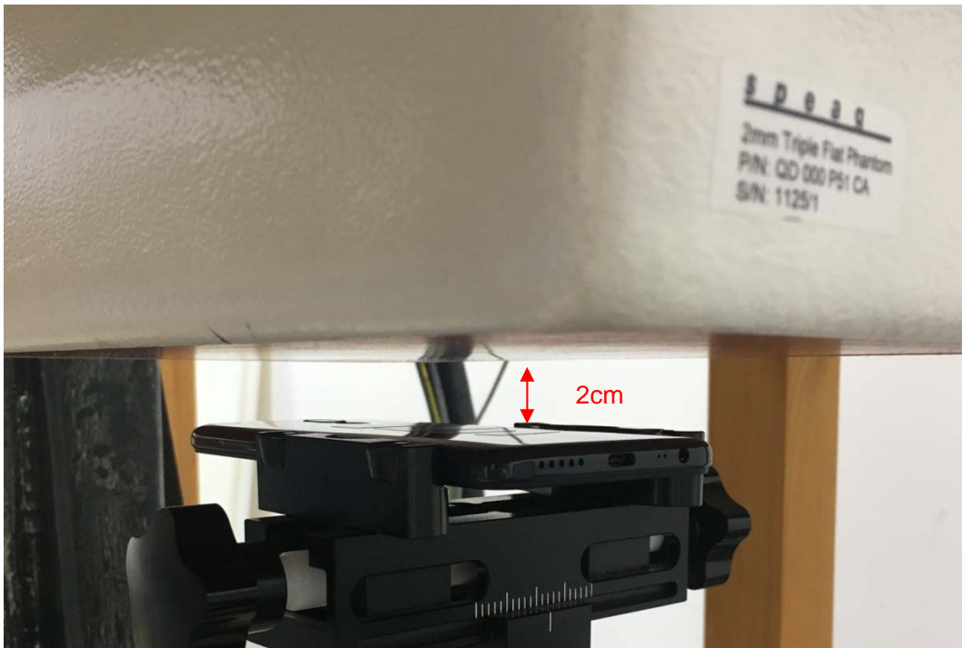
Picture 6: Back Side, the distance from handset to the bottom of the Phantom is 2.0cm
