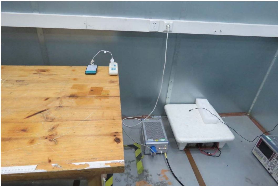
Picture 2 Conducted Emission Test Setup
