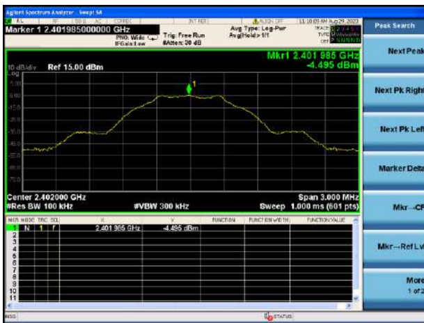
GFSK (BLE 1Mbps) LOW CHANNEL, CARRIER LEVEL
