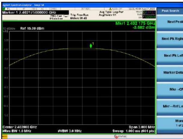
GFSK (BLE 1Mbps) LOW CHANNEL
