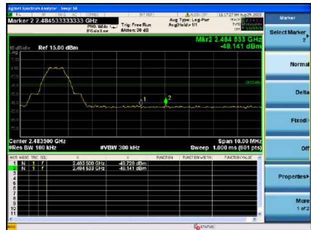
GFSK (BLE 1Mbps) HIGH CHANNEL, BAND EDGE
