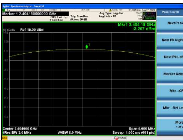
GFSK (BLE 2Mbps) LOW CHANNEL
