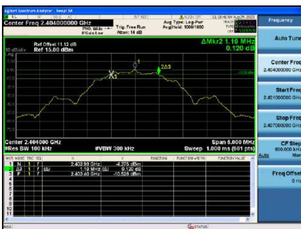
GFSK (BLE 2Mbps) LOW CHANNEL
