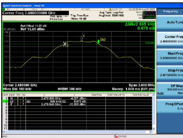
GFSK (BLE 1Mbps) HIGH CHANNEL
