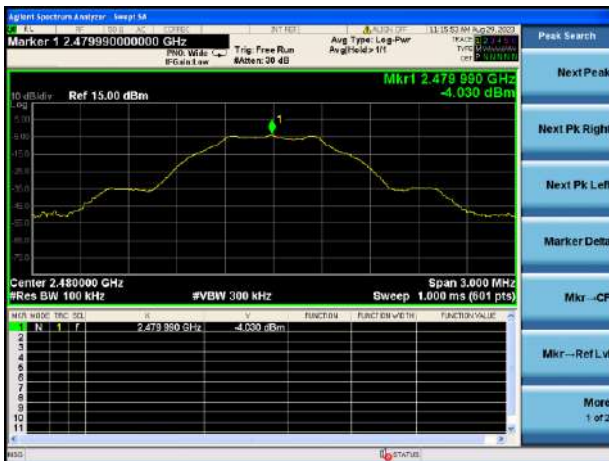
GFSK (BLE 1Mbps) HIGH CHANNEL, CARRIER LEVEL
