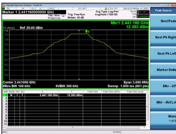
GFSK MIDDLE CHANNEL, CARRIER LEVEL
