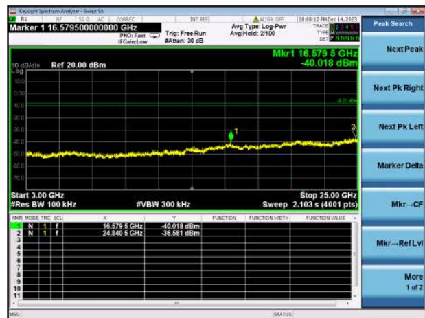
GFSK LOW CHANNEL, SPURIOUS 3 GHz ~ 25 GHz
