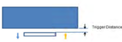
Picture : Proximity sensor triggering distances assessment (Back/front side)
