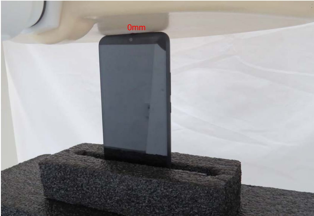
Picture 13: Top Edge, the distance from handset to the bottom of the Phantom is 0mm
