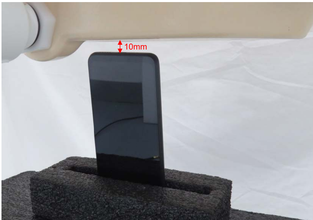
Picture 10: Bottom Edge, the distance from handset to the bottom of the Phantom is 10mm
