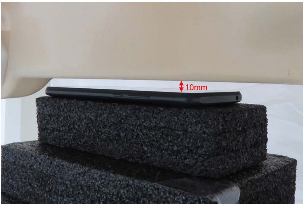
Picture 6: Front Side, the distance from handset to the bottom of the Phantom is 10mm
