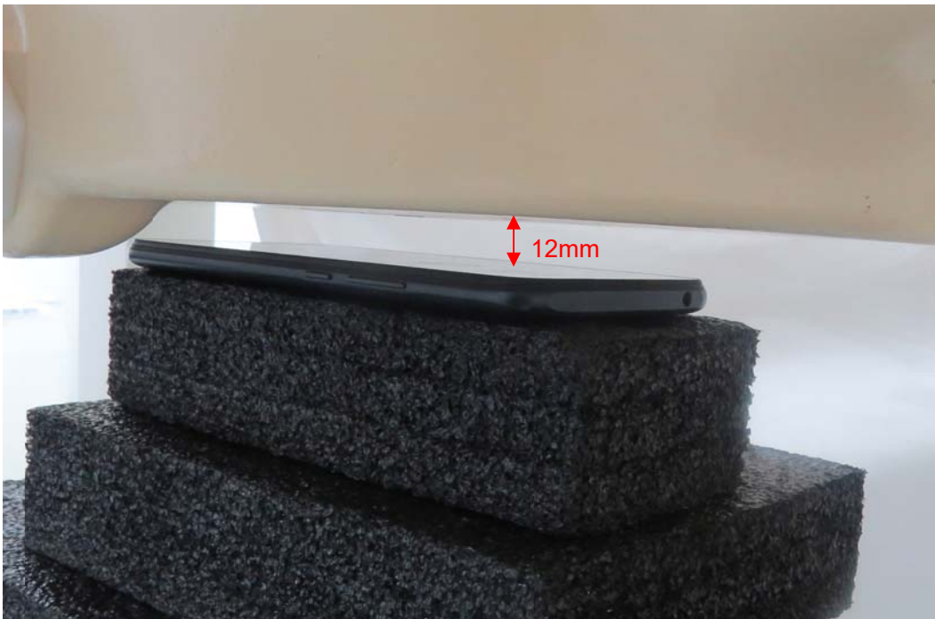
Picture 16: Front Side, the distance from handset to the bottom of the Phantom is 12mm
