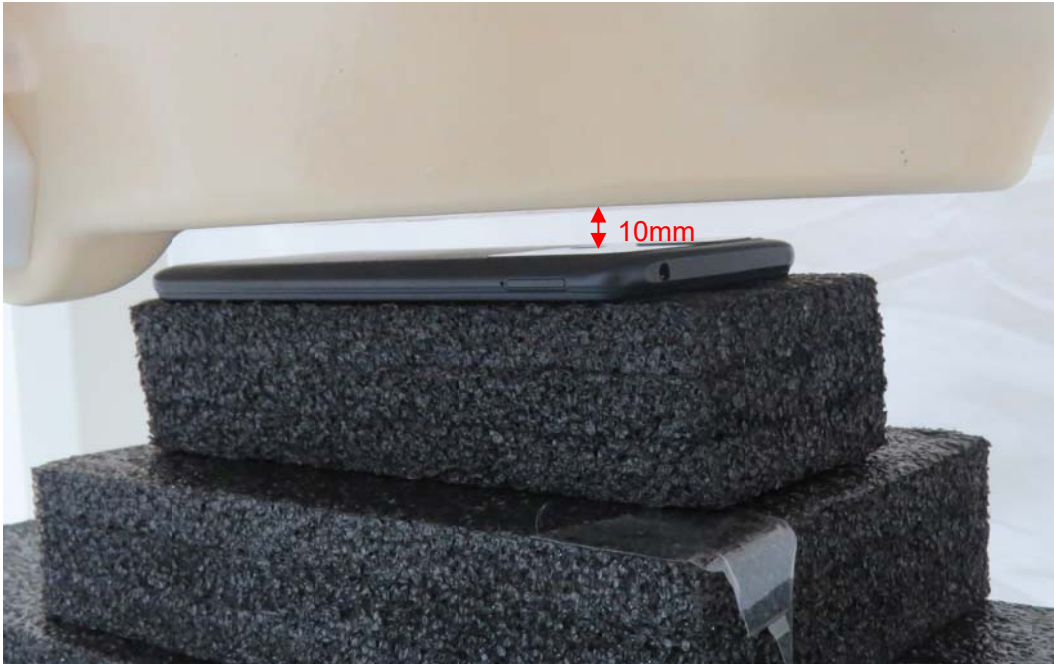
Picture 5: Back Side, the distance from handset to the bottom of the Phantom is 10mm
