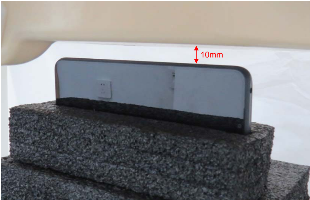
Picture 7: Left Side, the distance from handset to the bottom of the Phantom is 10mm
