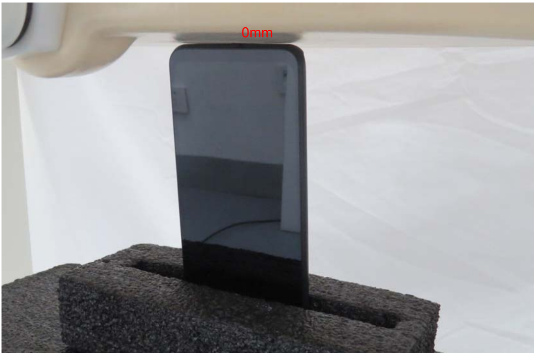
Picture 14: Bottom Edge, the distance from handset to the bottom of the Phantom is 0mm
